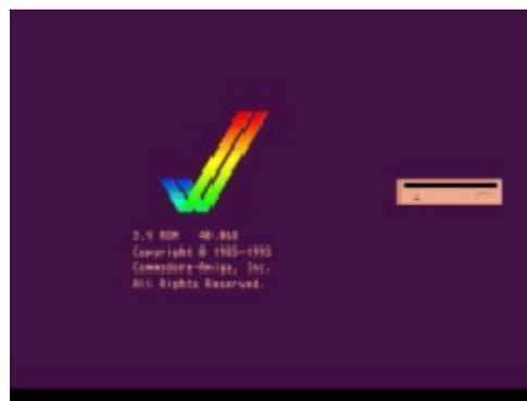
You can then insert either a Workbench disk or any other bootable disk such as a game into the floppy drive on the right-hand side of the Amiga (called DF0: - Disk Floppy Zero).
