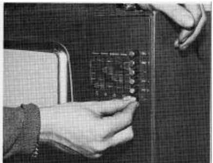
2 Next, plug the computer into the mains and turn it and the television set both on, with the volume control setting at minimum. Note that there is an on-off switch at the back of the computer. One of the lights below the keyboard should come on.
