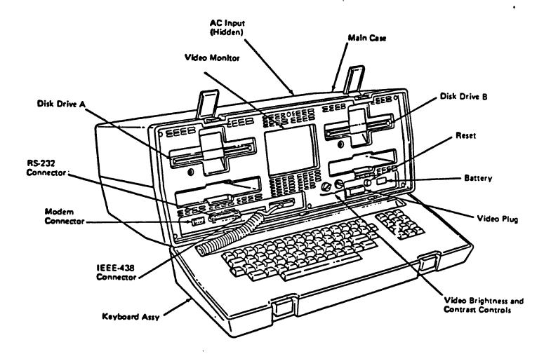
FIGURE 6-3. OCC-1A ASSEMBLED
