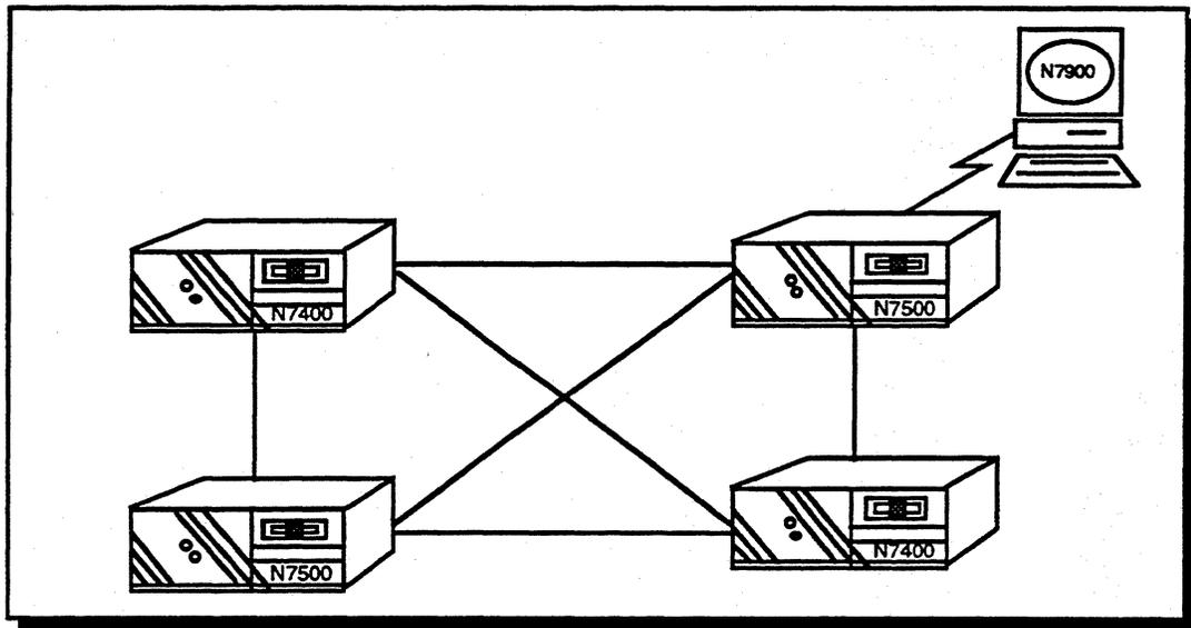
Figure 1-5 Typical Backbone Network
