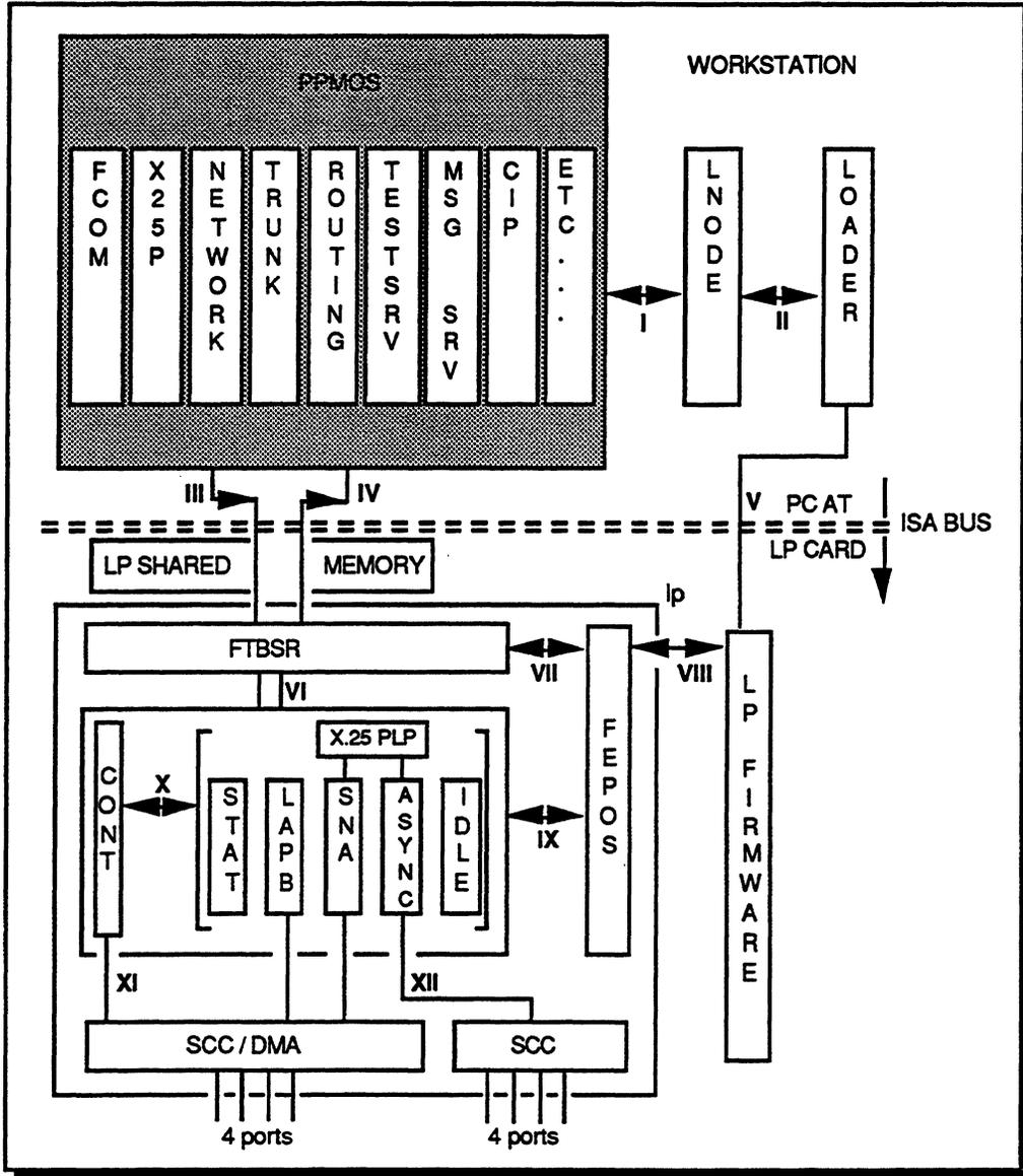
Figure D-1 Standard LP Port Interface
