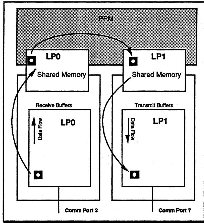
Figure 2-2 Typical LP Data Flow
