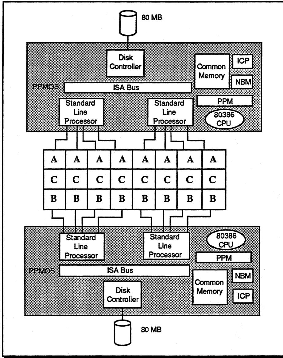
Figure 6-1 Hot Standby Switch
