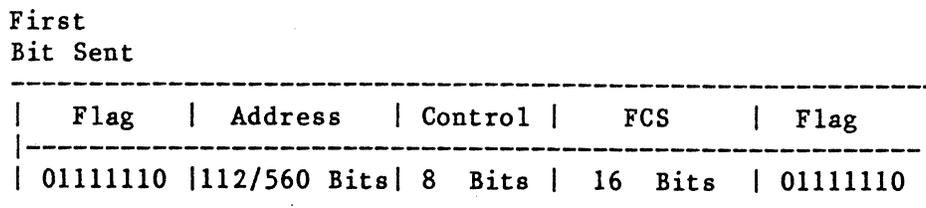
Fig. 1A -- U and S frame construction
