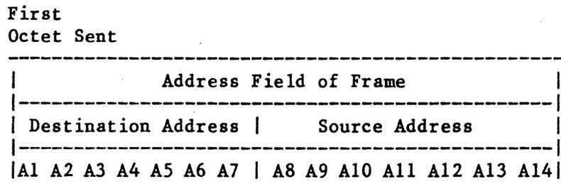
Fig. 2 -- Nonrepeater Address-Field Encoding
