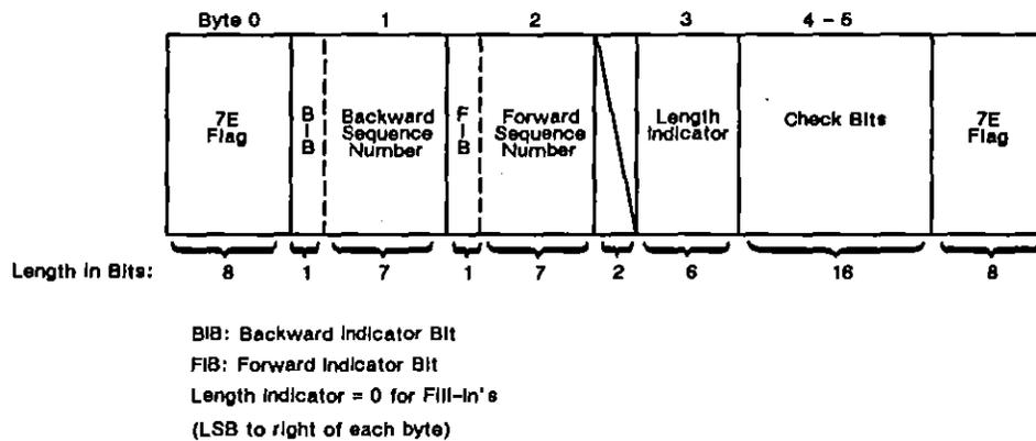
Figure 45-10 Format of Fill-in Signal Unit (FI).
