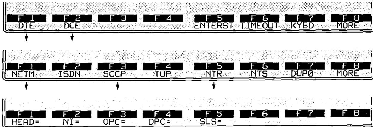
Figure 46-5 Selected MSU type determines subsequent softkey selections.
