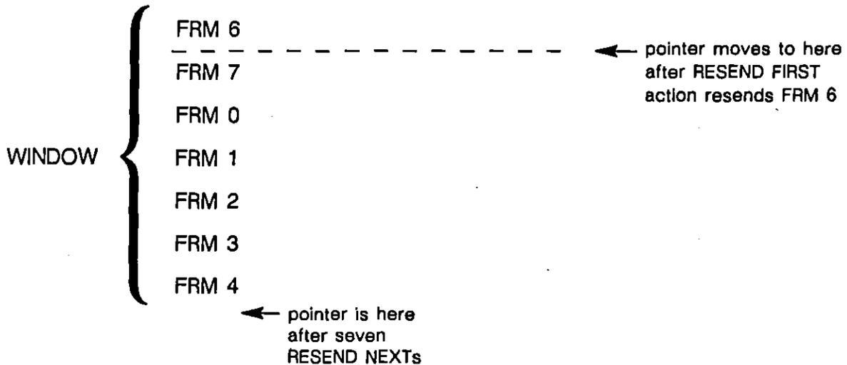
Figure 42-29 *RESEND FIRST* resets the pointer, allowing you to resend the entire window repeatedly.
