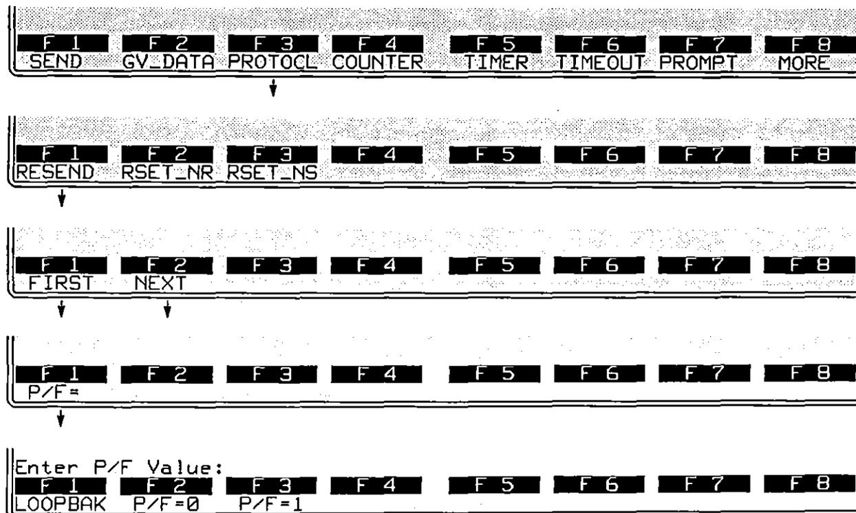
Figure 42-27 The RESEND action allows you to recover from sequence errors.
