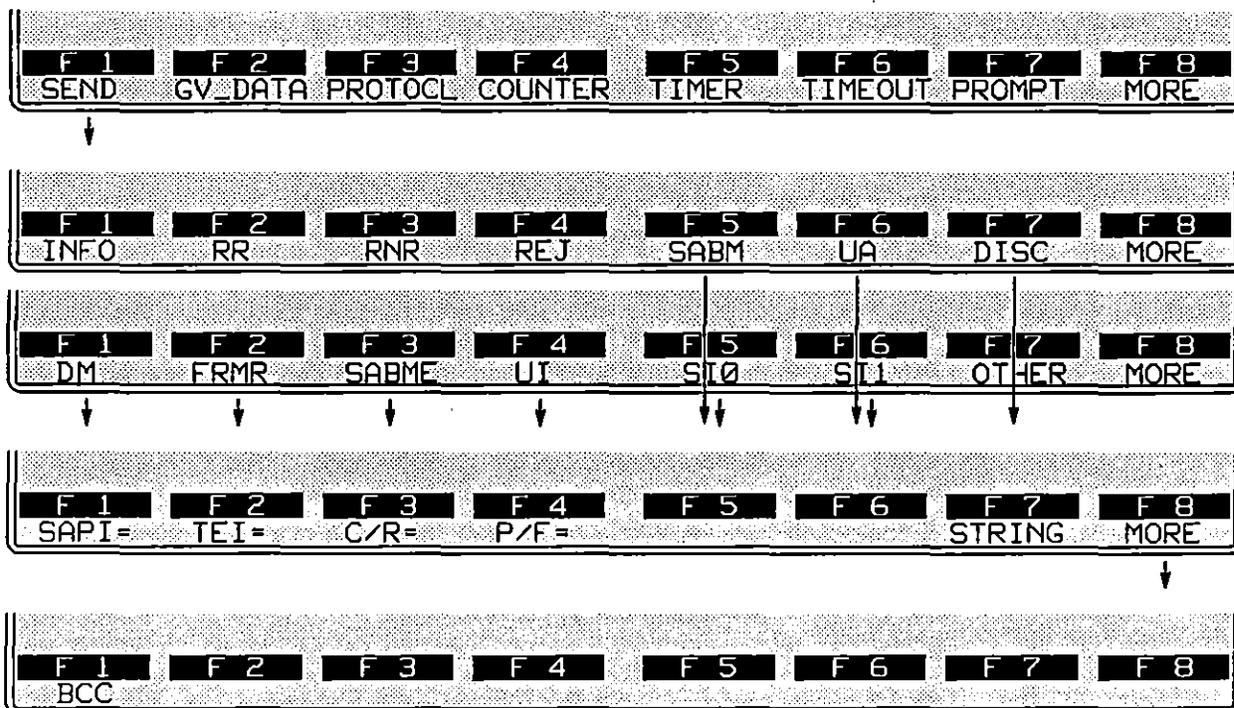
Figure 42-20 SAPI, TEI, C/R, P/F, string, and BCC options may be added to SEND unnumbered-type and SI-type actions.
