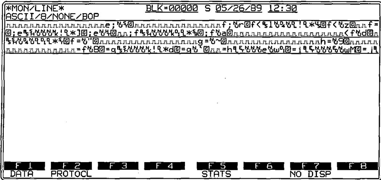
Figure 44-1 SS#7 Dual-line data display, with 7E flags suppressed and redundant LSU's and Fill-In's compressed.
