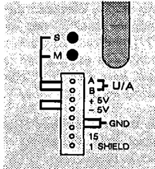
Figure 49-3 A special column of patch jacks provides UA input, positive and negative output jacks, two electrical grounds, a test point for pin 15, and case ground.
