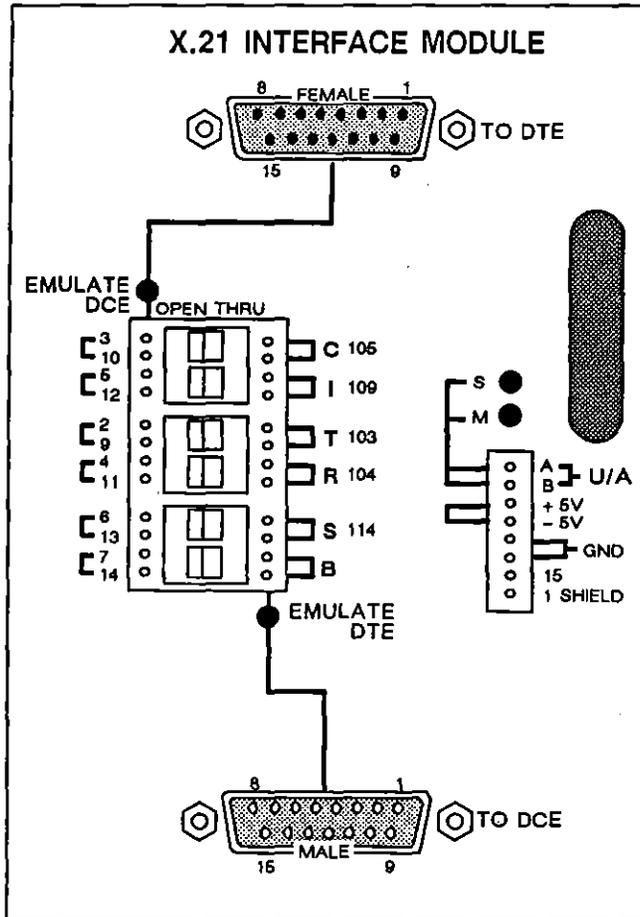
Figure 49-1 X.21 Interface Module.
