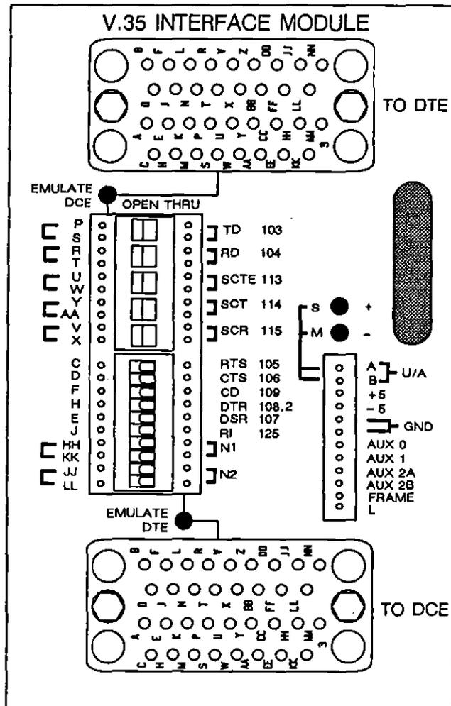
Figure 47-1 Breakout panel on V.35 Test Interface Module (TIM).
