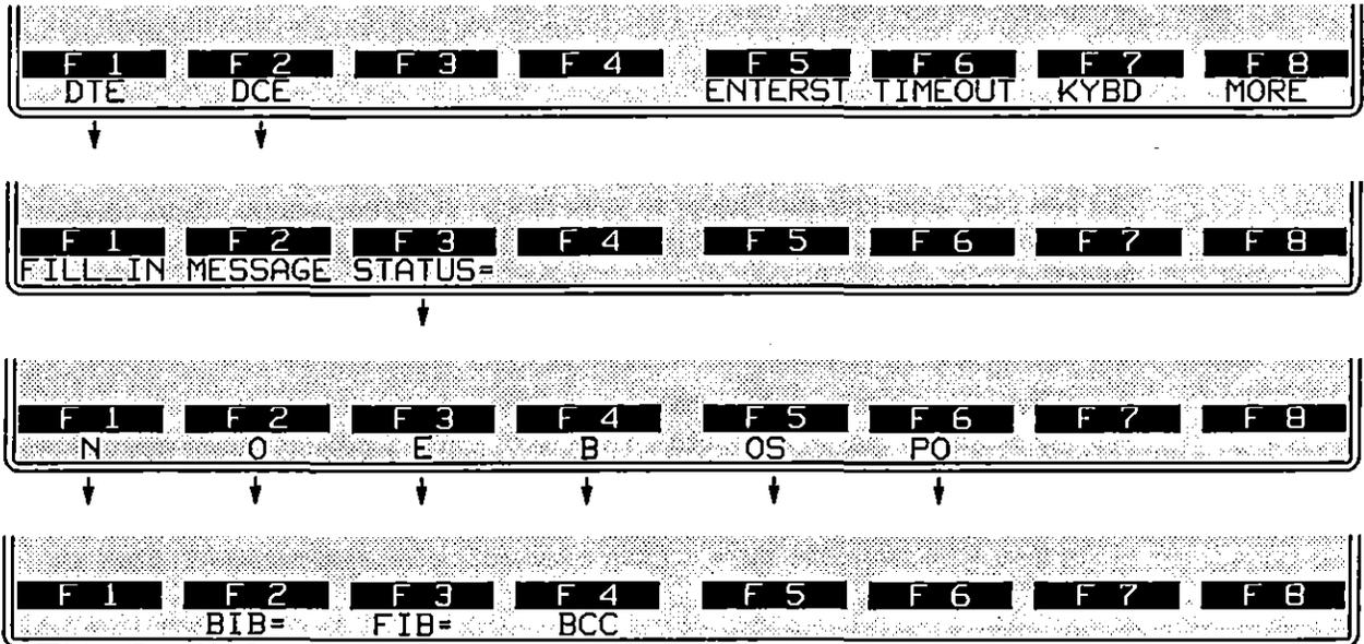
Figure 45-7 You must specify the type of Link Status Unit for a *STATUS=* spreadsheet condition. *BIB*, *FIB*, and *BCC* conditions may then be selected.
