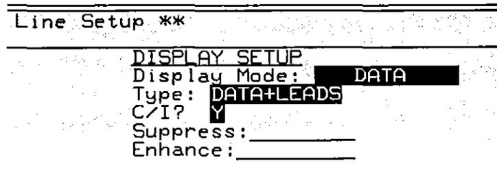
Figure 49-5 Two X.21 control leads are selectable under Type: **DATA+LEADS**.
