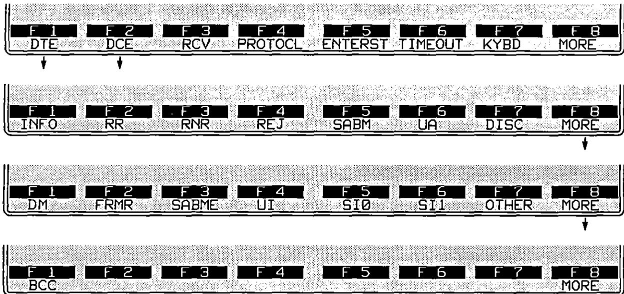
Figure 42-6 Frame type or block-check type may be specified as a complete condition for DTE or DCE.
