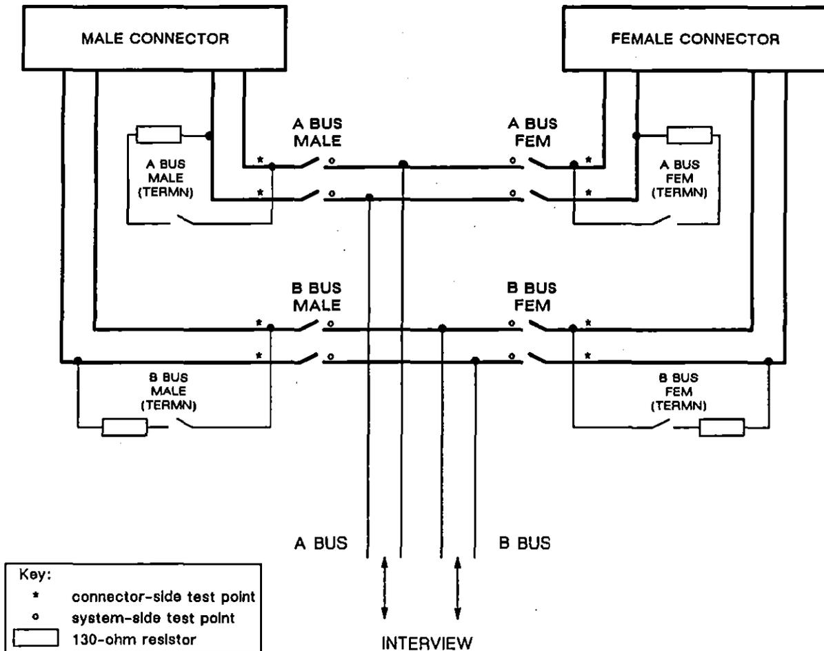
Figure 50-2 There is a pair of DIP switches for each bus. One switch controls the connection from the bus to the female connector; the other controls the connection to the male connector. When the *AUTO TERMN* switch is *OPEN*, use the four connector-termination switches (located below the *AUTO TERMN* switch on the TIM) to selectively place 130-ohm resistors across the balanced buses. To illustrate their positions, all switches in this figure are *OPEN*.
