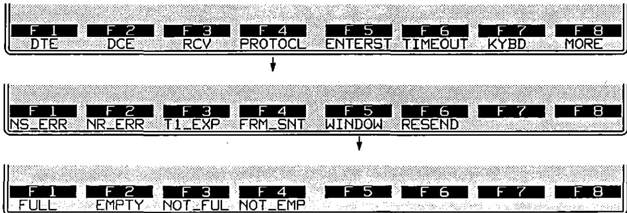
Figure 42-16 When the retransmit window fills, Layer 2 stops buffering frames for retransmission.
