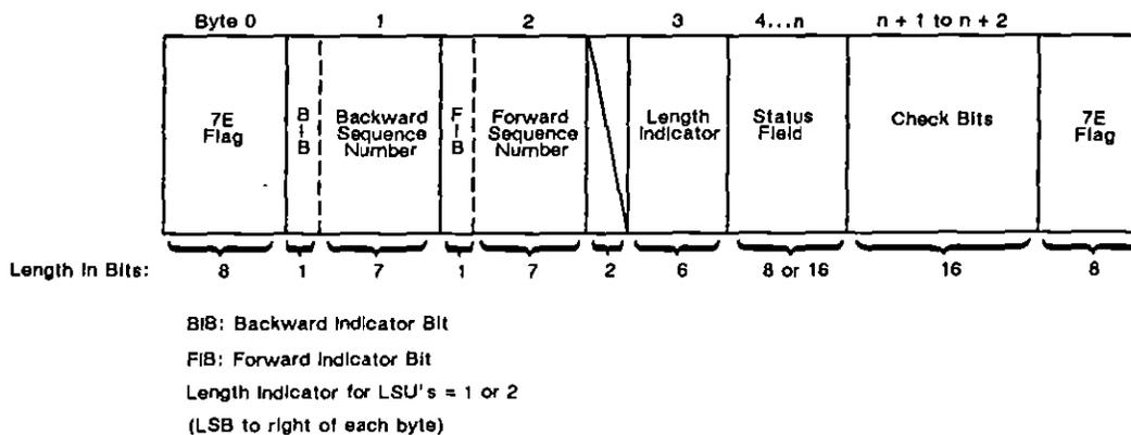
Figure 45-11 Format of Link Status Signal Unit (LSU).
