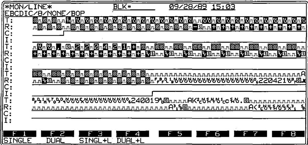
Figure 49-4 Control-lead transitions are displayable: in this example, C transitions high to indicate Call Request and I goes high to signal Ready for Data.
