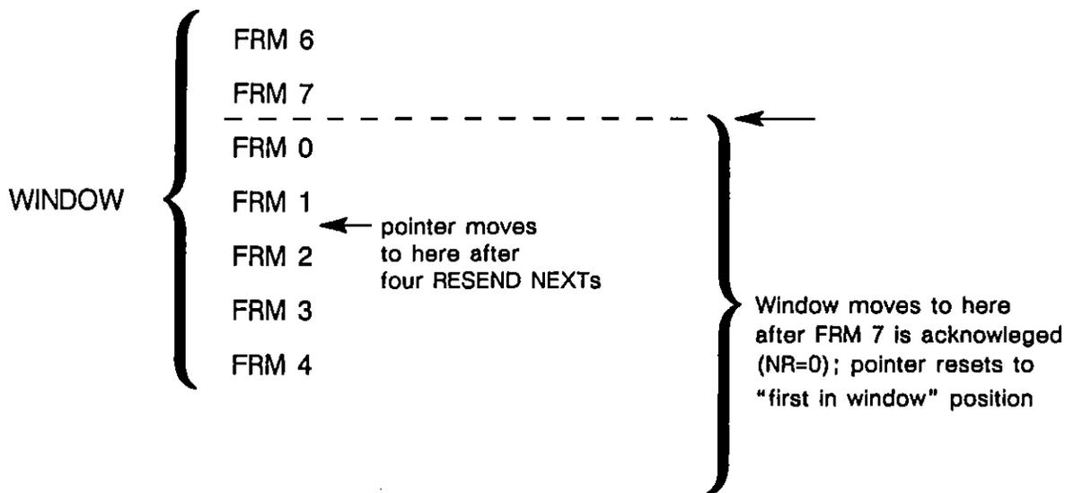
Figure 42-28 Resends cause the pointer to move, while acknowledgments move the pointer and the entire window.
