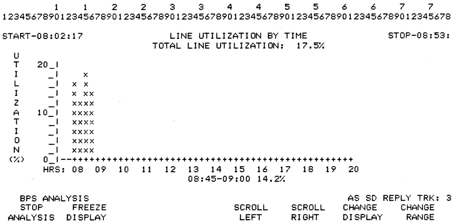
The LINE UTILIZATION BY TIME display provides analysis of total line utilization for the Host and all devices.
