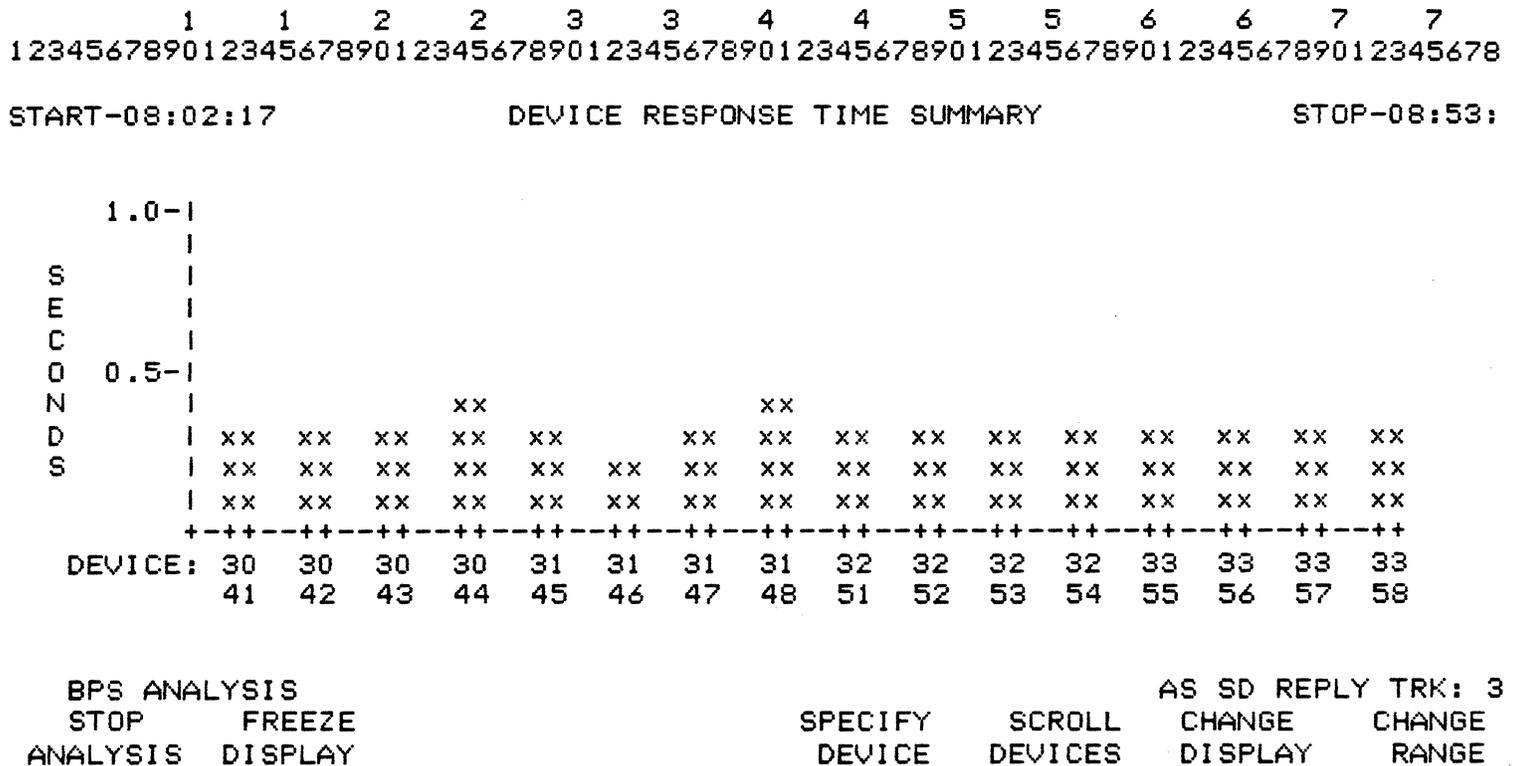
The DEVICE RESPONSE TIME SUMMARY display represents real-time or recorded / replayed data in a dynamic manner - the display is automatically updated as devices are detected and data is analyzed.
