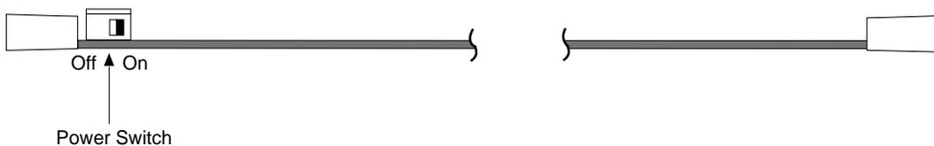
**Figure 5-9. Location of Power Switch on FRE/FRE-2 Module and SRM-F**
