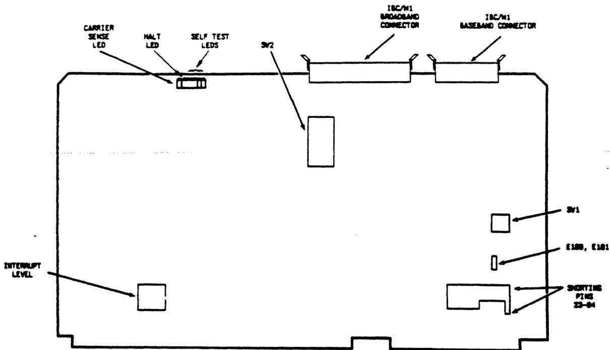
Figure 3-5 IBC/M Board (CS/1-FT)
