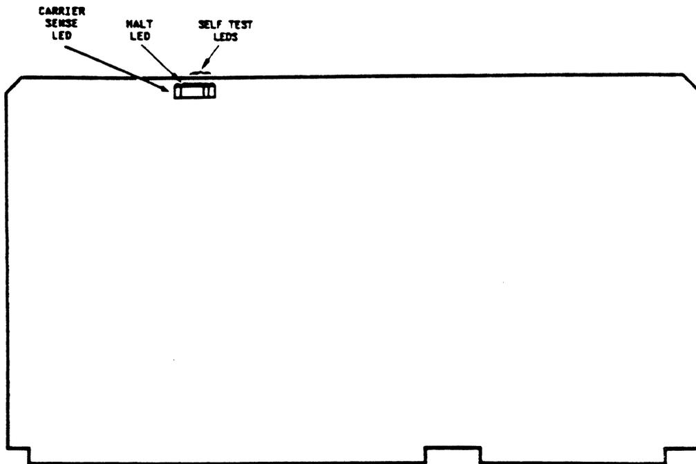
Figure 3-4 IBC/M Board
