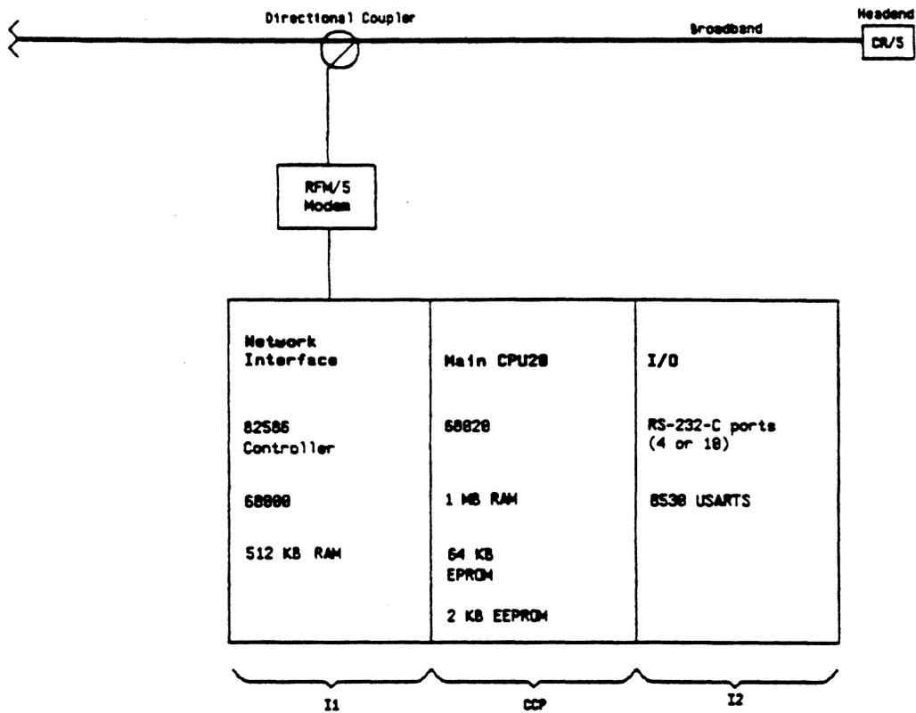
**Figure C-4 CS/1 Hardware Architecture
