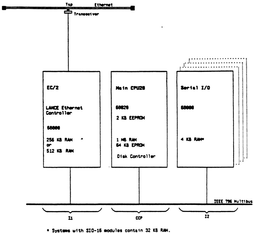
Figure C-3 Ethernet-based CS/1 (with MCPU20 Board and Asynchronous, Byte-synchronous, and Bit-synchronous Interfaces) Hardware Architecture
