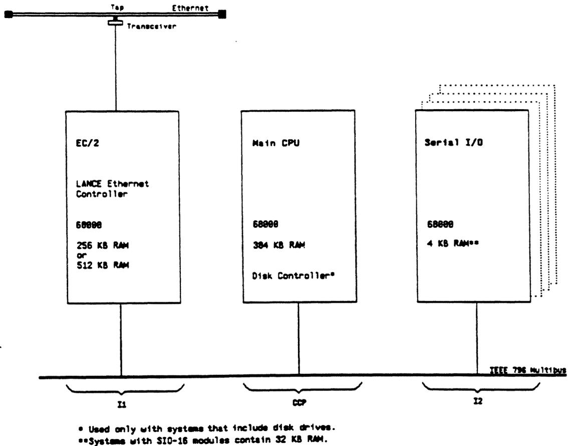
Figure C-2 CS/1 (with MCPU Board and Asynchronous, Byte-synchronous, or Bit-synchronous Interfaces) Hardware Architecture
