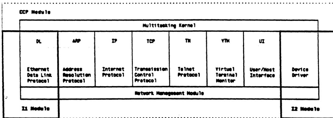
Figure C-7 CS/1 Software Architecture (with TCP/IP Protocols)
