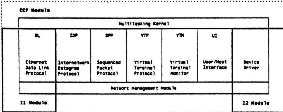
Figure C-6 CS/1 Software Architecture (with XNS Protocols and Asynchronous, Byte-synchronous, or Bit-synchronous Interfaces)
