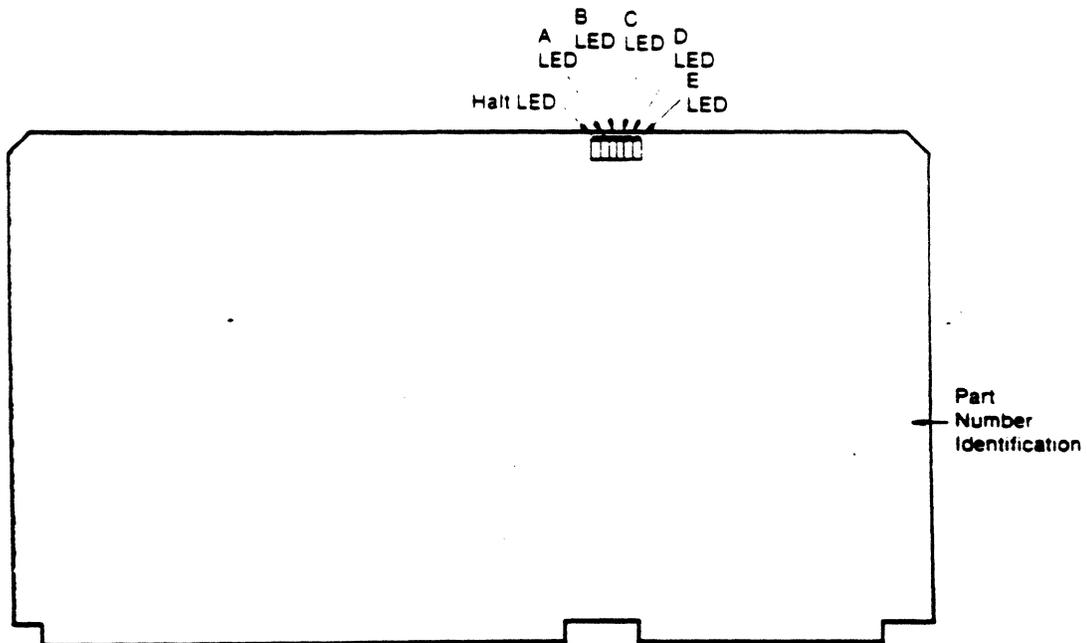
Figure 3-3 LEDs and Part Number ID Location for EC/2 Board No. 06-0041-xx
