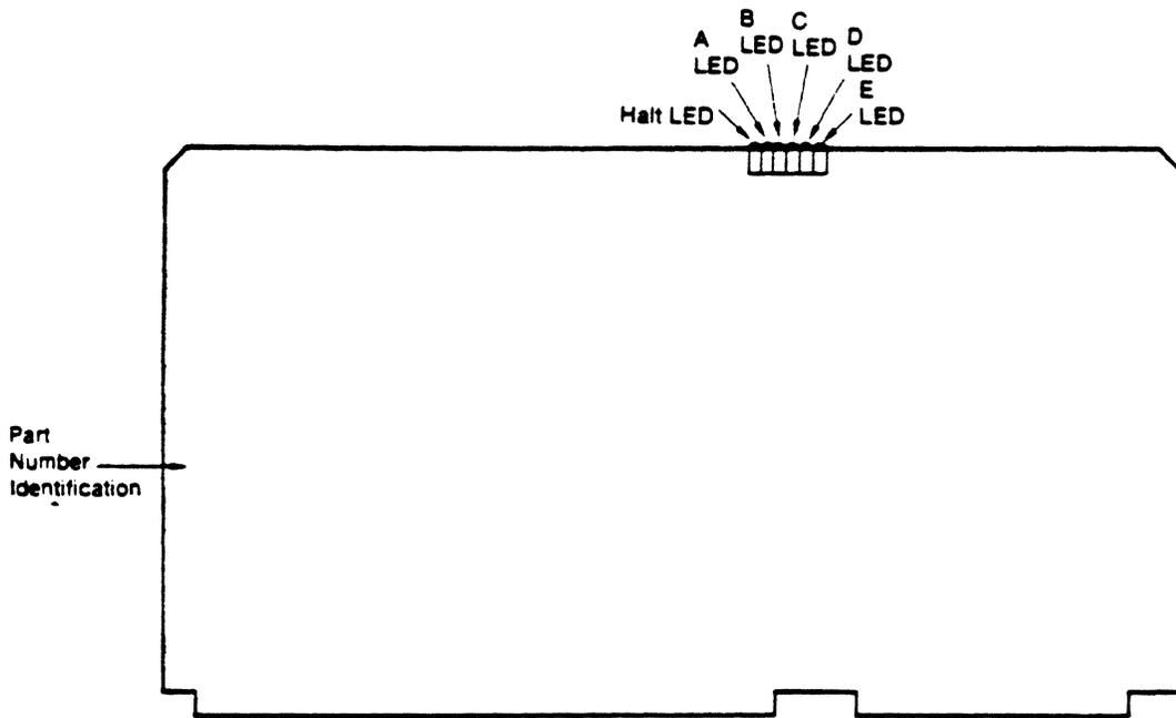
Figure 3-2 LEDs and Part Number ID Location for EC/2 Board No. 06-0021-xx
