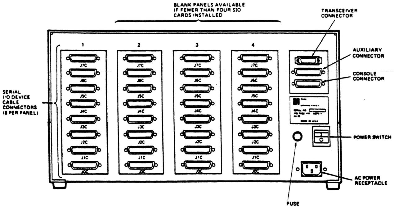
Figure 2-4 CS/1 Back Panel with SIO-A or SIO-ST Modules
