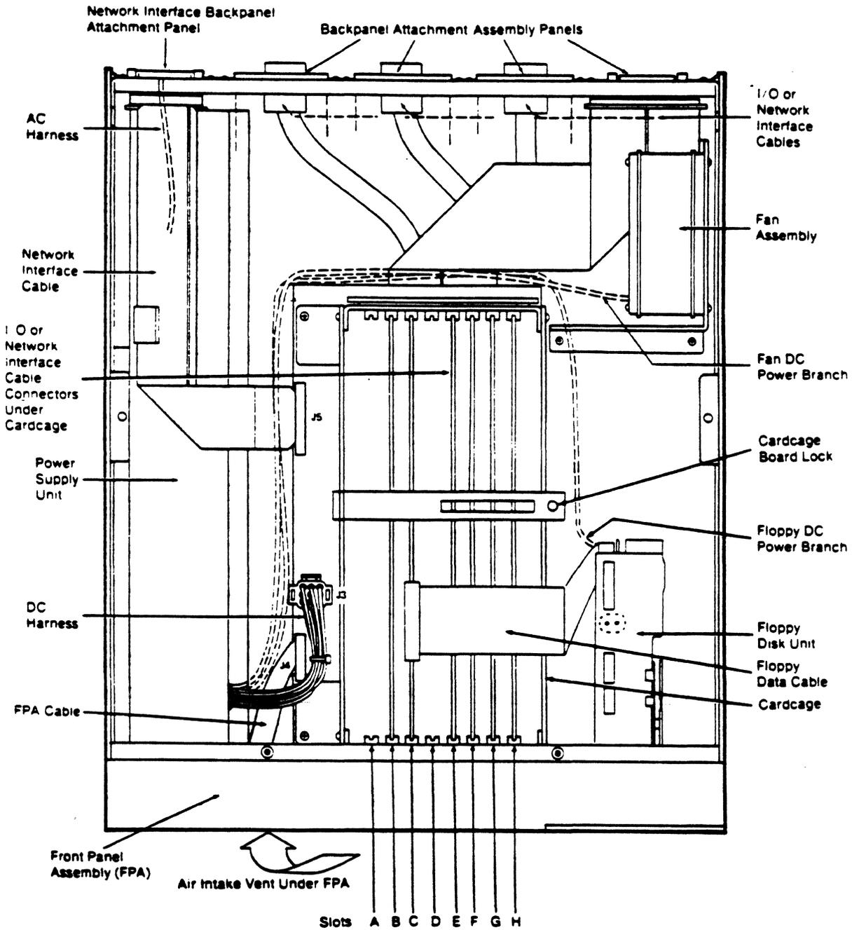
Figure 3-1 Placement of Major Hardware Components
