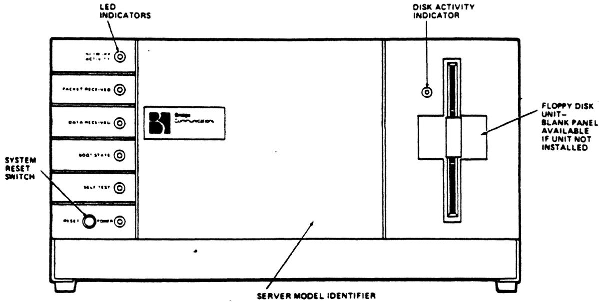
Figure 2-3 CS/1 Front Panel
