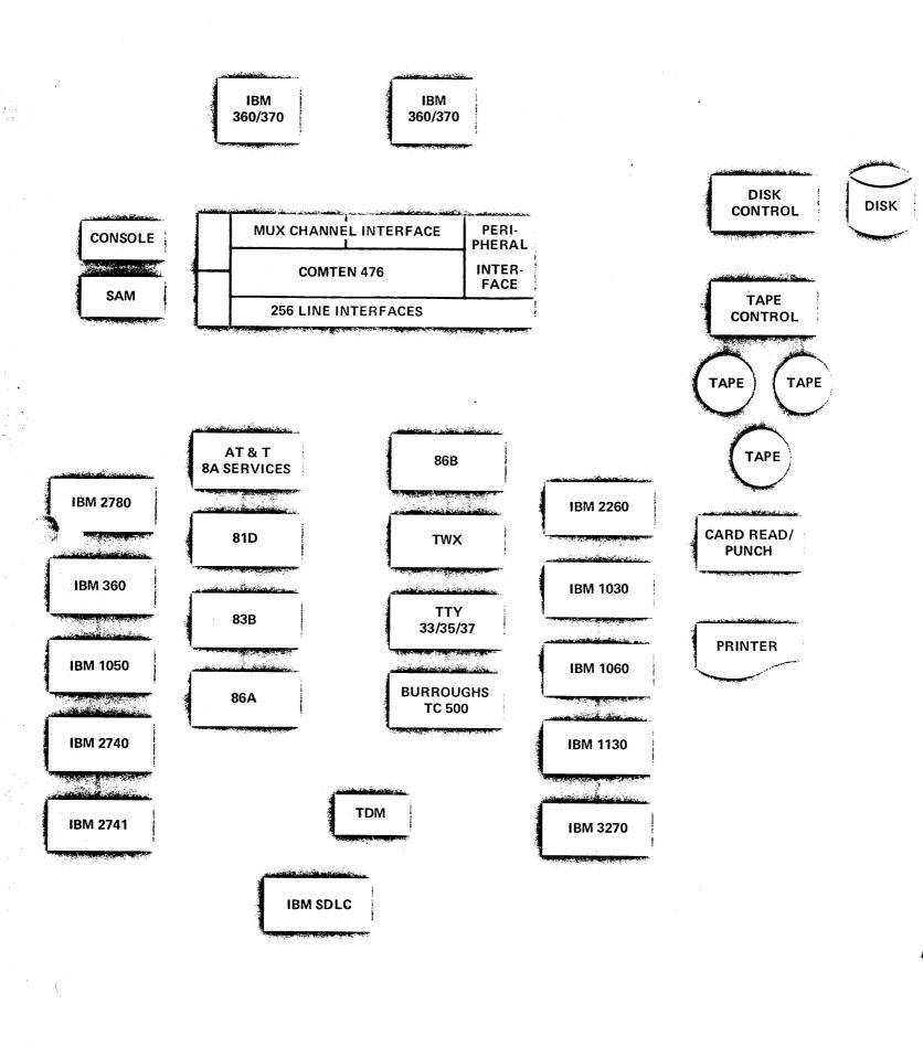
Orderly flow of work through the COMTEN communication system is controlled and maintained by the COMTEN Supervisor. This versatile executive system assures maximum system efficiency by overlapping compute and I/O tasks of several programs.
