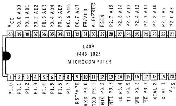
The clear to send (CTS) and data terminal ready (DTR) control signals (handshaking) on the computer port (DTE) are taken directly from the microcomputer and passed to the line drivers. On the auxiliary port the clear to send (CTS), data terminal ready (DTR), data set ready (DSR), and the received line signal detect (RLSD) signals are all tied together.
