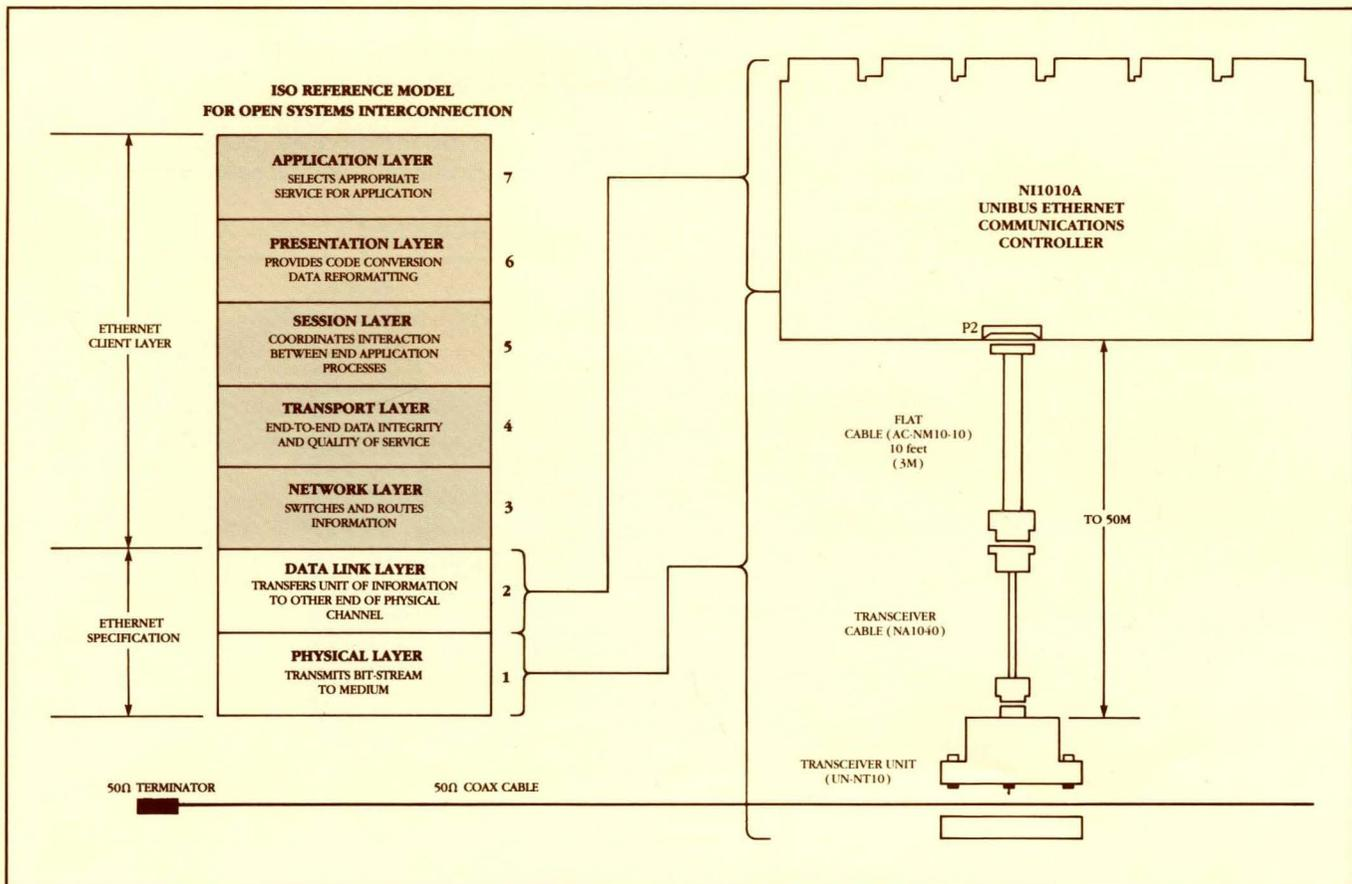
Figure 1. Ethernet Architecture and Implementation
