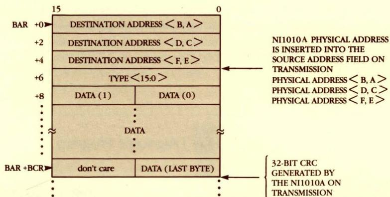
Figure 7. Transmit Data Organization in Unibus Memory
