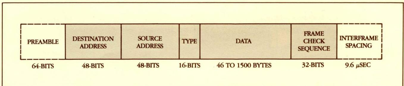
Figure 2. Ethernet Frame Format
