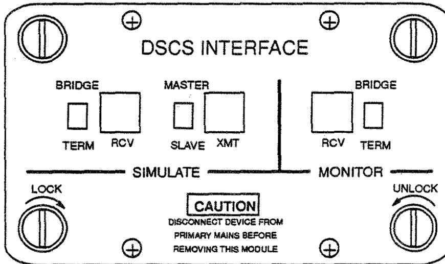
The receiver (A) and transmitter (B) connections to the DSCS interface are industry-standard 3-conductor bantam jacks. The receivers operate with standard DSCS/DDS signals per AT&T Pub 62310 and Bellcore TA-TSY-000083. The maximum distance from OCU and DSU is 1000 feet.
