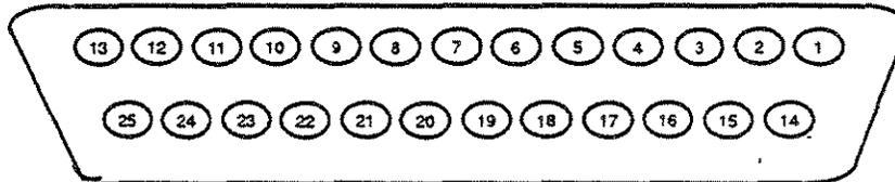
All signals are standard RS-232 voltage levels. The connector is physically and electrically a DCE type connector.
