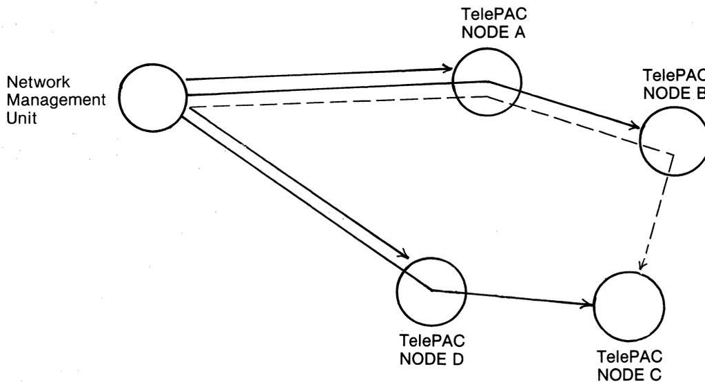
Main X.25 Call to MNGE ports and alternative to NODE C if NODE D down
