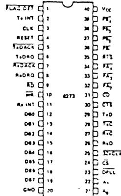
Figure 2. Pin Configuration
