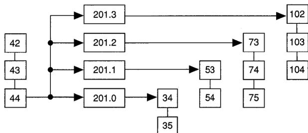
Any of the 13 available commands can be enhanced with multiway branching. For example, location 44 in Figure 10 can be a CALL to a subroutine, and address 201 can contain the starting instruction for 4 unique subroutines. The routine that is actually executed depends on the user-defined condition of the inputs. The following ASM code can be used to implement this example:
