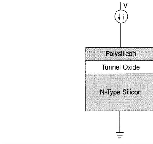
The I-V relationships for programmed and erased EEPROM cells are similar to those of EPROM cells (see Figure 6). Unlike the EPROM cell, however, the threshold voltage of a discharged EEPROM cell is negative (less than 0 V) because electrons are removed from the floating gate. Electron removal gives the floating gate a net positive charge.
