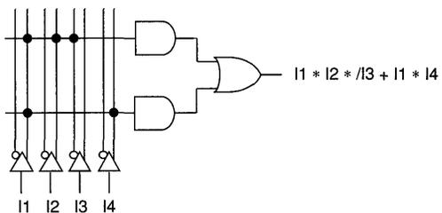
Outputs of the product terms are tied to the inputs of an OR gate to compute the sum. Since all combinatorial logic can be reduced to a sum-of-products expression, the generic AND-OR array of Circuit C can produce any Boolean function. (The actual product terms in Altera devices are much wider than the 8 inputs shown.)
