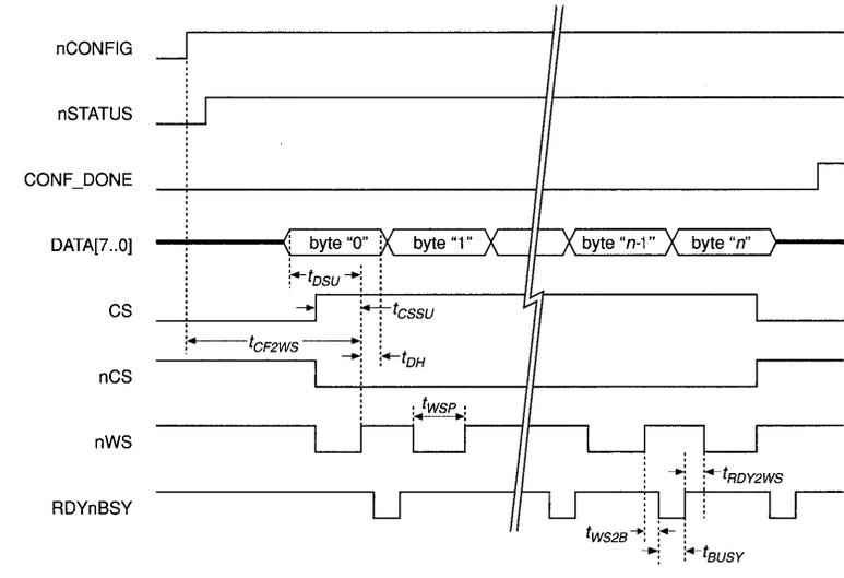
The CPU must poll the RDYNBSY signal to establish when the FLEX 8000 device is ready to receive more data. RDYNBSY falls immediately after the rising edge of the DCLK signal that latches data, indicating that the device is busy. While the FLEX 8000 device processes the data byte, RDYNBSY remains low. On the eighth falling edge of DCLK, RDYNBSY returns to V<sub>CC</sub>, indicating that another byte of data can be latched. Table 6 shows the timing parameters associated with PPA configuration.
