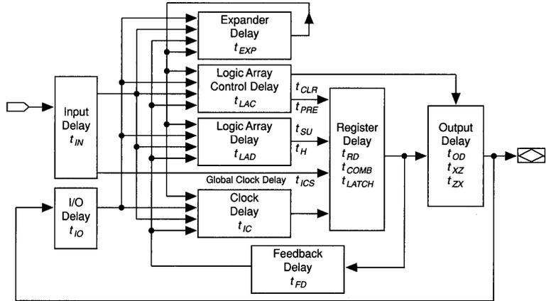
Figure 3 shows the timing model for the multi-LAB MAX 5000 EPLDs: the EPM5064, EPM5128, EPM5128A, EPM5130, EPM5192, and EPM5192A EPLDs. In multi-LAB devices, the Programmable Interconnect Array (PIA) routes signals between different LABs. All I/O inputs come into the logic array through the PIA. Signals routed through the PIA incur an additional delay.
