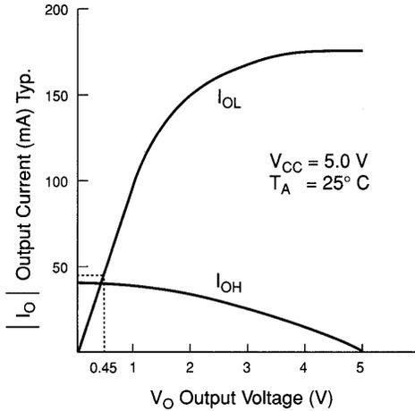
**Output Drive Characteristics of EP1810-35 & EP1810-45 EPLDs**
