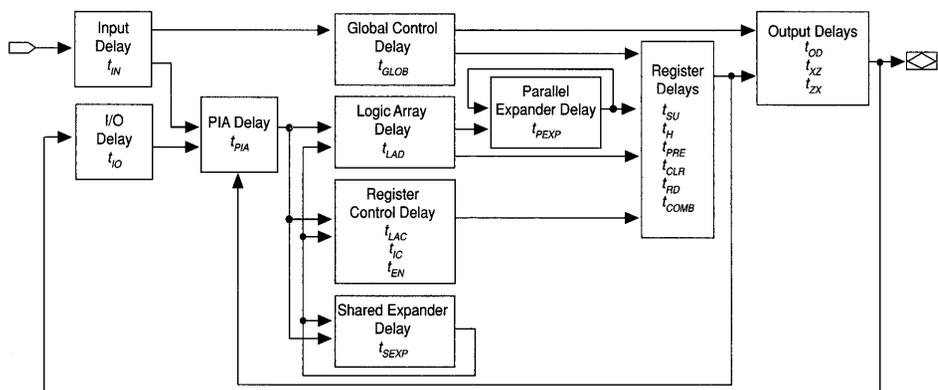
Timing information can be derived from the timing model and parameters for a particular EPLD. External timing parameters can be calculated from the sum of internal parameters and represent pin-to-pin timing delays. Figure 8 shows the internal timing relationship for internal and external delay parameters. See *Application Brief 100 (Understanding EPLD Timing)* in this data book for more information.
