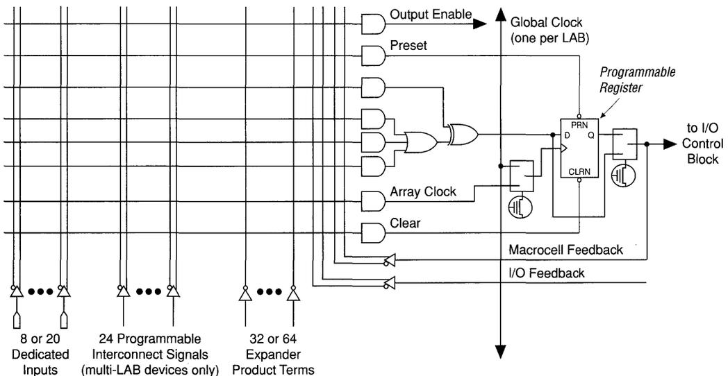
The output of the XOR gate feeds the programmable register or bypasses it for combinatorial operation.
