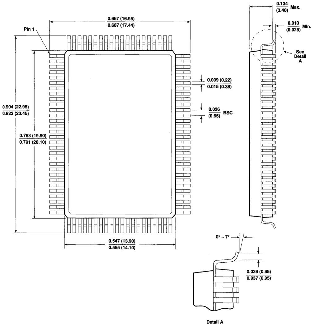
**100-Pin Thin Plastic Quad Flat Pack (TQFP)**
