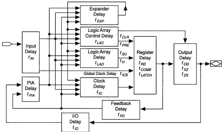
The timing model for the EPS464 EPLD is shown in Figure 4.
