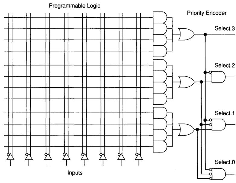
The EPS448 EPLD is designed so that the number of available product terms is always sufficient for a design. Prioritization provides an effective product-term count of more than 12 per location. A tradeoff between the number of product terms and the number of possible branches can be made simply by placing identical state information in 2 locations, as shown in Figure 6.
