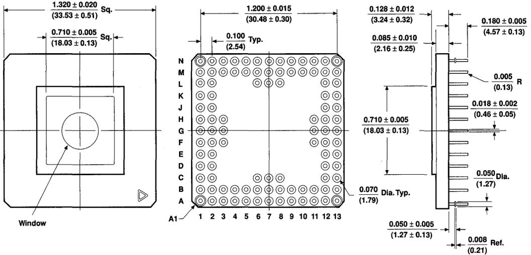
**100-Pin Large Outline Ceramic Pin-Grid Array (PGA)**
