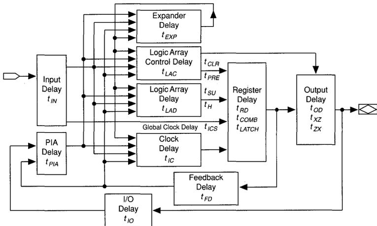
Timing information can be derived from the timing model and parameters for a particular EPLD. External timing parameters are calculated with the sum of internal parameters and represent pin-to-pin timing delays. Figure 6 shows the internal timing relationship for internal and external delay parameters. For more information on EPLD timing, refer to *Application Brief 100 (Understanding EPLD Timing)* in this data book.
