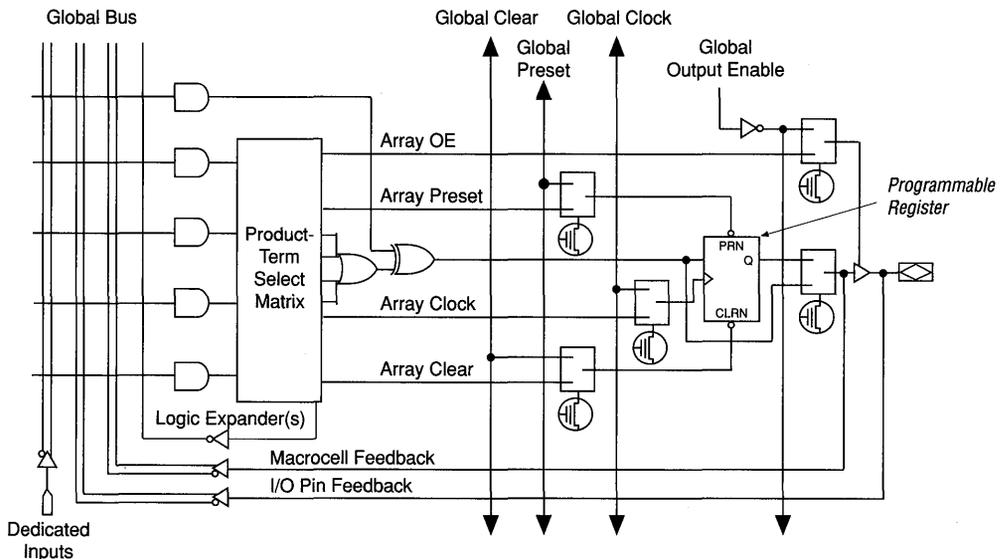
Combinatorial logic is implemented in the product-term array, which consists of five product terms. Four product terms feed the product-term select matrix; the fifth feeds one input of an XOR gate, making it possible to implement active-high or active-low logic. The XOR gate is also used to build complex arithmetic logic functions and to perform De Morgan's
