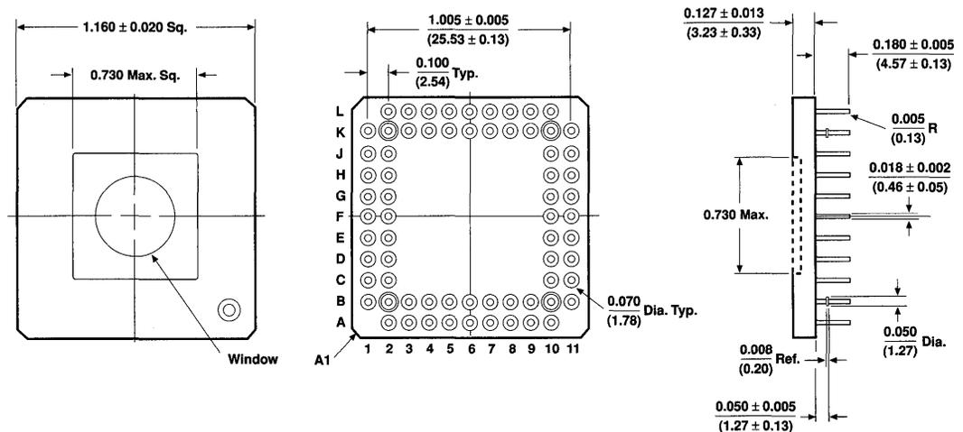
**84-Pin Ceramic J-Lead Chip Carrier (JLCC)**
