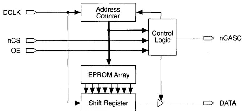
The control signals for Configuration EPROMs (DCLK,  $nCS$ , OE) interface directly to the FLEX 8000 device control signals. A FLEX 8000 device can control the entire configuration process by retrieving the configuration data from the Configuration EPROM without an external intelligent controller. Configuration usually occurs automatically at system power-up.
