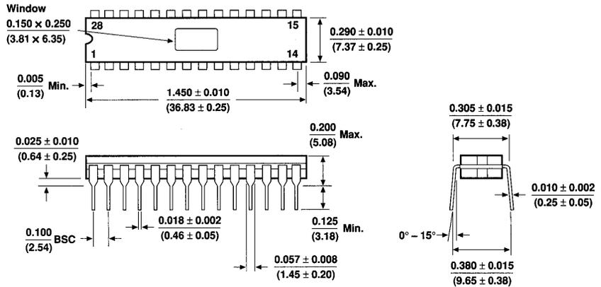
**28-Pin Plastic Dual In-Line Package (PDIP)**
