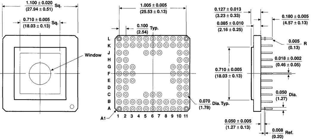
**84-Pin Large Outline Ceramic Pin-Grid Array (PGA)**
