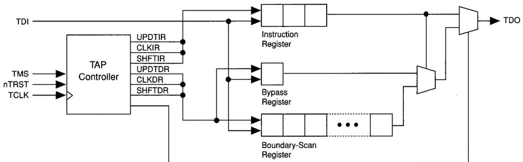
Table 5 describes the SAMPLE, EXTEST, and BYPASS test instruction modes. For additional information on JTAG boundary-scan testing for FLEX 8000 devices, contact Altera Applications at (800) 800-EPLD.
