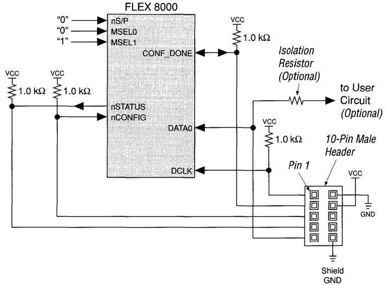
A 10-pin female plug on one end of the FLEX Download Cable is connected to the 10-pin male header on the circuit board; the other end of the FLEX Download Cable is connected to a Configuration EPROM programming adapter. See Figure 15. Timing for PS configuration is identical to the timing for bit-wide PS configuration shown later in this application note.
