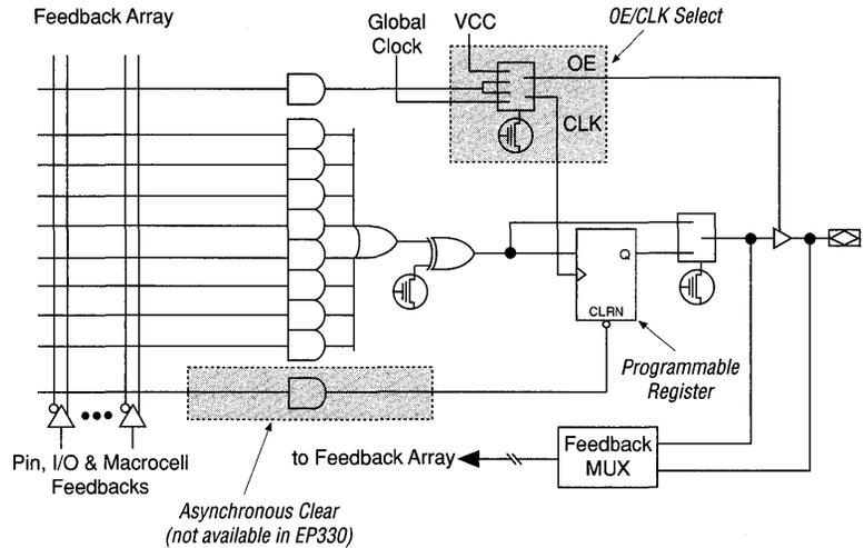
The eight product terms of the programmable-AND array feed the 8-input OR gate, which then feeds one input to an XOR gate. The other input to the XOR gate is connected to a programmable bit that allows the array output to be inverted. Altera's MAX+PLUS II software uses the XOR gate to implement active-high or active-low logic, or uses De Morgan's inversion to reduce the number of product terms to implement a function.
