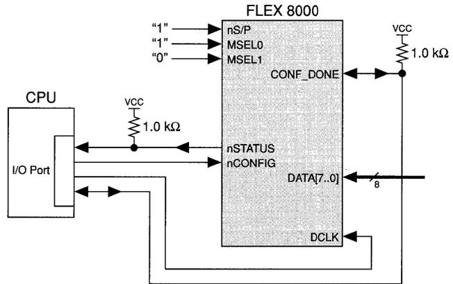
Figure 9 shows the timing for the PPS configuration scheme. The CPU generates Clock cycles and data; eight DCLK cycles are required to latch and serialize each 8-bit data word. A new data word must be present at the DATA[7..0] inputs upon every eighth DCLK cycle.
