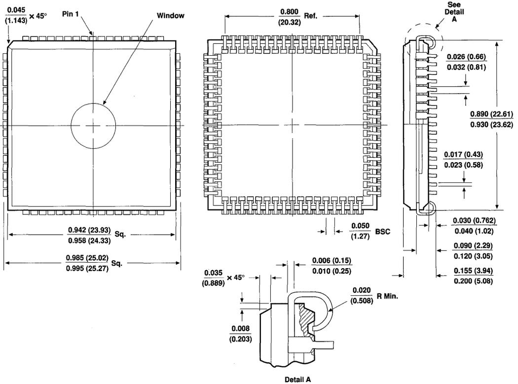
**68-Pin Plastic J-Lead Chip Carrier (PLCC)**
