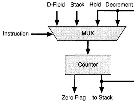
The CREG is loaded or decremented on the leading edge of the Clock. It stops decrementing once it reaches zero, thereby preventing roll-over. A zero flag indicates when the counter has reached zero. This flag is used with the `LOOPNZ` command to control program flow. (See “Instruction Set” later in this data sheet.) Single-instruction delay loops are easily constructed, and nested loops or delays of arbitrary length can be generated in combination with the stack.
