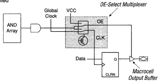
In Mode 1, the output is permanently enabled and the register is clocked by the product term, which allows gated clocks to be generated. (Not available in EP330 EPLDs.)
