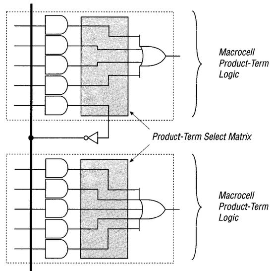
Parallel expanders are unused product terms from macrocells that can be allocated to a neighboring macrocell to implement fast, complex logic functions. With parallel expanders, up to 20 product terms can directly feed the macrocell OR logic—5 product terms provided by the macrocell and 15 parallel expanders provided by neighboring macrocells in the LAB.
