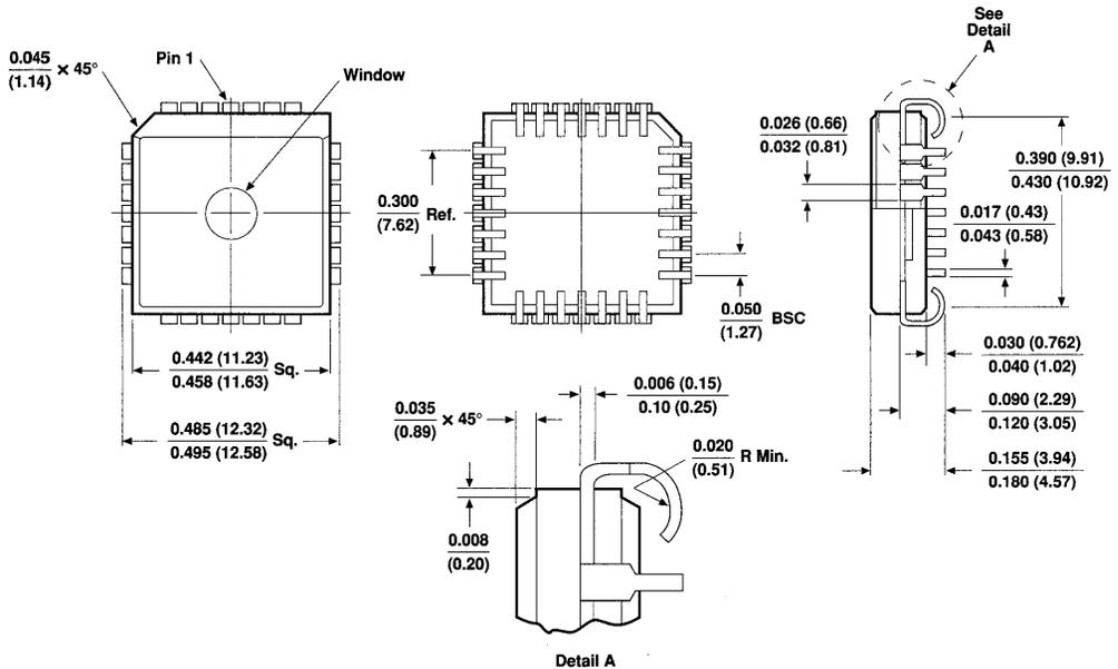
**28-Pin Plastic J-Lead Chip Carrier (PLCC)**
