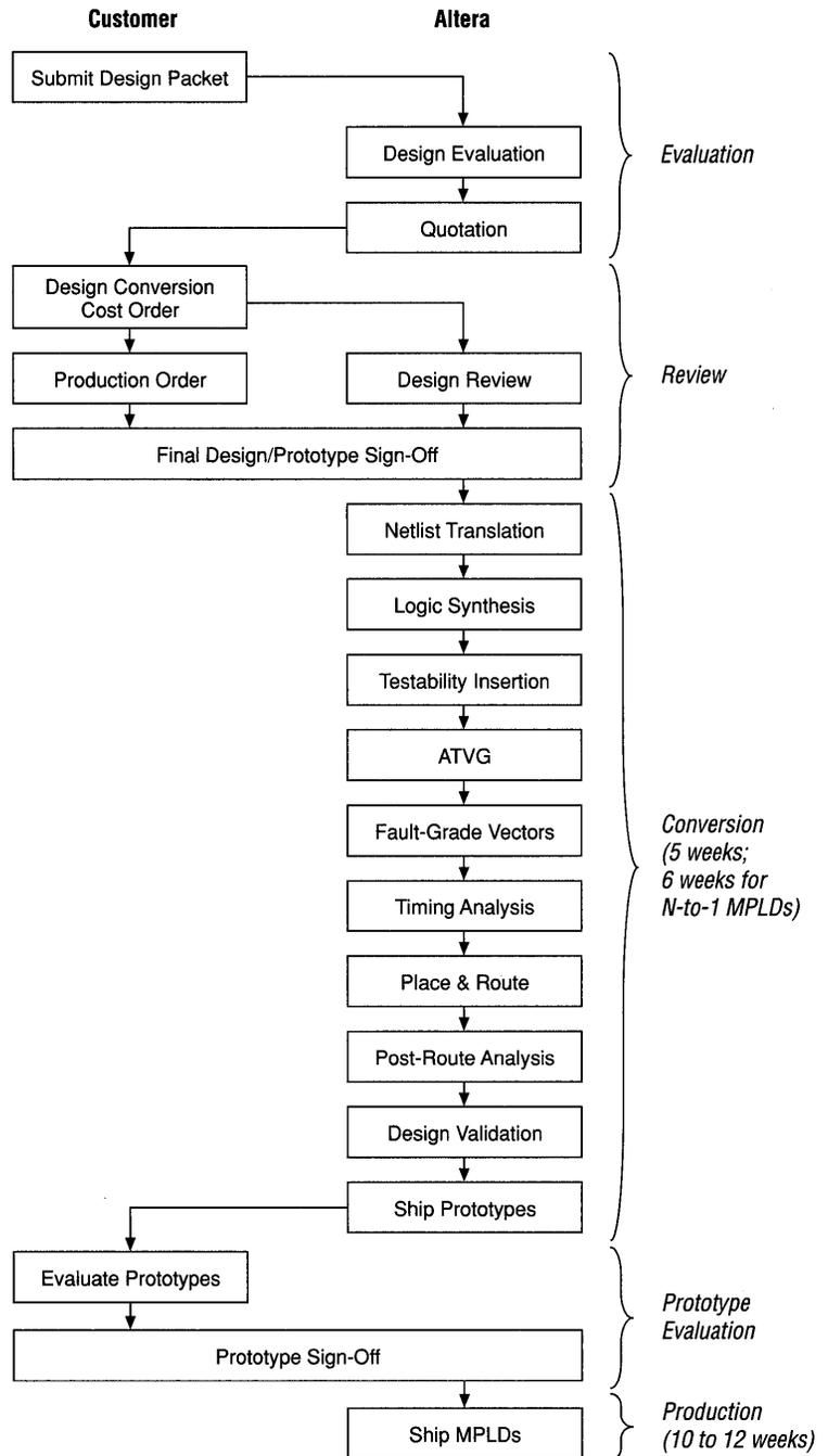
After the customer submits an order for the Design Conversion Cost (DCC), an Altera engineer reviews the design and submits a *Final Design Sign-Off Form* for customer approval. This form describes the specifications of the MPLD in detail. After the final design has been signed off, Altera begins the design conversion.
