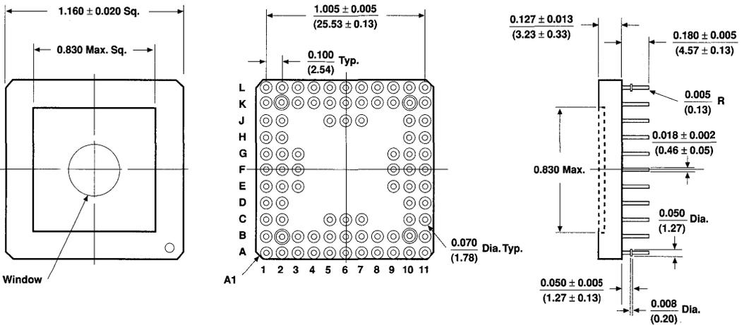
**100-Pin Small Outline Ceramic Pin-Grid Array (PGA)**
