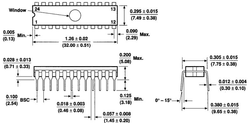
**24-Pin Plastic Dual In-Line Package (PDIP)**
