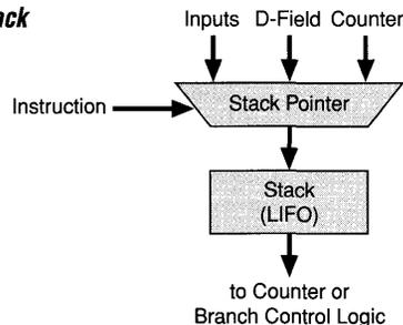
The pushing or popping of the stack occurs on the leading edge of the Clock. The stack is "zero-filled" so that a pop from an empty stack resets all 8 bits to zero. On the other hand, a push to a full stack writes over the top-of-stack, leaving the other 14 values unchanged.
