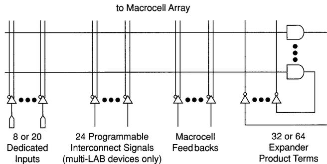
Expanders are fed by all signals in the LAB. One expander can feed all macrocells in the LAB or multiple product terms in the same macrocell. Since expanders also feed the secondary product terms of each macrocell, complex logic functions can be implemented without using additional macrocells. Expanders can also be cross-coupled to build additional flipflops, latches, or input registers. A small delay ( $t_{\text{EXP}}$ ) is incurred when shared expanders are used.
