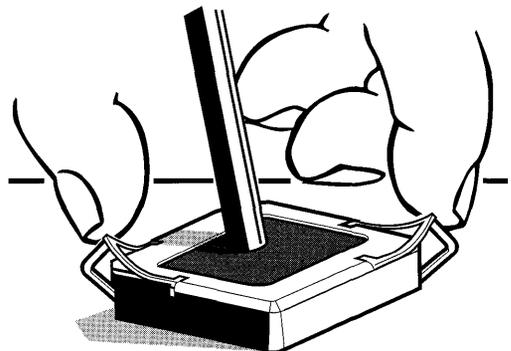
4. Lift the QFP carrier straight up. See Figure 7.
