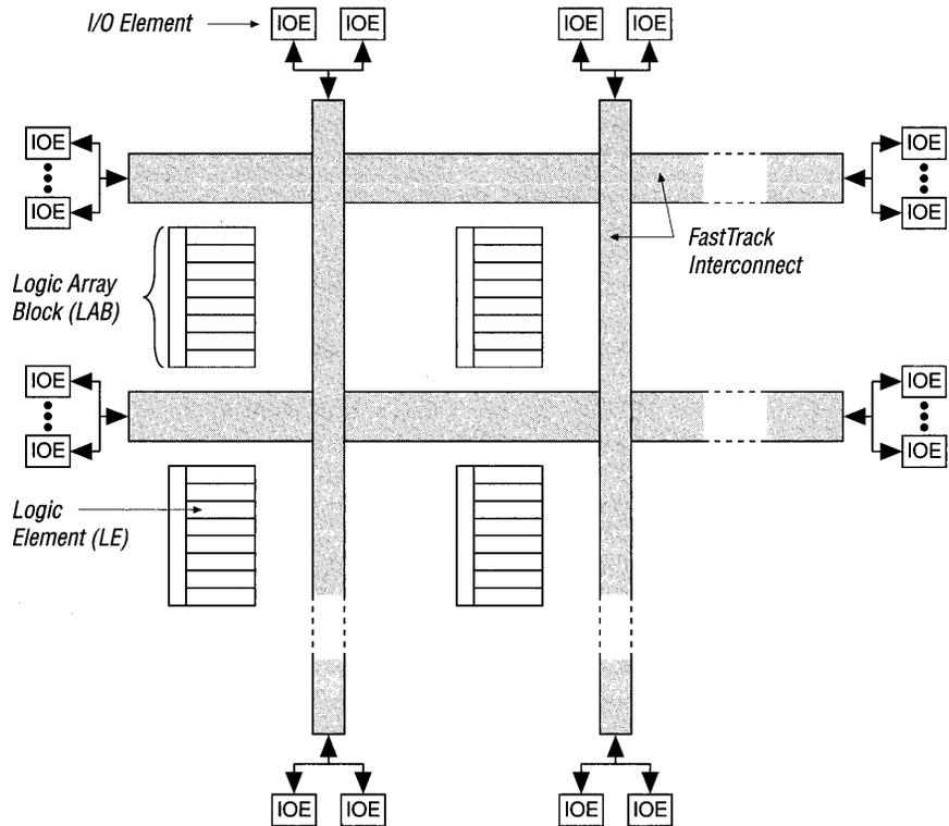
Signal interconnections within FLEX 8000 devices and to and from device pins are provided by the FastTrack Interconnect, a series of fast, continuous lines that run the entire length and width of the device. IOEs are located at the end of each row (horizontal) and column (vertical) FastTrack Interconnect path.
