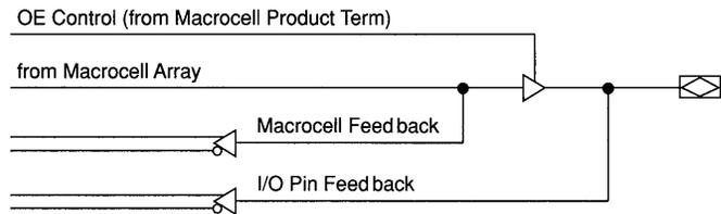
Each I/O pin in a MAX 5000 device provides dual feedback, i.e., a feedback path both before and after the tri-state buffer. Since the tri-state buffer decouples the I/O pins from the macrocells, all registers within the LAB can be “buried.” Thus, I/O pins can be configured as dedicated input, output, or bidirectional pins. Using an I/O pin as an input in single-LAB devices reduces the number of available expanders by two. In multi-LAB devices, I/O pins feed the PIA directly.
