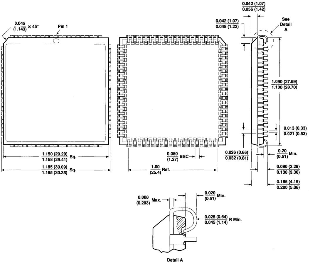
**84-Pin Small Outline Ceramic Pin-Grid Array (PGA)**
