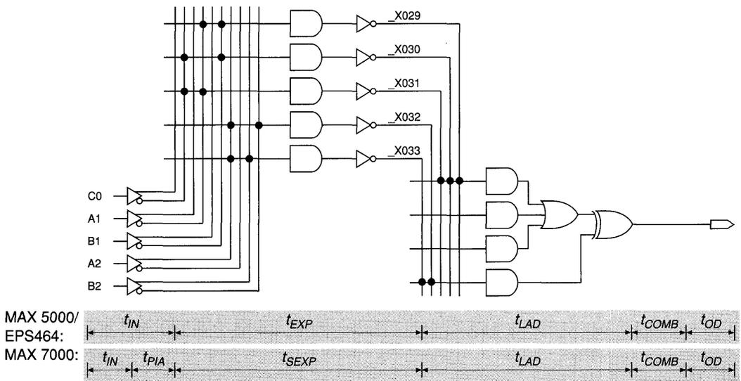
**Example 3: S2 Adder Bit With Parallel Expanders (MAX 7000)**
