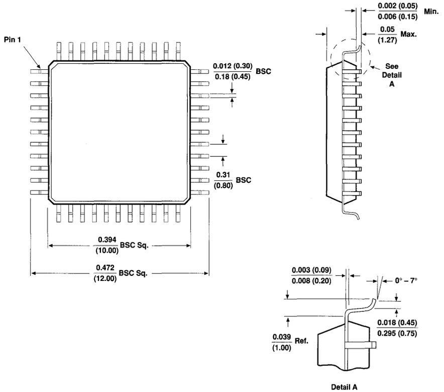
**68-Pin Ceramic J-Lead Chip Carrier (JLCC)**
