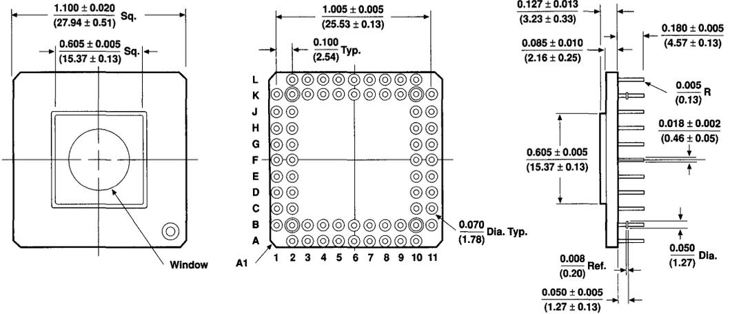
**68-Pin Large Outline Ceramic Pin-Grid Array (PGA)**
