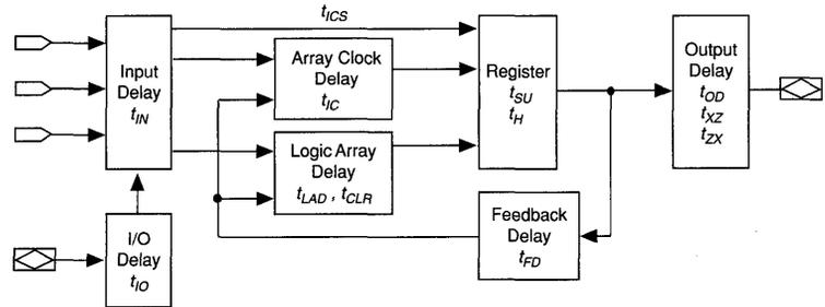
Timing information can be derived from the timing model and parameters for a particular EPLD. External timing parameters can be calculated from the sum of internal parameters and represent pin-to-pin timing delays. Figure 5 shows the internal timing relationship for internal and external delay parameters. For more information on EPLD timing, refer to *Application Brief 100 (Understanding EPLD Timing)* in this data book.
