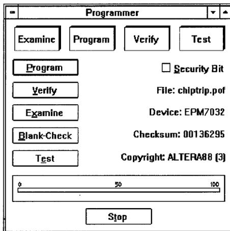
supports functional testing, so that vectors created for simulation can be applied to a programmed device to verify its functionality.
