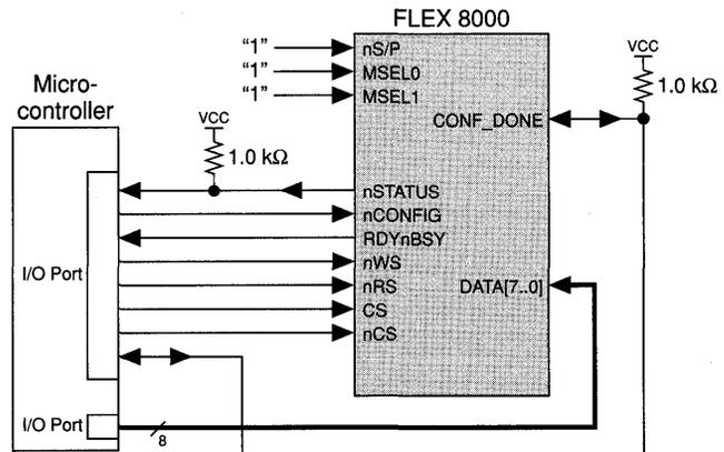
microcontroller is used as the intelligent host to ensure that sufficient dedicated I/O ports are available to drive all control signals and the data bus to the FLEX 8000 device. The chip select signals CS and nCS are both used to select the device. However, you can also tie nCS to GND and control chip selection with the CS pin only (or vice-versa), thus saving one bit in the I/O port.
