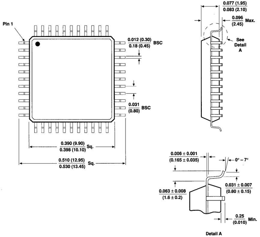
**44-Pin Thin Plastic Quad Flat Pack (TQFP)**
