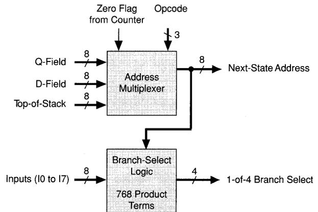
The address multiplexer provides the next-state address to the microcode memory. The next-state address can come from the Q-field, the D-field, or the top-of-stack. The selection is based on the instruction in the pipeline register and the condition of the zero flag from the counter.
