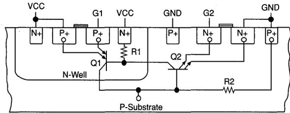
Figure 1 also shows the parasitic resistors that occur in the CMOS structure. Generally, these resistors are of no concern as long as currents do not flow through the structure laterally. However, I-R drops may occur in the structure if any of the associated diodes turn on. These diodes may be initially turned on by power-supply or I/O pin transients that exceed the limits of GND and  $V_{CC}$ . These transients can be induced by signal ringing and other inductive effects in the system.
