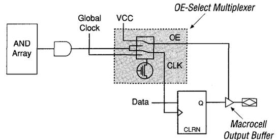
individually configured for each macrocell. In Mode 0, the tri-state output buffer is controlled by a single product term. If the output of the AND gate is high, the output buffer is enabled. If the output is low, the output buffer has a high-impedance value. In this mode, the macrocell flipflop is clocked by its global Clock input signal. (The EP330 supports only Mode 0.)
