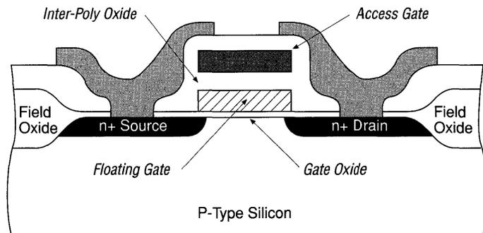
EPROM transistors are programmed to a high-threshold voltage with hot electron injection. When a programming voltage  $V_{PP}$  (normally 12.5 V) is applied to the access gate of an EPROM cell and a slightly lower voltage is applied to its drain, electrons flow from the source to the drain. As these electrons pick up kinetic energy, their path is altered by an electric field located between the access gate and substrate. This electric field is generated
