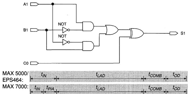
S1 is the output of macrocell 21 (`_LC021`), which contains combinatorial logic. The combinatorial logic `LCELL(_EQ026 $ C0)` represents the XOR of the intermediate equation `_EQ026` and the carry-in `C0`. In turn, `_EQ026` is logically equivalent to the XOR of inputs `B1` and `A1`. Therefore:
