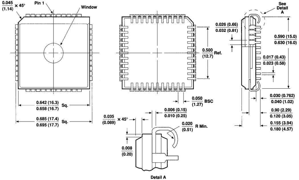
**44-Pin Plastic J-Lead Chip Carrier (PLCC)**
