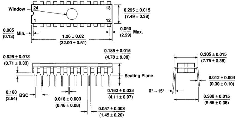
**24-Pin Plastic Dual In-Line Package (PDIP)**
