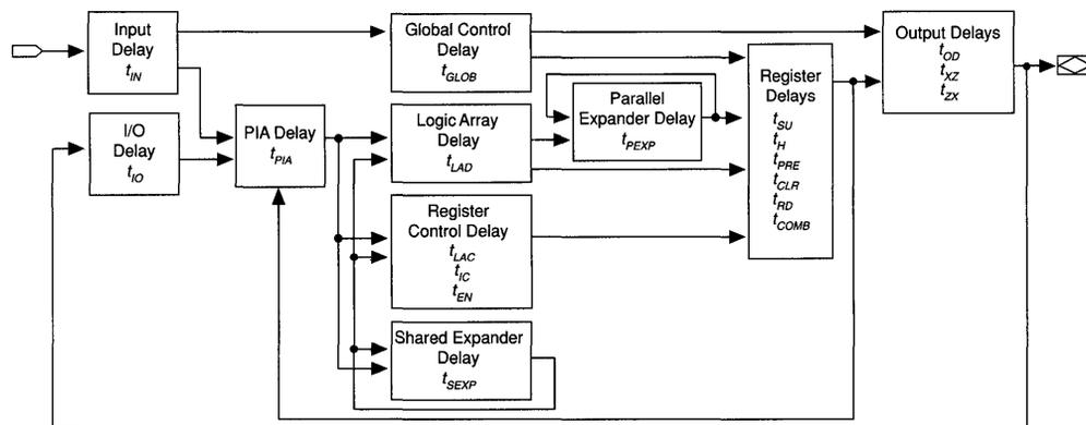
Timing information can be calculated with the timing model and parameters for a particular EPLD. External timing parameters are derived from the sum of internal parameters and represent pin-to-pin timing delays. Figure 8 shows the internal timing relationship for internal and external delay parameters. Timing can also be calculated in a timing simulation or timing analysis with MAX+PLUS II or with other industry-standard CAE tools.
