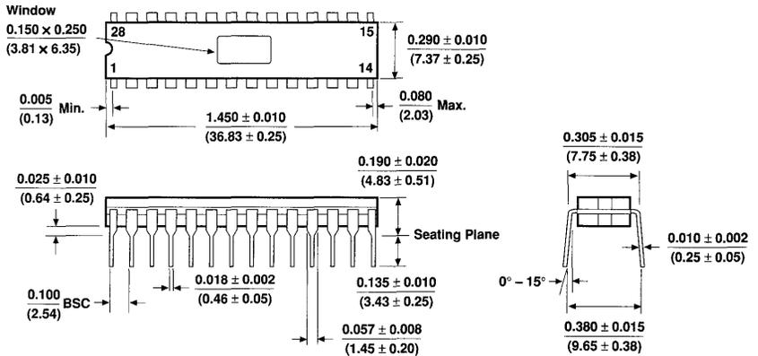
**28-Pin Plastic Dual In-Line Package (PDIP)**
