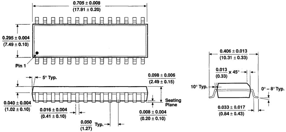
**28-Pin Ceramic J-Lead Chip Carrier (JLCC)**
