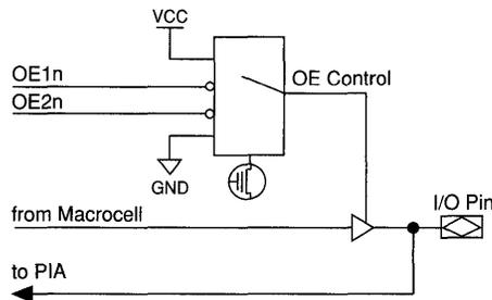
The EPM7032V provides dual I/O feedback, in which macrocell and pin feedbacks are independent. When an I/O pin is configured as an input, the associated macrocell can be used for buried logic.
