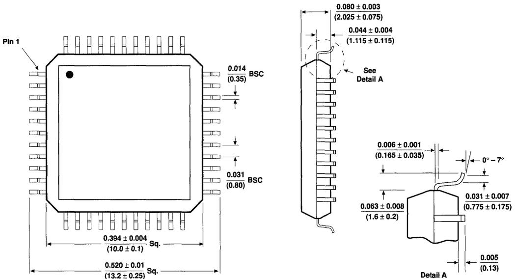
**44-Pin Thin Plastic Quad Flat Pack (TQFP)**
