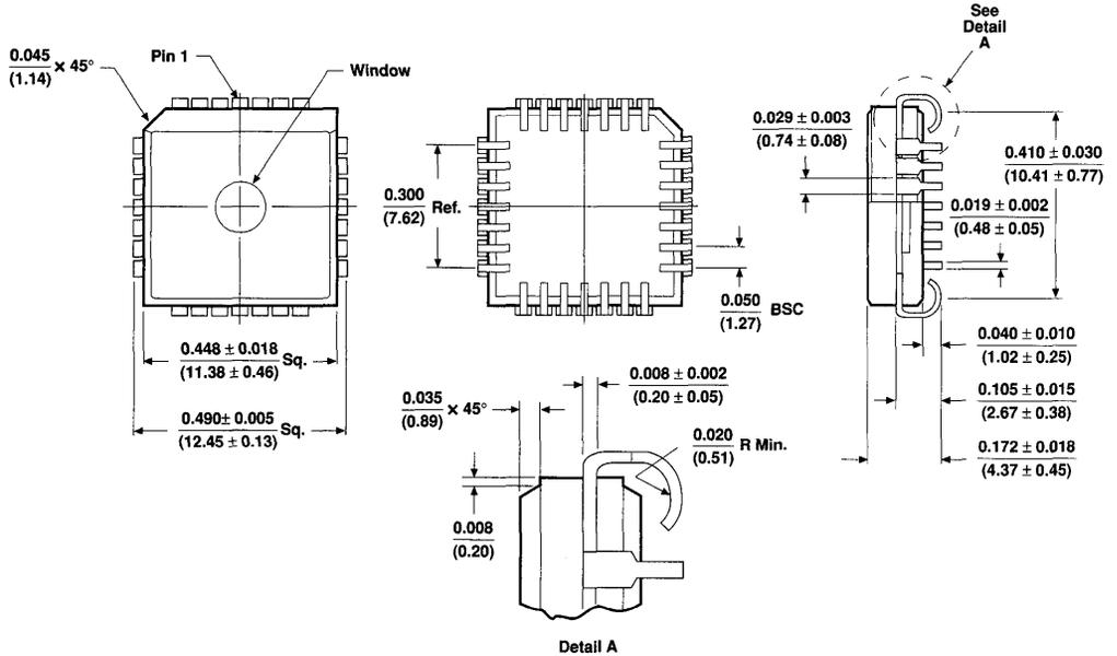
**28-Pin Plastic J-Lead Chip Carrier (PLCC)**
