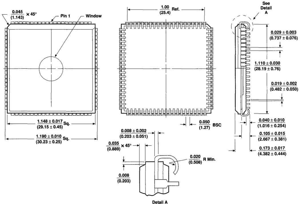
**84-Pin Plastic J-Lead Chip Carrier (PLCC)**
