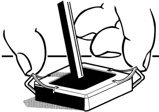
4. Lift the QFP carrier straight up. See Figure 7.
