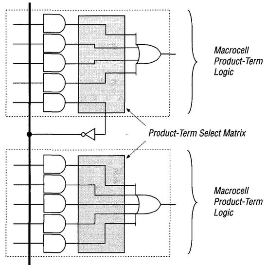
Parallel expanders are unused product terms from macrocells in the LAB. The product-term select matrix can allocate parallel expanders to any neighboring macrocell to implement fast, complex logic functions. With parallel expanders, up to 20 product terms can directly feed the macrocell OR logic—5 product terms from the macrocell and 15 parallel expanders provided by neighboring macrocells in the LAB.
