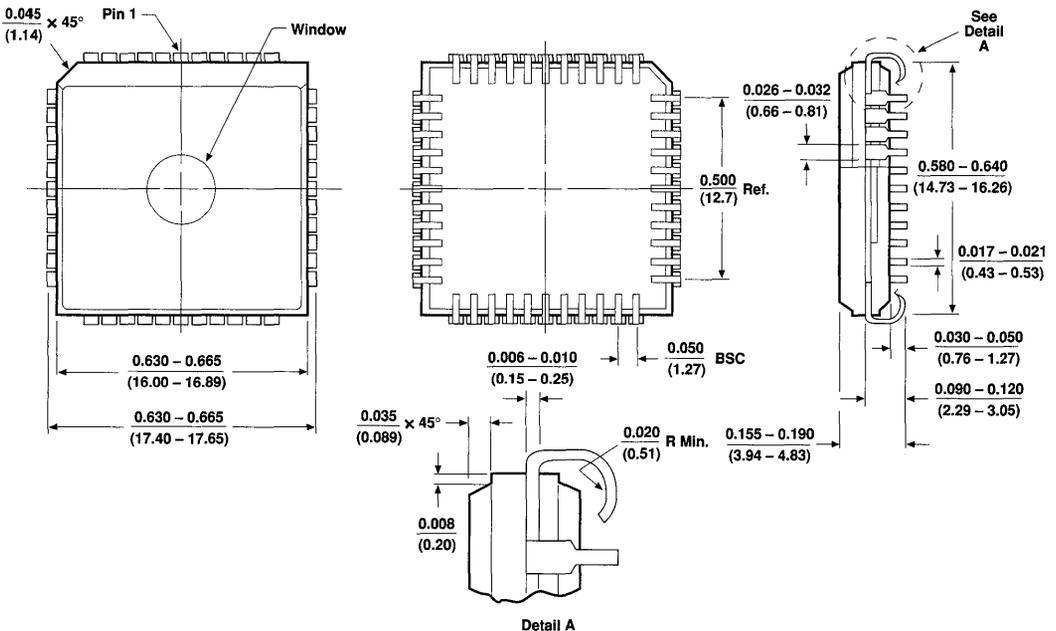
**44-Pin Plastic J-Lead Chip Carrier (PLCC)**
