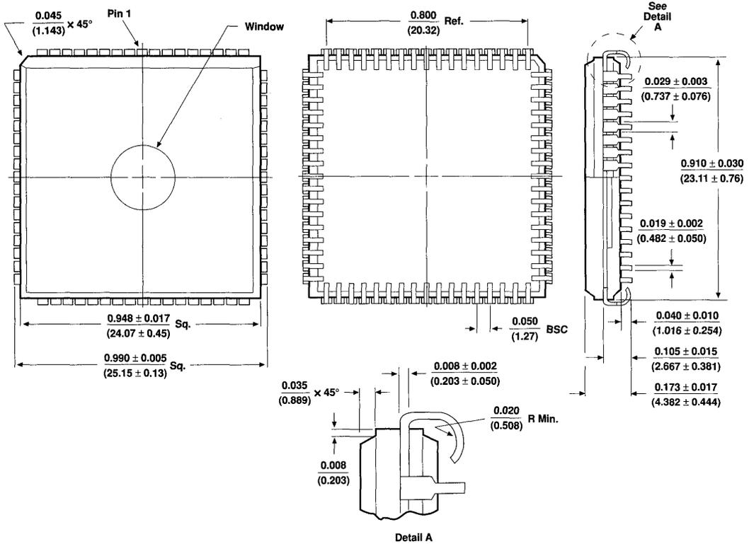
**68-Pin Plastic J-Lead Chip Carrier (PLCC)**
