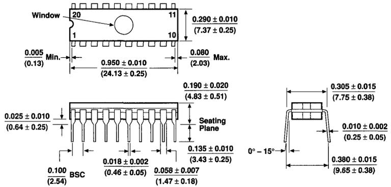
**20-Pin Plastic Dual In-Line Package (PDIP)**
