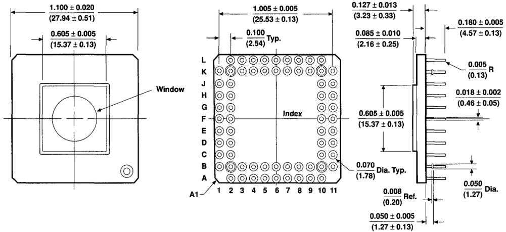
**84-Pin Ceramic J-Lead Chip Carrier (JLCC)**
