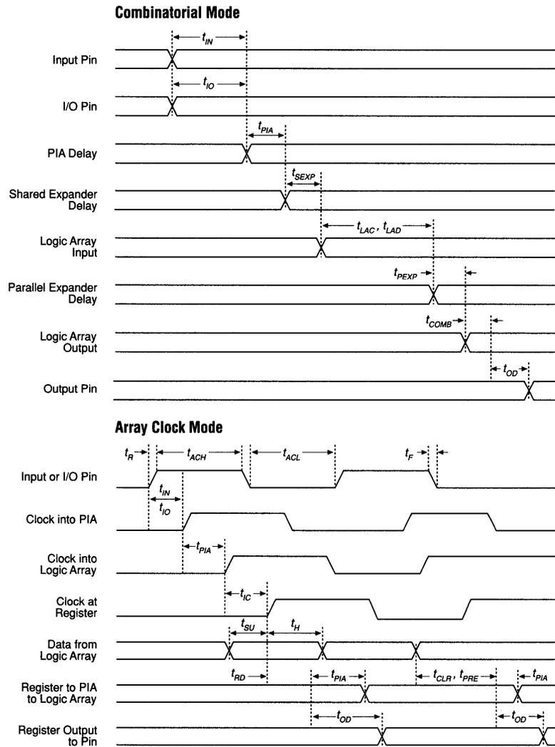
Figure 6. Switching Waveforms (Part 2 of 2)
