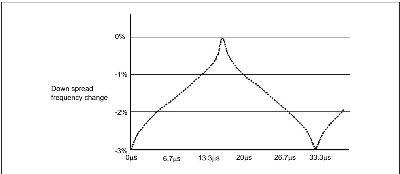
Analysis was done to show that, with a PLL bandwidth of 100x the modulation frequency and a phase angle  $\ll 0.1$  degrees, tracking skew should be manageable. For the 405GP the tracking skew for up to a -3% variation in the SysClk frequency modulated at 30 kHz ranges from -77.5 to -185 ps depending on the VCO frequency. Tracking skew in pico seconds can be determined using the following formula.
