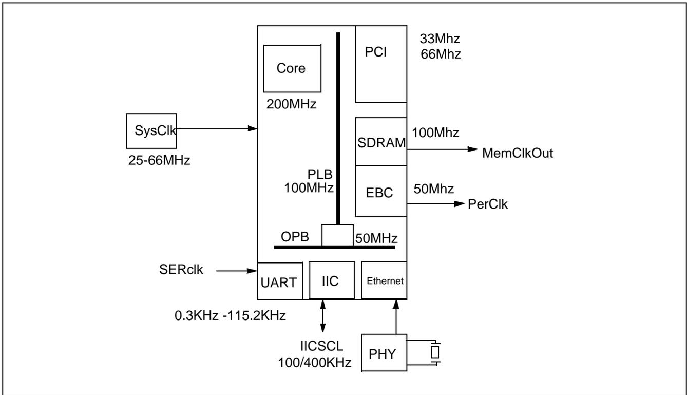
The clocking for the chip is derived from the input clock. Figure 4 is a simple representation of how the various clocks are derived from the system clock. The effect of using a SSCG must be examined for each interface.
