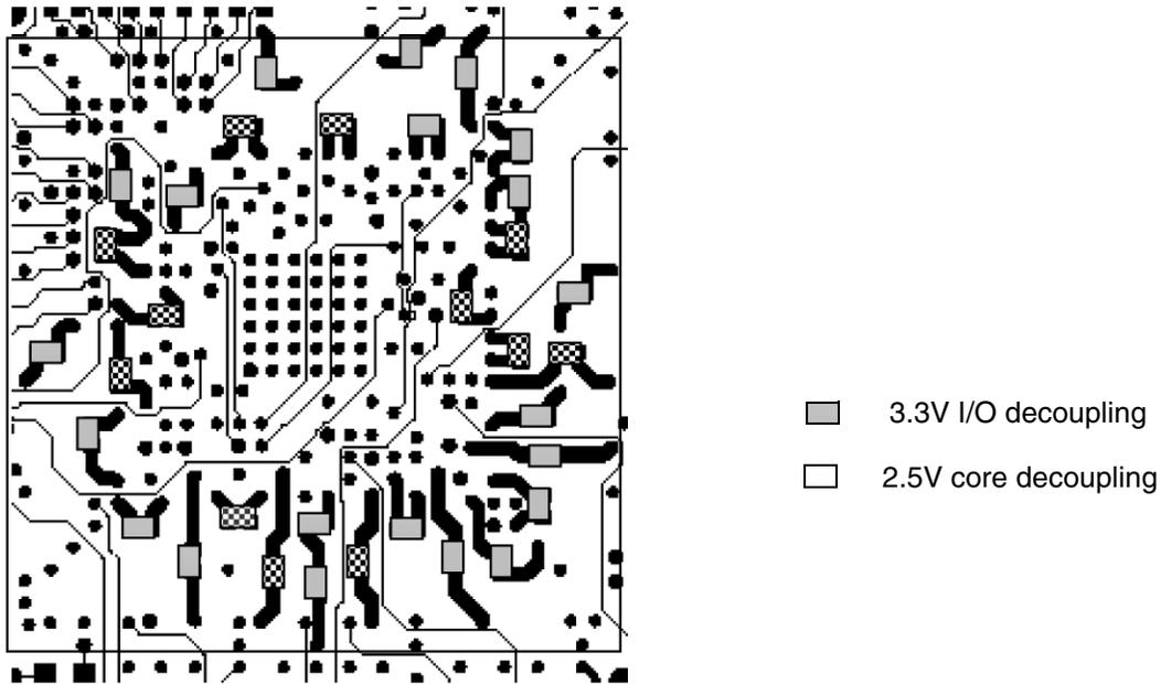
Figure 6. Decoupling Capacitors
