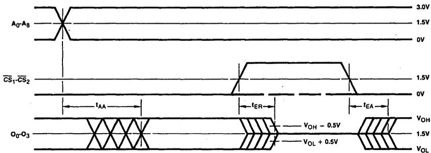
Note: Level on output while either  $\overline{CS}$  is HIGH is determined externally.
