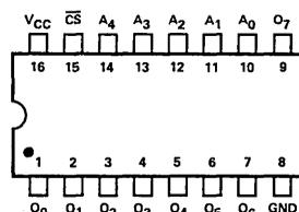
Note: Pin 1 is marked for orientation.
