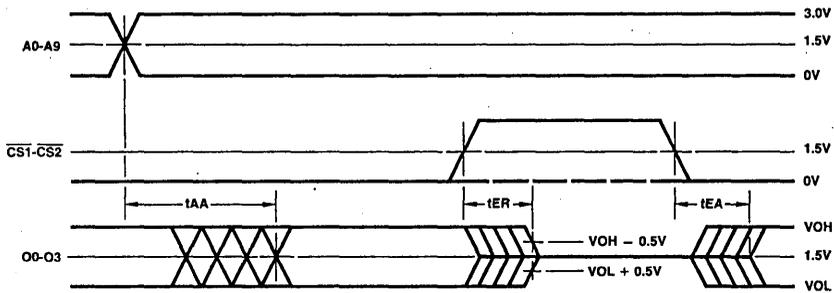
Note: Level on output while either CS is HIGH is determined externally.
