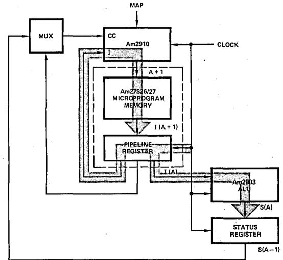
A Register at the Microprogram Memory output contains the microinstruction being executed. The microprogram memory and Am2903 delay are in series. Conditional branches are executed on same cycle as the ALU operation generating the condition.
