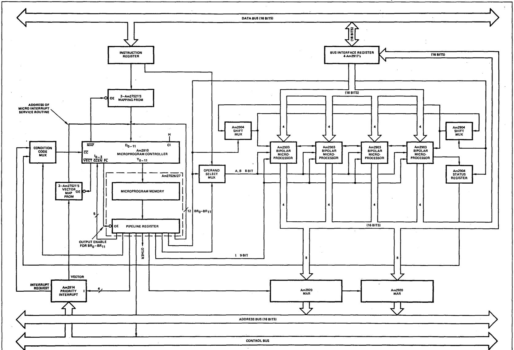
Fig. 3. Typical Bipolar Microcomputer using the Am27S26/27.
