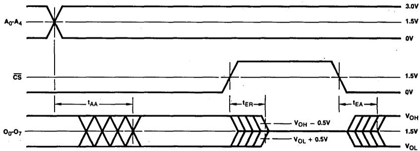
Note: Level on output while  $\overline{CS}$  is HIGH is determined externally.
