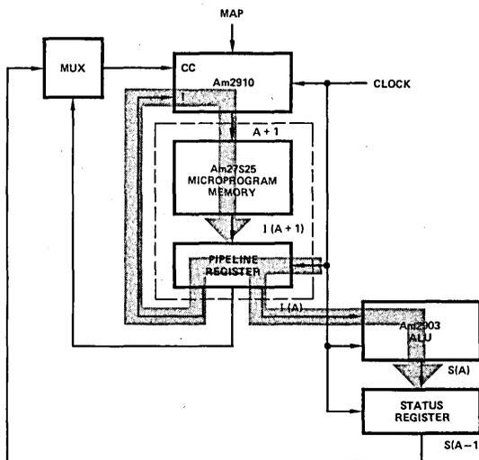
One level pipeline provides better speed than the architecture to the left. The Microprogram Memory and the Am2903 array are in parallel speed paths instead of in series. This is the recommended architecture for Am2900 designs. Note that the Am27S25 reduces the parts count of the microprogram memory/pipeline by a factor of two.
