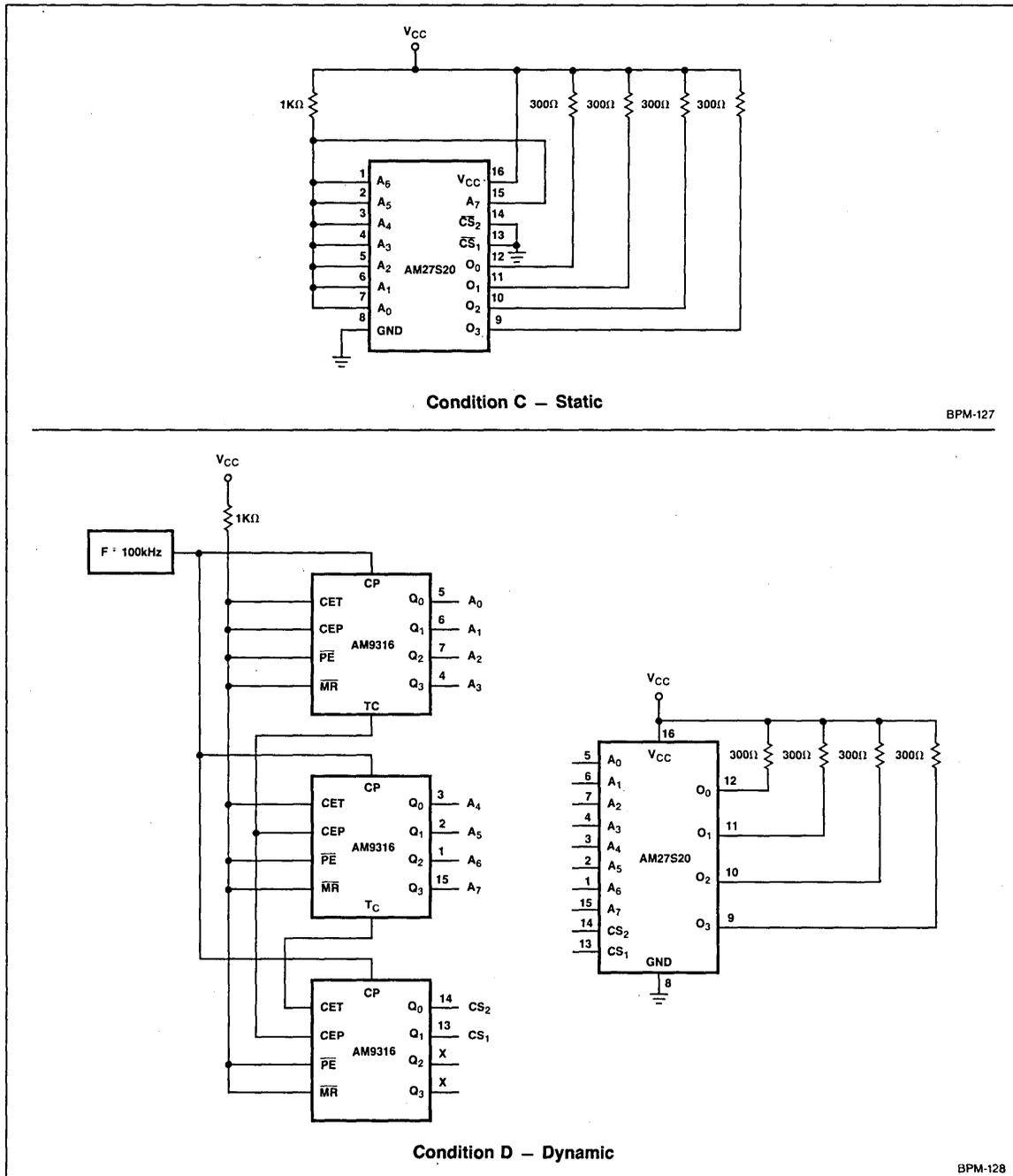
Figure 9. Burn-In Circuits For Conditions C & D-27S20.
