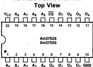
Note: Pin 1 is marked for orientation.
