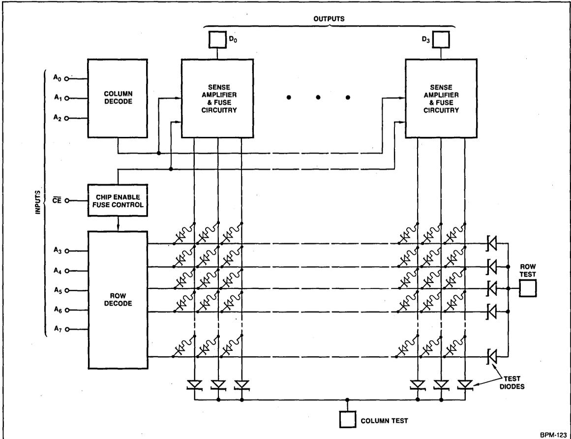
Figure 4. PROM Circuitry Block Diagram.
