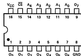
Note: Pin 1 is marked for orientation.
