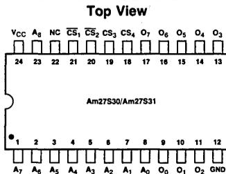
Note: Pin 1 is marked for orientation.
