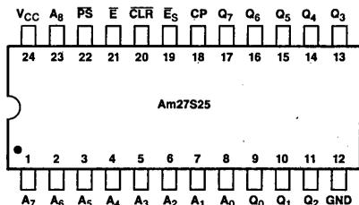
Note: Pin 1 is marked for orientation.
