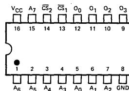
Note: Pin 1 is marked for orientation.
