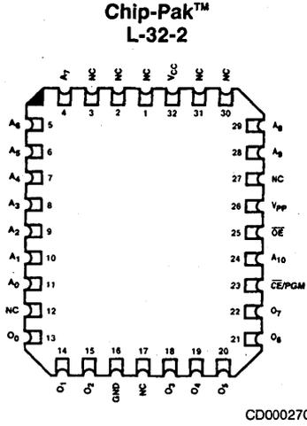
Note: Pin 1 is marked for orientation
