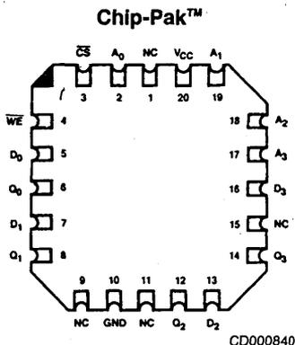
Note: Pin 1 is marked for orientation
