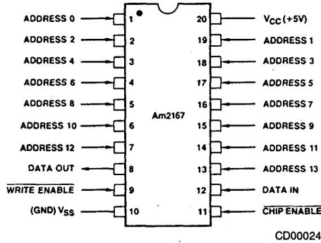
Note: Pin 1 is marked for orientation
