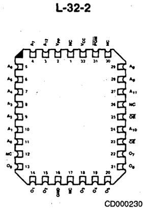
Note: Pin 1 is marked for orientation
