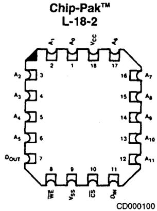
Note: Pin 1 is marked for orientation
