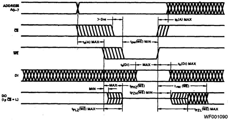
Write Cycle Timing. The cycle is initiated by an address change. After  $t_{s(A) \text{ max}}$ , the write enable may begin. The chip select must also be LOW for writing. Following the write pulse,  $t_{h(A) \text{ max}}$  must be allowed before the address may be changed again. The output will be inactive (floating for the Am27LS00-1A/00-1) while the write enable is LOW. Ordinarily, the chip select should be LOW during the entire write pulse.
