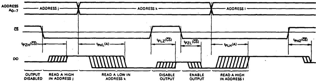
Switching delays from address and chip select inputs to the data output. For the Am27LS00-1A/00-1 disabled output is "OFF," represented by a single center line. For the Am27LS01-1A/01-1, a disabled output is HIGH.
