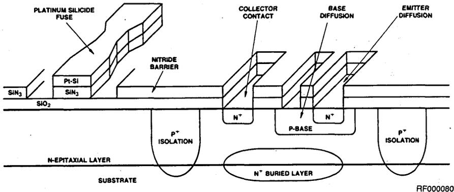
Figure 2. Transistor & Fuse Structures.
