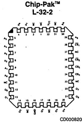
Note: Pin 1 is marked for orientation
