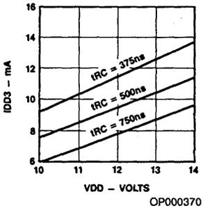
Typical Page Mode Current  $I_{DD4}$  Versus  $V_{DD}$
