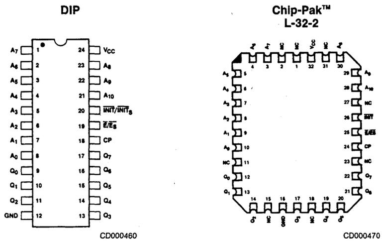
Note: Pin 1 is marked for orientation
