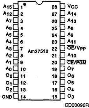
Note: Pin 1 is marked for orientation
