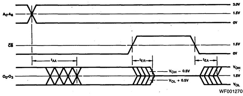
Note: Level on output while CS is HIGH is determined externally.
