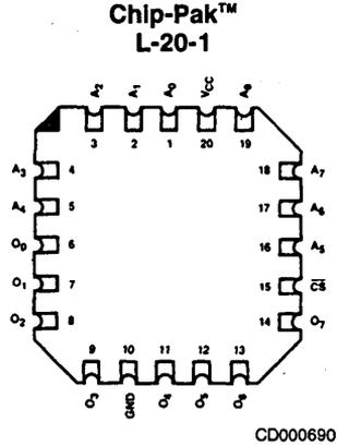
Note: Pin 1 is marked for orientation
