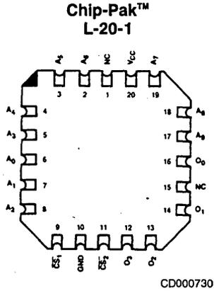
Note: Pin 1 is marked for orientation
