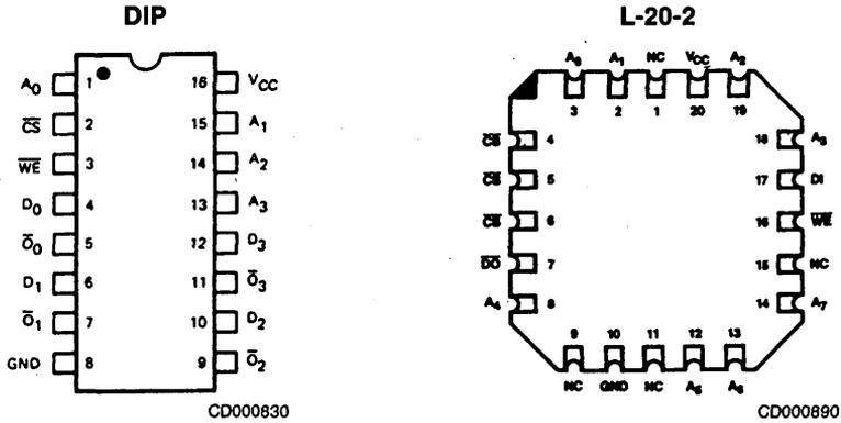
Note: Pin 1 is marked for orientation
