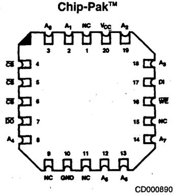
Note: Pin 1 is marked for orientation
