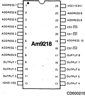
Note: Pin 1 is marked for orientation
