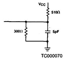
**Figure 2. Output Load for tHZ, tLZ, tOW, tWZ**
