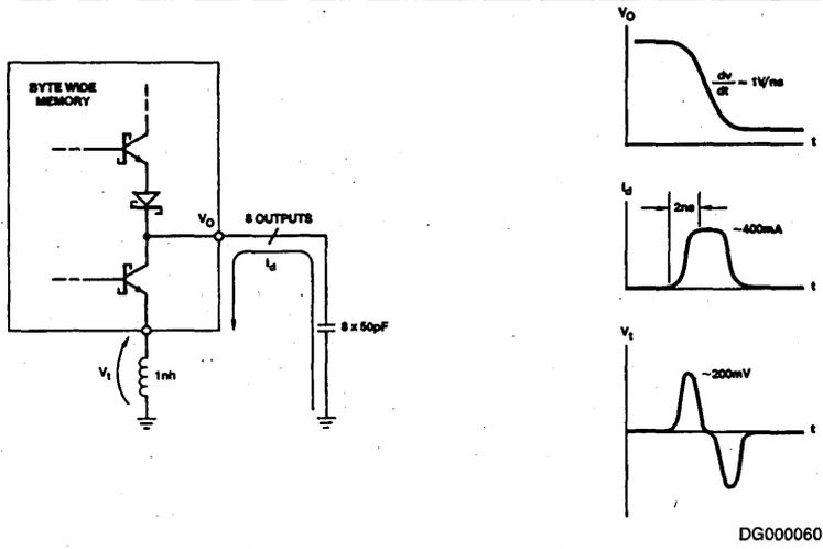
Figure 6. Byte Wide Memory Ground Transients
