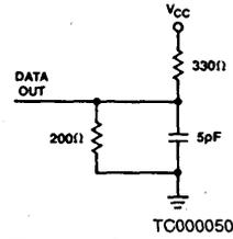
Figure 2. Output Load for  $t_{HZ}$ ,  $t_{LZ}$ ,  $t_{OW}$ ,  $t_{WZ}$
