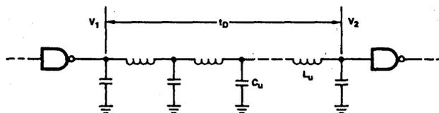
The unit length capacitance and inductance ( $C_u$  and  $L_u$ ) give each system connection transmission line characteristics. Without a matched termination, switching at  $V_1$  causes reflection voltages to appear at  $V_2$ , reducing noise immunity.
