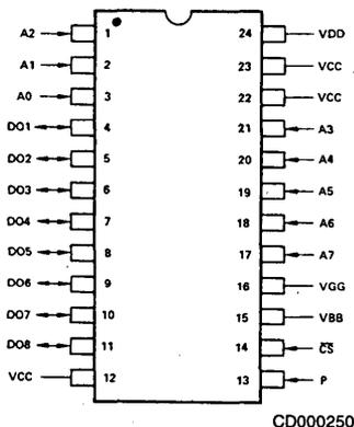
Note: Pin 1 is marked for orientation
