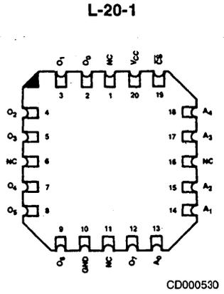
Note: Pin 1 is marked for orientation
