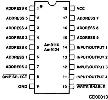
Note: Pin 1 is marked for orientation
