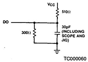
**Figure 1. Output Load**
