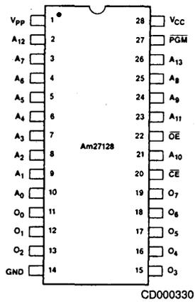
Note: Pin 1 is marked for orientation
