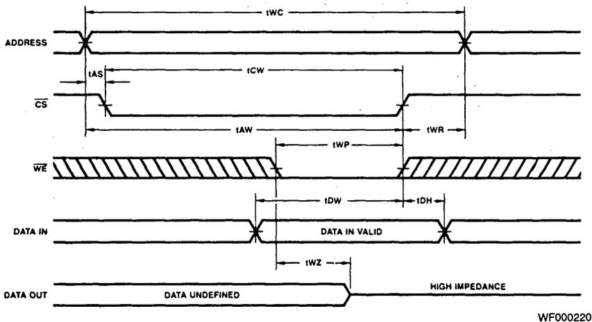
Note: If  $\overline{CE}$  goes high simultaneously with  $\overline{WE}$  high, the output remains in a high impedance state.
