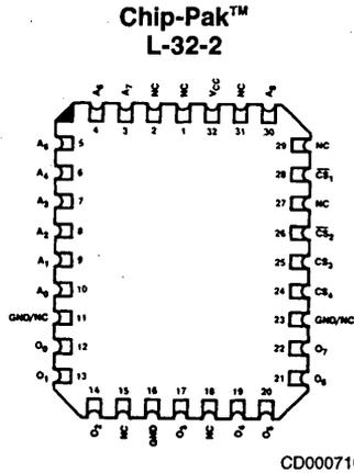
Note: Pin 1 is marked for orientation
