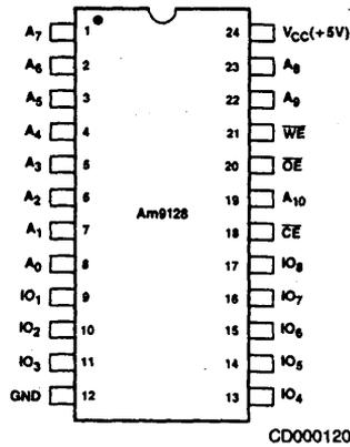
Note: Pin 1 is marked for orientation
