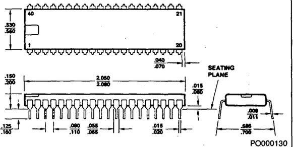
Note. Standard lead finish is tin plate or solder dip.
