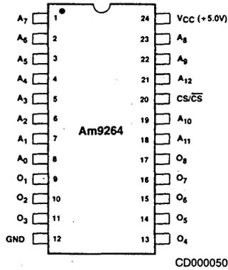
Note: Pin 1 is marked for orientation
