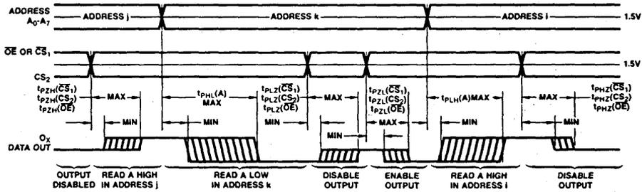
Switching delays form address input, output enable input and the chip select inputs to the data output. For the Am93422A/422 disabled output is "OFF", represented by a single center line. For the Am93412A/412, a disabled output is HIGH.
