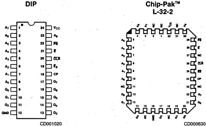
Note: Pin 1 is marked for orientation
