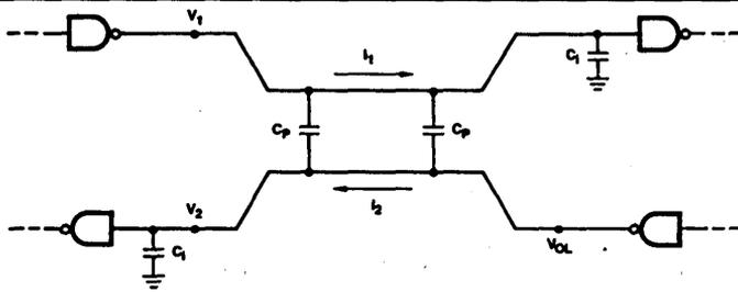
As  $V_1$  switches,  $I_1$  flows to charge the input capacitance  $C_i$ .  $I_2$  flows as a result of mutual inductance. The  $V_1$  voltage change is also coupled directly to  $V_2$  through the parasitic line-to-line capacitances,  $C_p$ .
