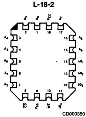
Note: Pin 1 is marked for orientation
