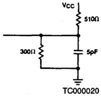
Figure 2. Output Load for  $t_{HZ}$ ,  $t_{LZ}$ ,  $t_{OW}$ ,  $t_{wZ}$
