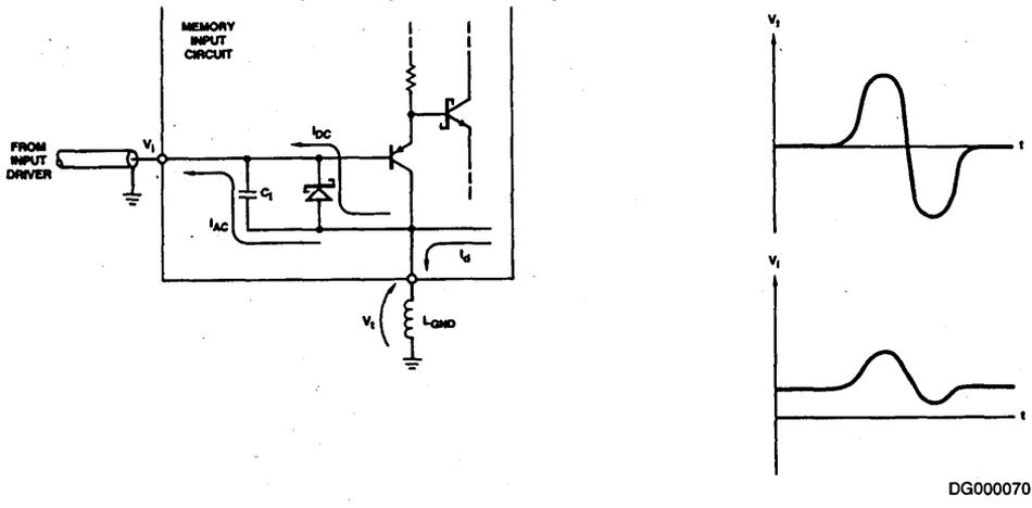
For small magnitudes of noise,  $V_t$ , noise is AC coupled to the inputs through the input capacitance,  $C_i$ . If  $V_i$  is low, large
