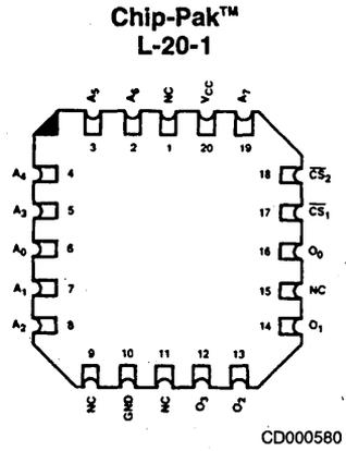
Note: Pin 1 is marked for orientation
