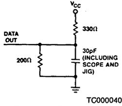
Figure 1. Output Load
