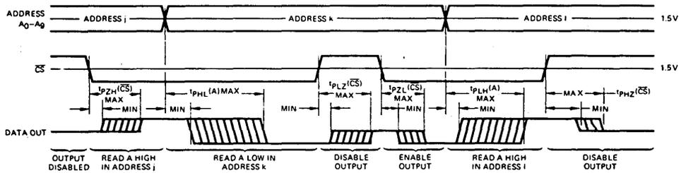
Switching delays from address and chip select inputs to the data output. For the Am93425A/425 disabled output is "OFF", represented by a single center line. For the Am93415A/415 a disabled output is HIGH.
