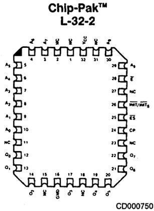
Note: Pin 1 is marked for orientation
