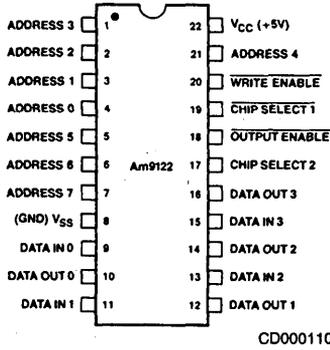
Note: Pin 1 is marked for orientation
