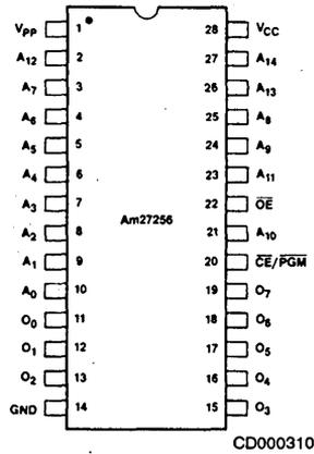
Note: Pin 1 is marked for orientation
