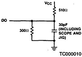
Figure 1. Output Load
