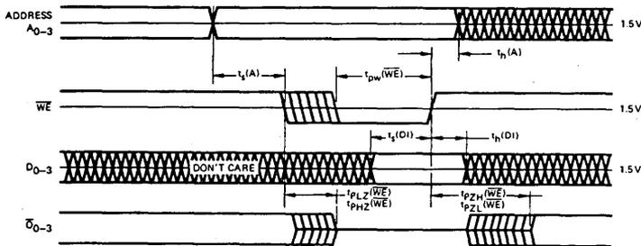
Write Cycle Timing. The cycle is initiated by an address change. After  $t_s(A)$  min, the write enable may begin. The chip select must also be LOW for writing. Following the write pulse,  $t_h(A)$  min must be allowed before the address may be changed again. The output will be inactive (floating for the Am27S03A/03) while the write enable is ( $\overline{WE}$ ) LOW.
