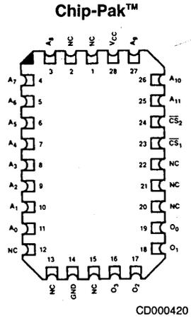
Note: Pin 1 is marked for orientation
