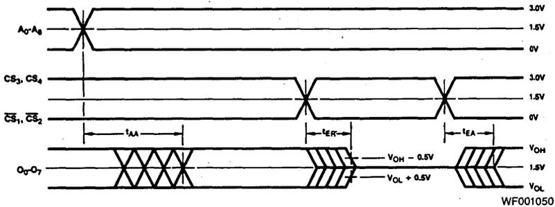
Note: Level on output while chip is disabled is determined externally.
