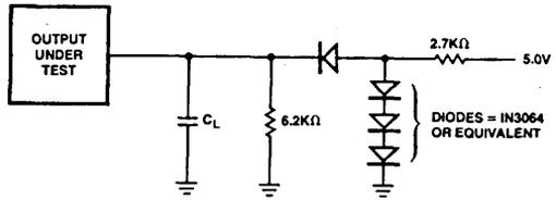
$C_L = 100\text{pF}$ , including jig capacitance
