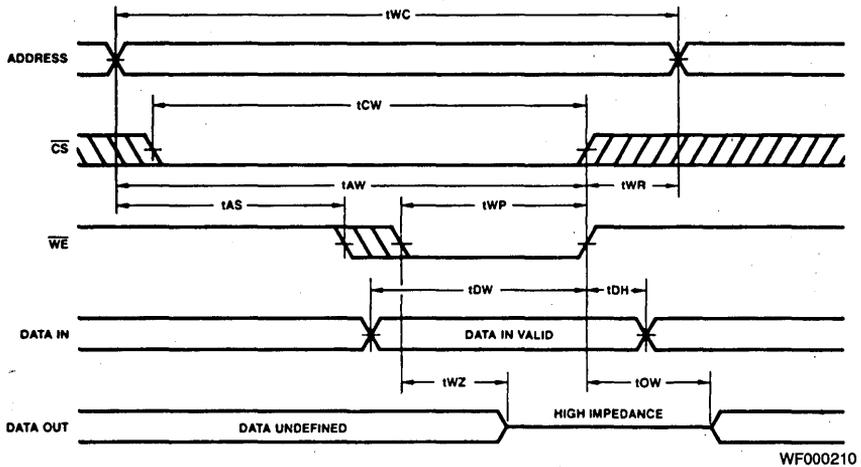
WRITE CYCLE NO. 2 ( $\overline{CS}$  CONTROLLED)
