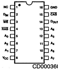
Note: Pin 1 is marked for orientation
