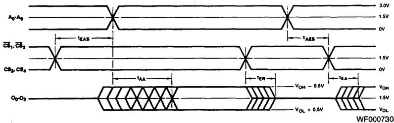
Note: Level on output while chip is disabled is determined externally.
