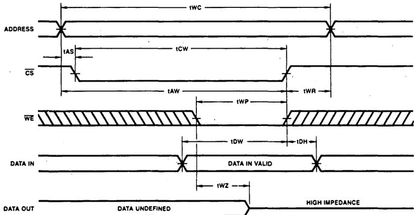
Note: If  $\overline{CS}$  goes high simultaneously with  $\overline{WE}$  high, the output remains in a high impedance state.
