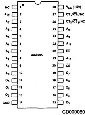
Note: Pin 1 is marked for orientation
