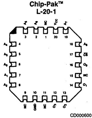
Note: Pin 1 is marked for orientation
