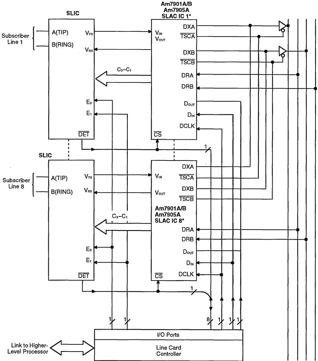
\*1/2 of an Am79C02 DSLAC IC per line can be used.
