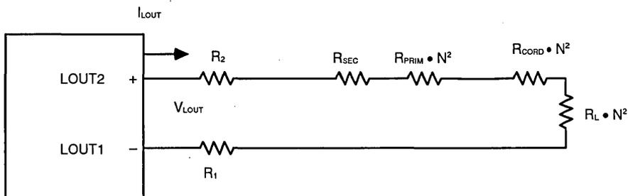
$R_{SEC}$  is the DC impedance of the transformer secondary (IC side of transformer).
