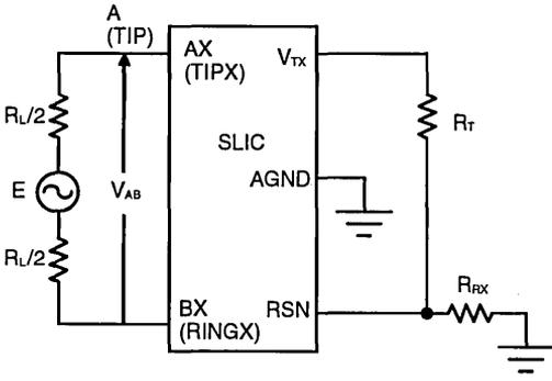
$$L_{2-4} = -20 \log (V_{TX} / V_{AB})$$
