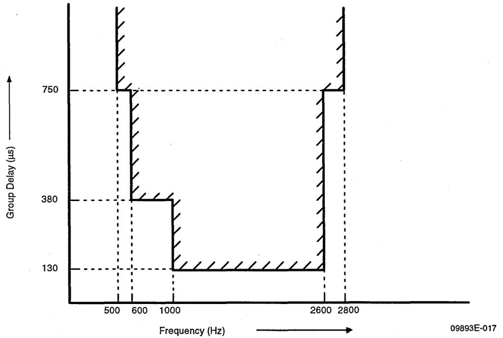
Figure 14. Group Delay Variation with Frequency (Transmit)
