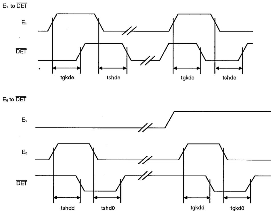
Note: All delays measured at 1.4-V level.
