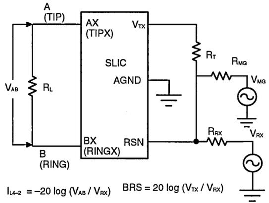
$$I_{L4-2} = -20 \log (V_{AB} / V_{RX}) \quad BRS = 20 \log (V_{TX} / V_{RX})$$
