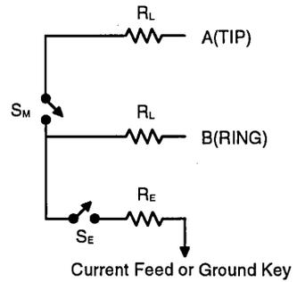
F. Ground-Key Detection Center Point Test
