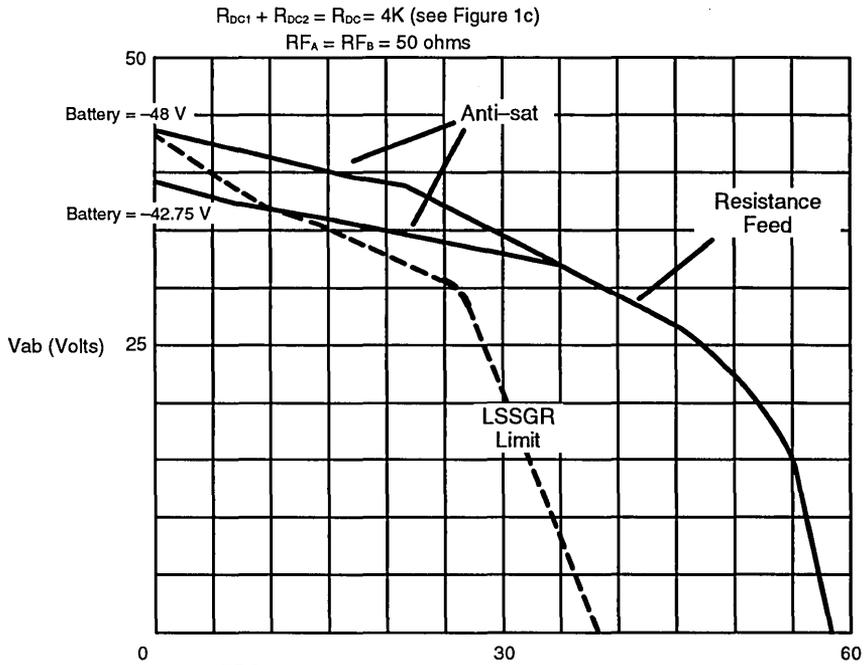
Resistance Feed Region:  $V_{ab} = 50 - \left( \frac{R_{DC}}{10} + R_{FA} + R_{FB} \right) I_L$
