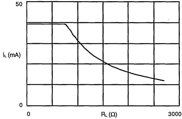
Load Current versus Load Resistance – Am79M531/Am79M535
