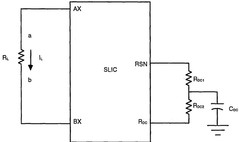
Current programmed by  $R_{DC1}$  and  $R_{DC}$ .
