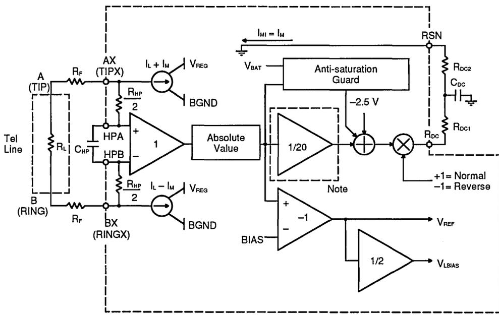
Note: The 1/20 operational amplifier is only present in constant resistance feed versions of the SLIC.
