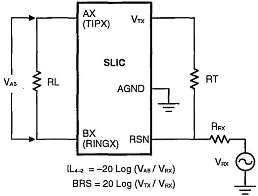
$$IL_{4-2} = -20 \text{ Log } (V_{Ab} / V_{Rx})$$
