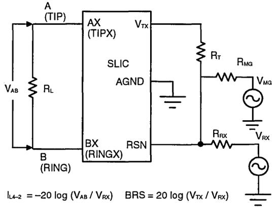
$$L_{4-2} = -20 \log (V_{AB} / V_{RX}) \quad BRS = 20 \log (V_{TX} / V_{RX})$$
