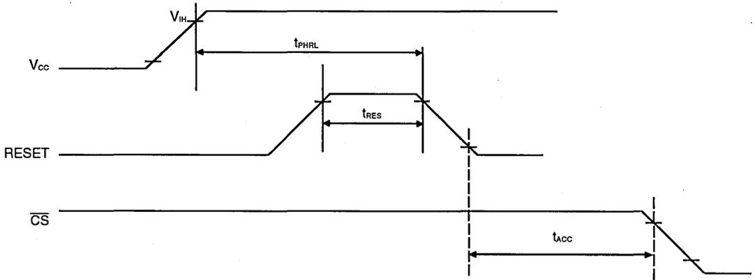
Figure 9. Reset Timing
