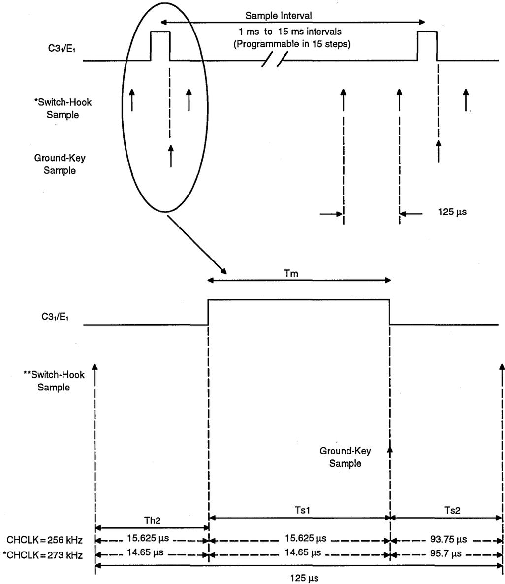
\*Programmed through CHF bit in Ground-Key Sampling Internal Register.
