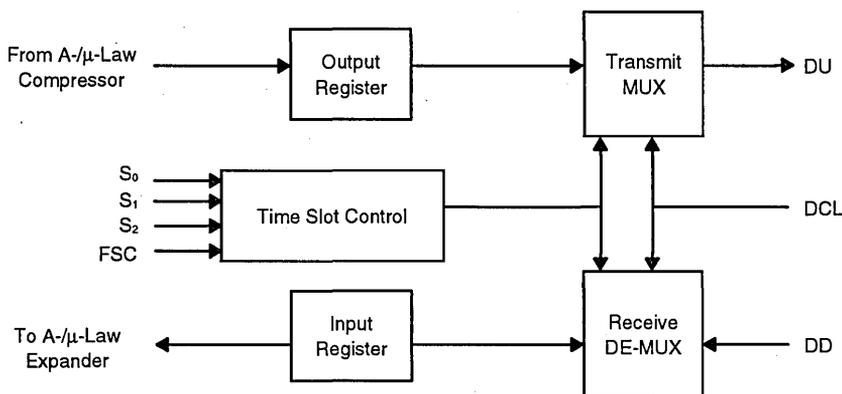
Figure 13. Time Slot Control and IOM 2 Interface
