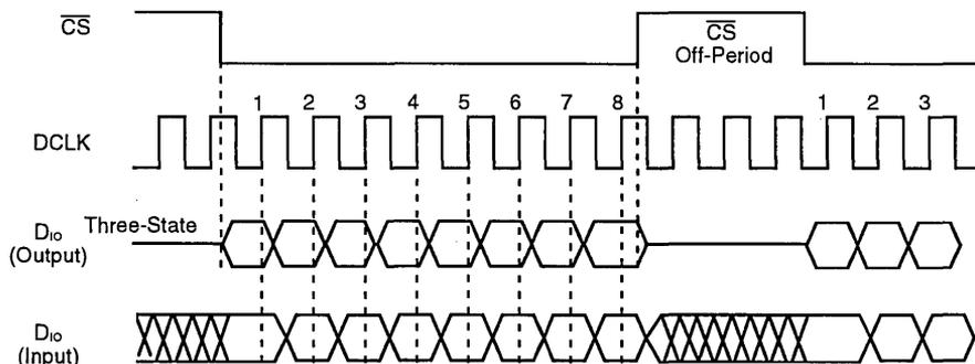
Figure 10. Serial I/O Interface Timing Diagram
