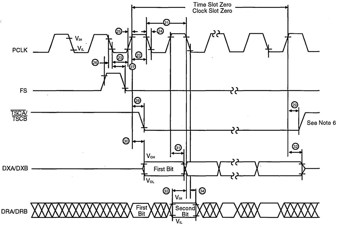
Note: In this mode, the PCM transmit timing is compatible with other CODEC IC's.
