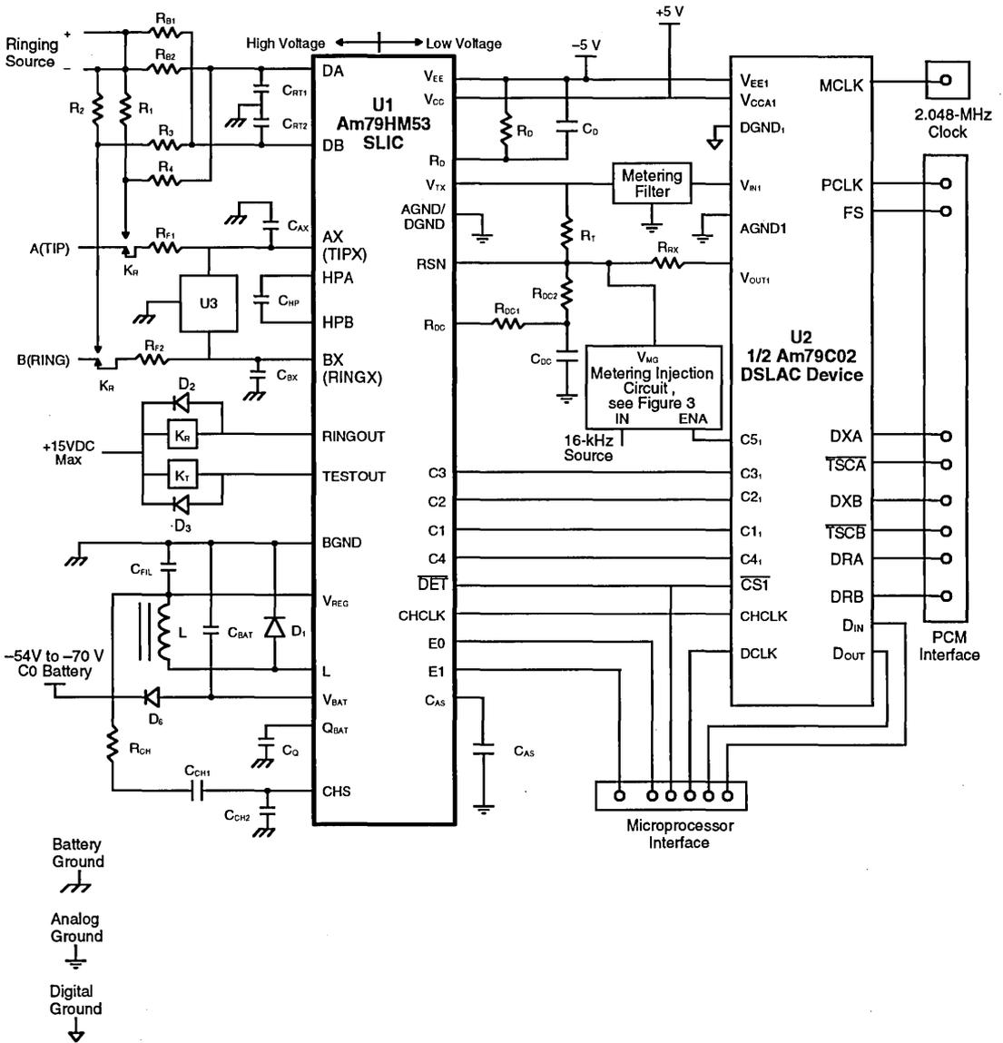
Figure 1. Single Channel of a Dual Channel Metering Subscriber Line Circuit
