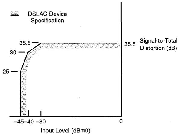
Figure 17. Total Distortion with Tone Input (Both Paths)
