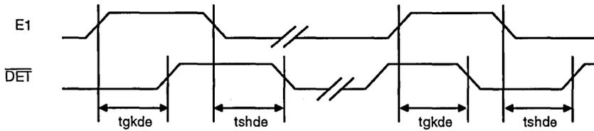
Note: All delays measured at 1.4-V levels.
