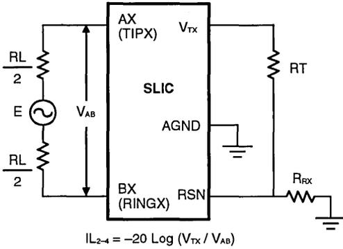
$$IL_{2-4} = -20 \text{ Log } (V_{Tx} / V_{Ab})$$
