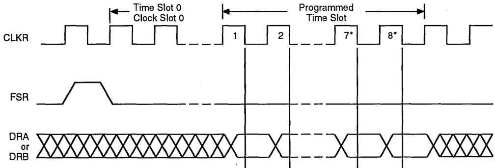
\*For linear code, the 7th and 8th clock cycles correspond to the 15th and 16th clock cycles.
