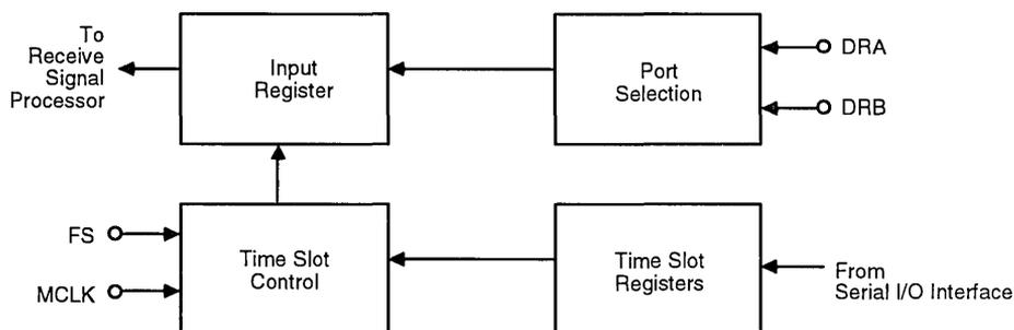
Figure 6. Receive PCM Interface
