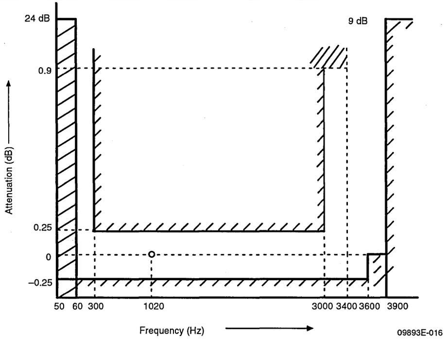
Figure 13. Attenuation/Frequency Distortion (Transmit)
