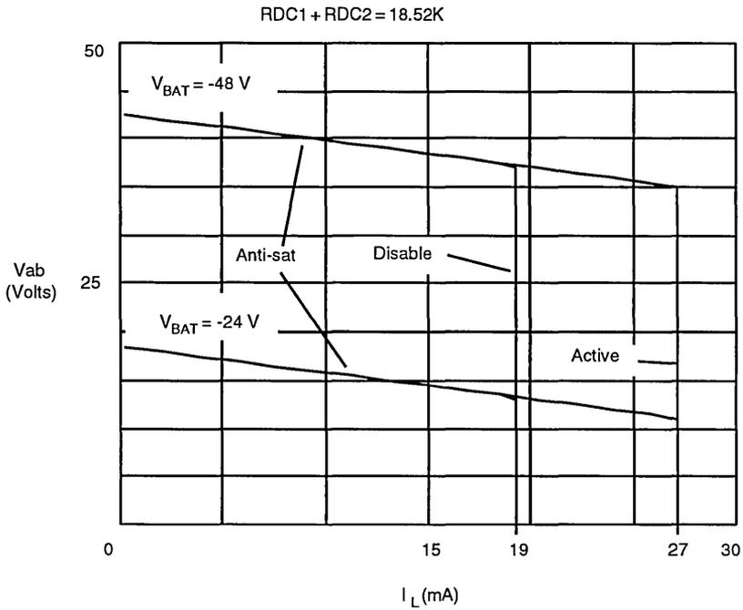
In anti-sat region:  $V_L = V_{BAT} - 5.7 - \frac{R_{DC}}{70} \cdot I_L$
