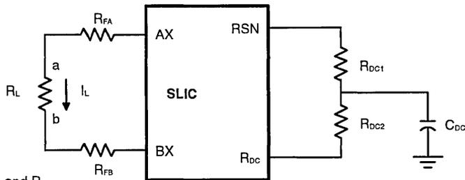
Current programmed by  $R_{DC1}$  and  $R_{DC2}$ .
