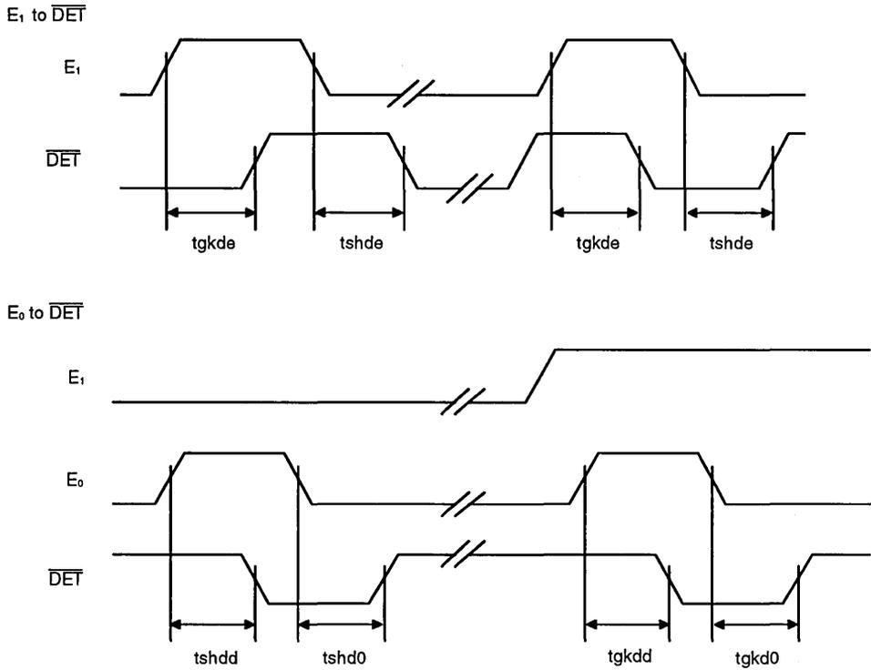
Note: All delays measured at 1.4-V level.
