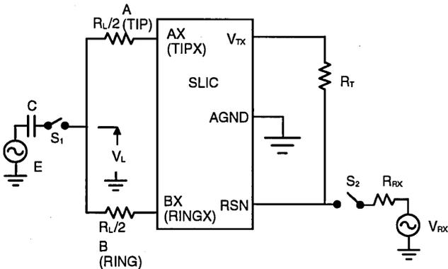
$S_1$  closed,  $S_2$  open and  $1/\omega C \ll R_L$ :
