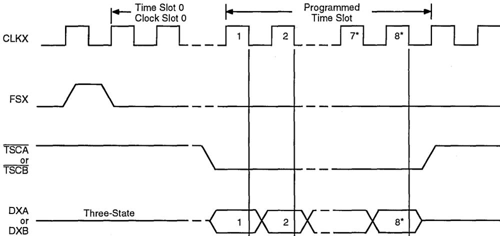
\*For linear code, the 7th and 8th clock cycles correspond to the 15th and 16th clock cycles.
