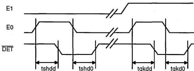
Note: All delays measured at 1.4-V level.
