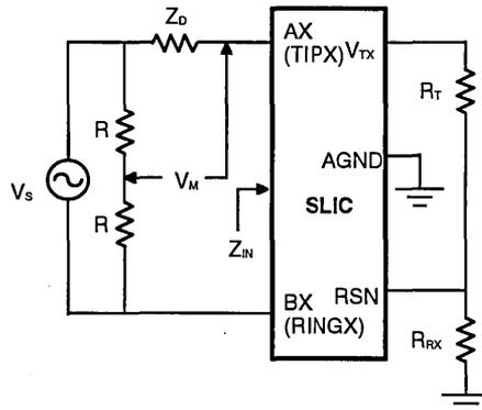
$Z_D$ : The desired impedance (e.g., the characteristic impedance of the line).
