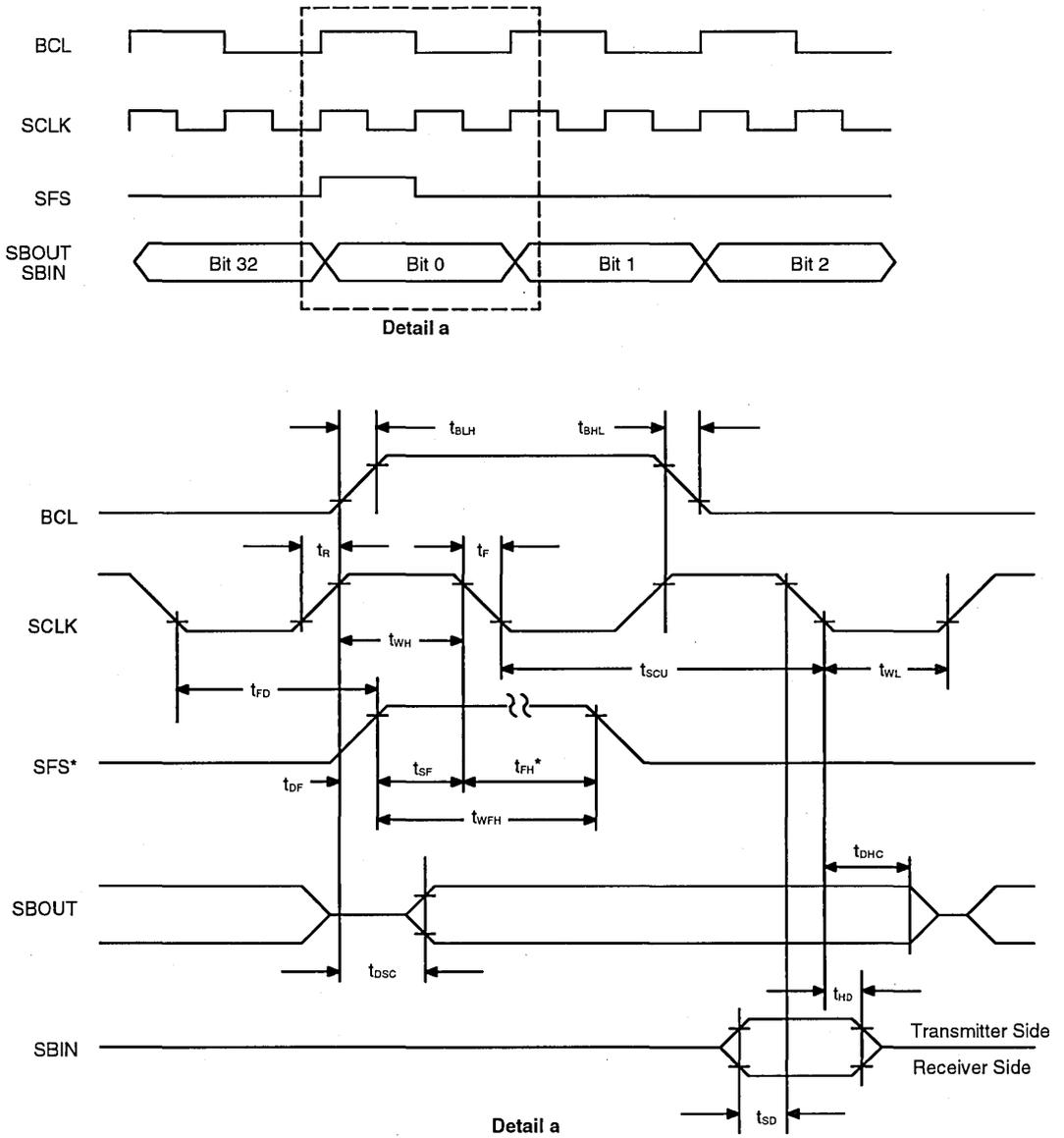
\* In Master Mode, SFS is 16 SCLK cycles + set-up time + hold time in length
