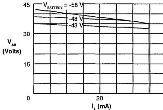
Figure 1a. Load Line (Typical)
