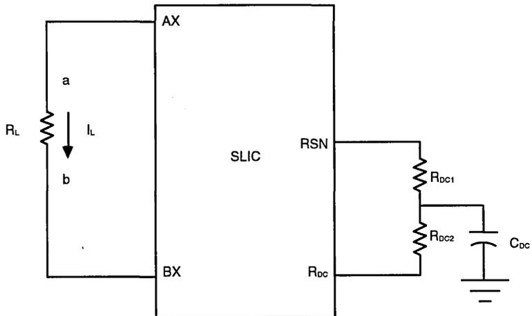
Feed resistance programmed by  $R_{DC1}$  and  $R_{DC2}$ .
