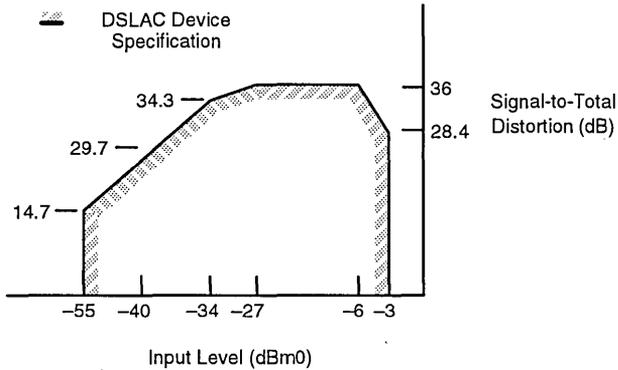
Figure 16. Total Distortion with Noise Input (Receive Path)
