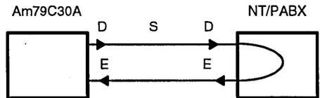
This loopback is provided for maintenance purposes from the TE's perspective. The Am79C30A/32A transmits D-channel bits to the NT where they are looped and transmitted back to the Am79C30A/32A in the E Channel. The operation is normal except differences between the D and E Channels do not halt the transmission.
