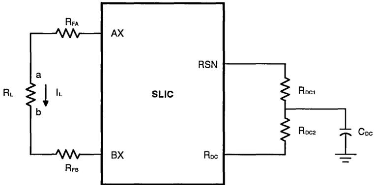
Feed Resistance programmed by  $R_{DC1}$  and  $R_{DC2}$ .
