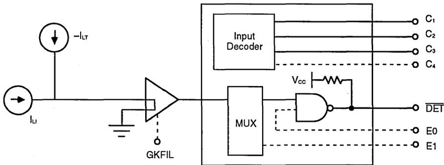
**Figure 7. Ground-Key Detector**
