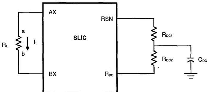
Feed Current programmed by  $R_{DC1}$  and  $R_{DC2}$ .
