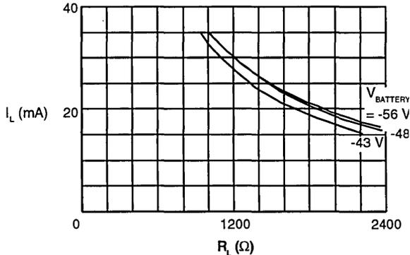
Figure 1b. Feed Characteristics (Typical)
