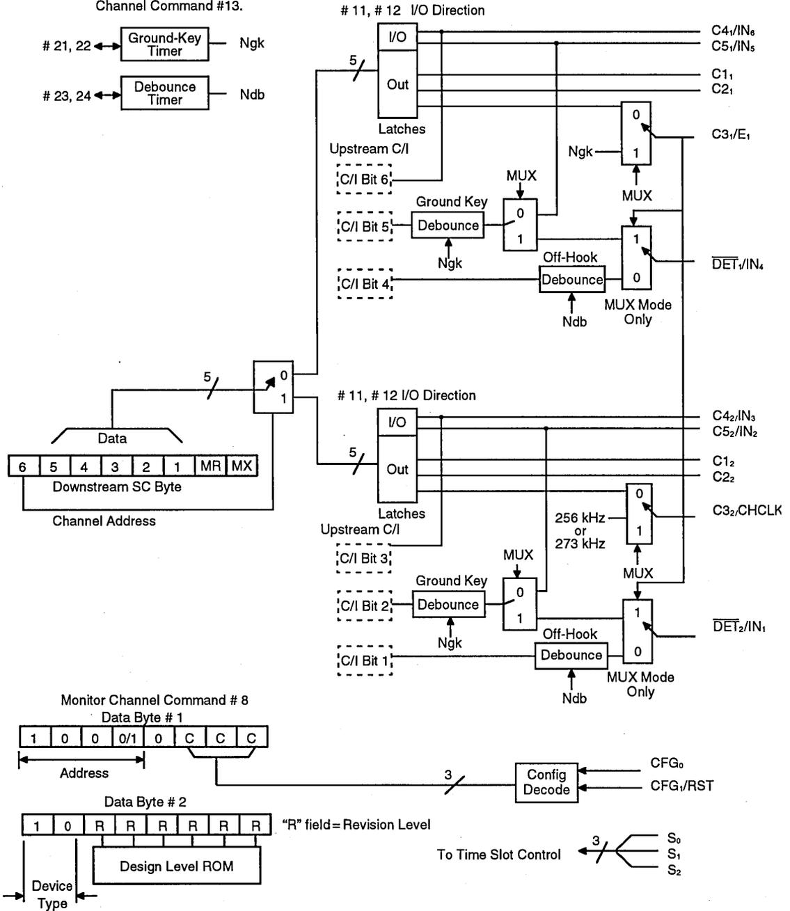
Figure 11. SLIC I/O Architecture
