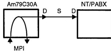
This local loopback is provided for local testing. Data on the incoming D Channel is ignored. The data from the microprocessor is processed by the DLC and then looped back to the microprocessor in addition to being output to the S Interface.
