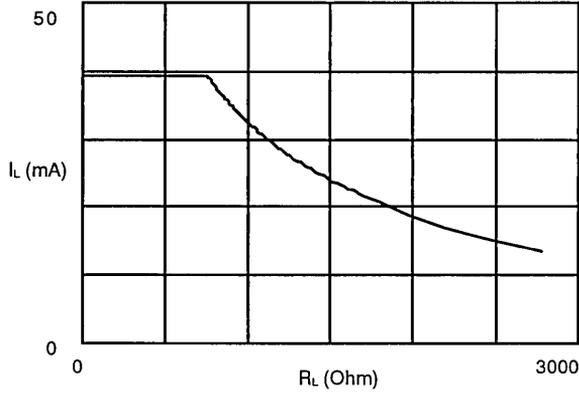
Load Current versus Load Resistance—Am79530/Am79531/Am79534/Am79535
