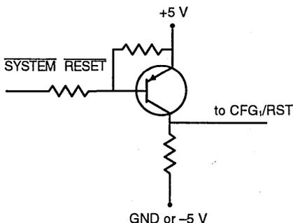
Figure 12. Circuit Schematic for the  $CFG_1$ , RST Input
