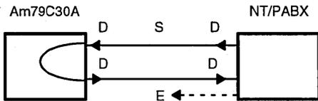
This remote loopback is provided for maintenance purposes from the NT's perspective. The NT transmits D-channel bits to the Am79C30A/32A where they are internally looped (with the Data Link Controller) and transmitted back to the NT. The incoming D-channel data can be accessed by the microprocessor; however, the microprocessor cannot send data on the outgoing D Channel.
