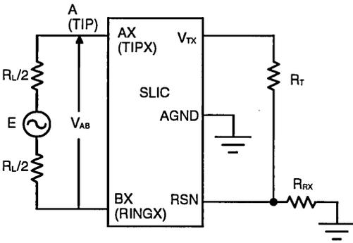
$$I_{L2-4} = -20 \log (V_{TX} / V_{AB})$$
