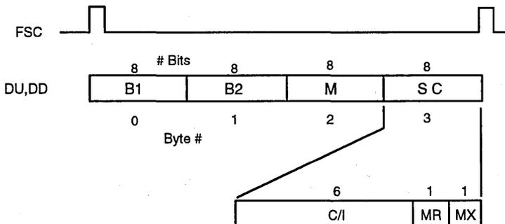
Figure 3. IOM 2 Time Slot Structure (256 kb/s)
