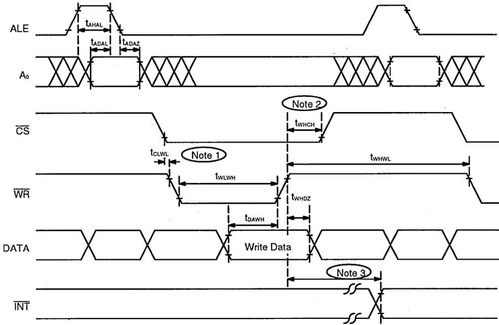
Figure 8. Microprocessor Write Timing
