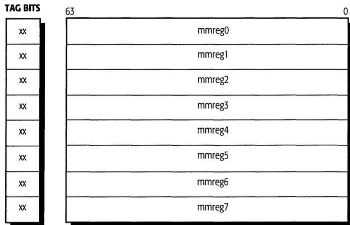
Aliasing the MMX registers onto the floating-point stack registers provides a safe way to introduce this new technology. Instead of needing to modify operating systems, new MMX applications can be supported through device drivers, MMX libraries, or DLL files. See the *Programming Considerations* section of this document for more information.
