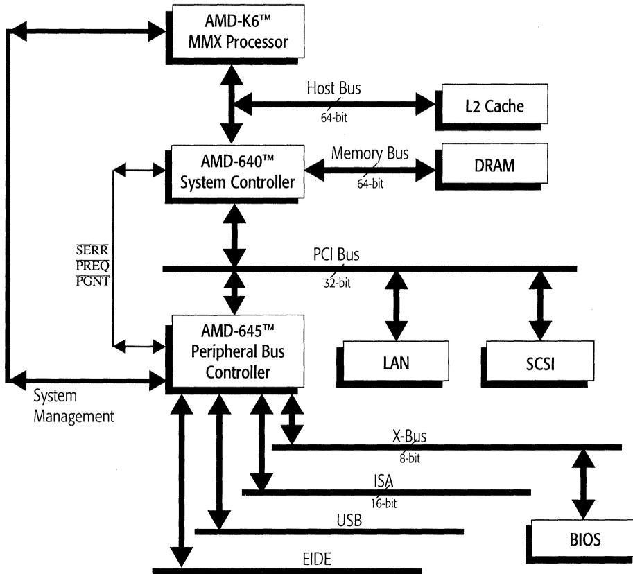
Figure 1-1. AMD-640 Chipset System Block Diagram
