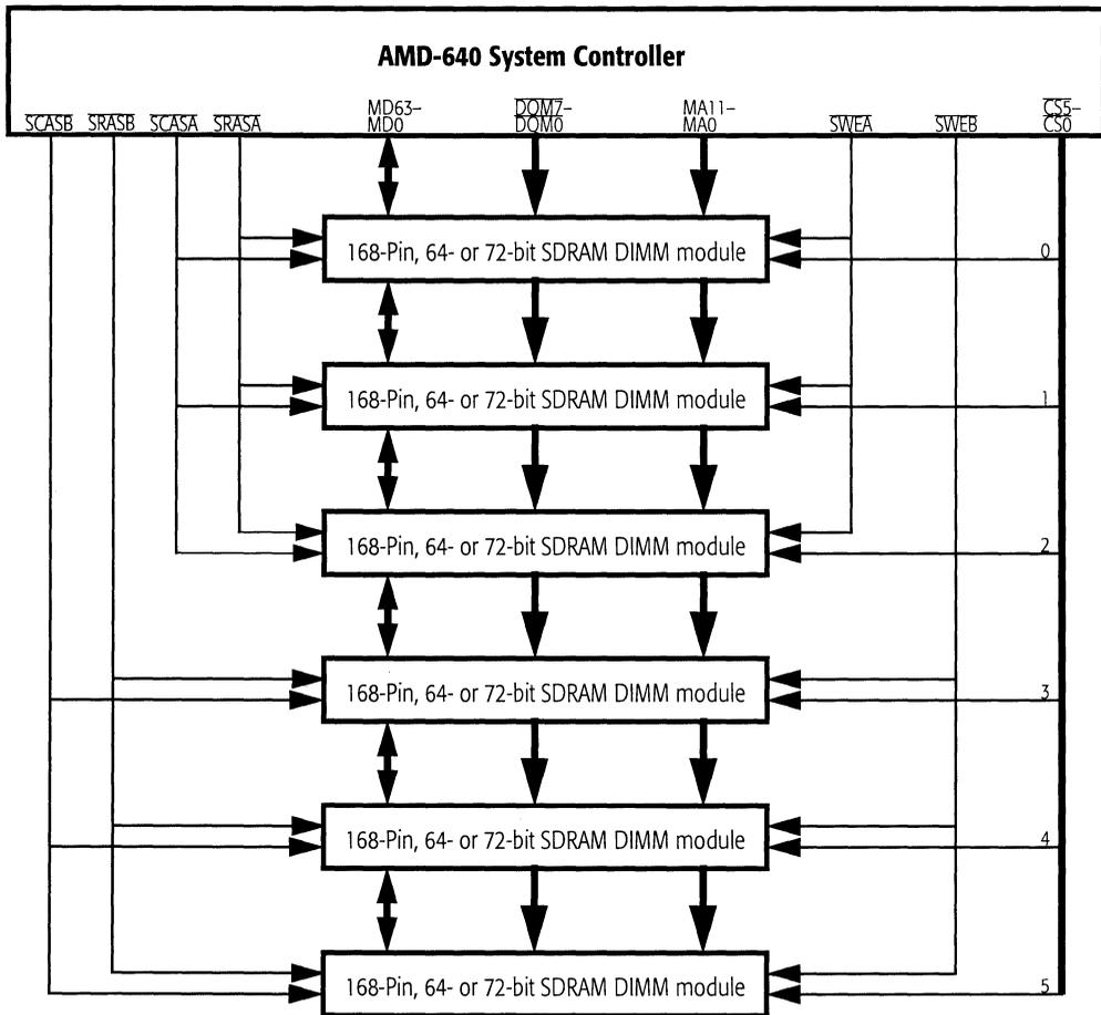
**Figure 5-6. SDRAM Interface Example**
