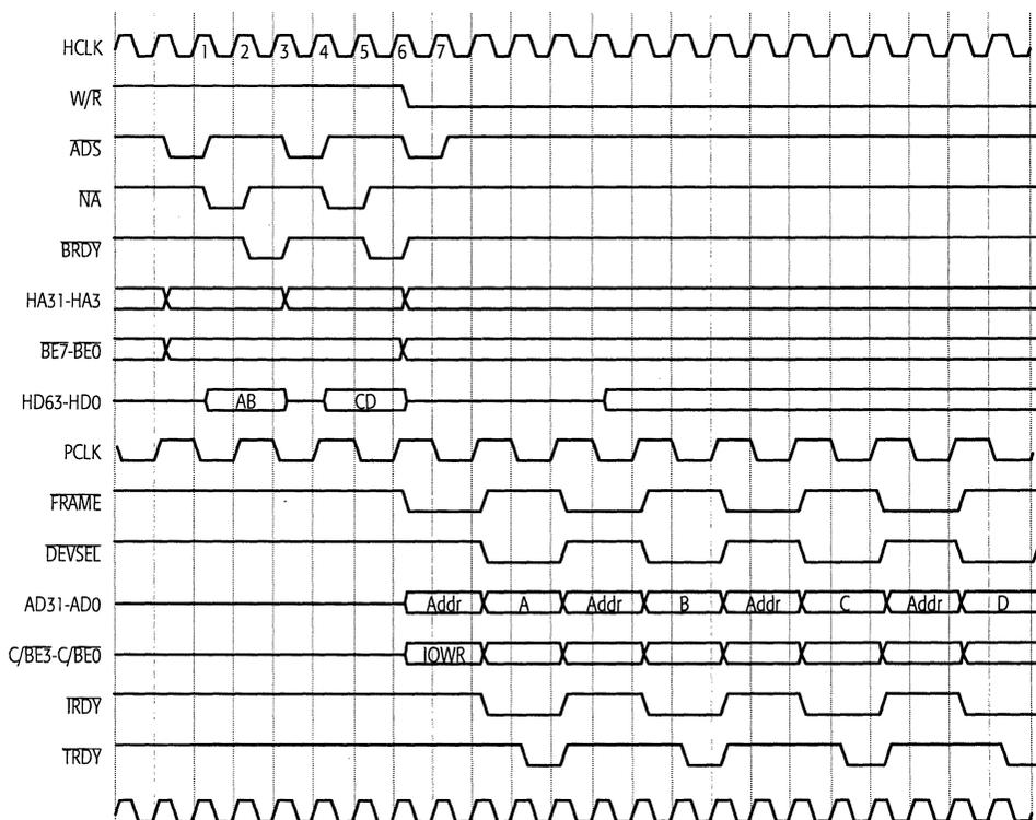
**Figure 5-23. Processor Write to PCI Target**
