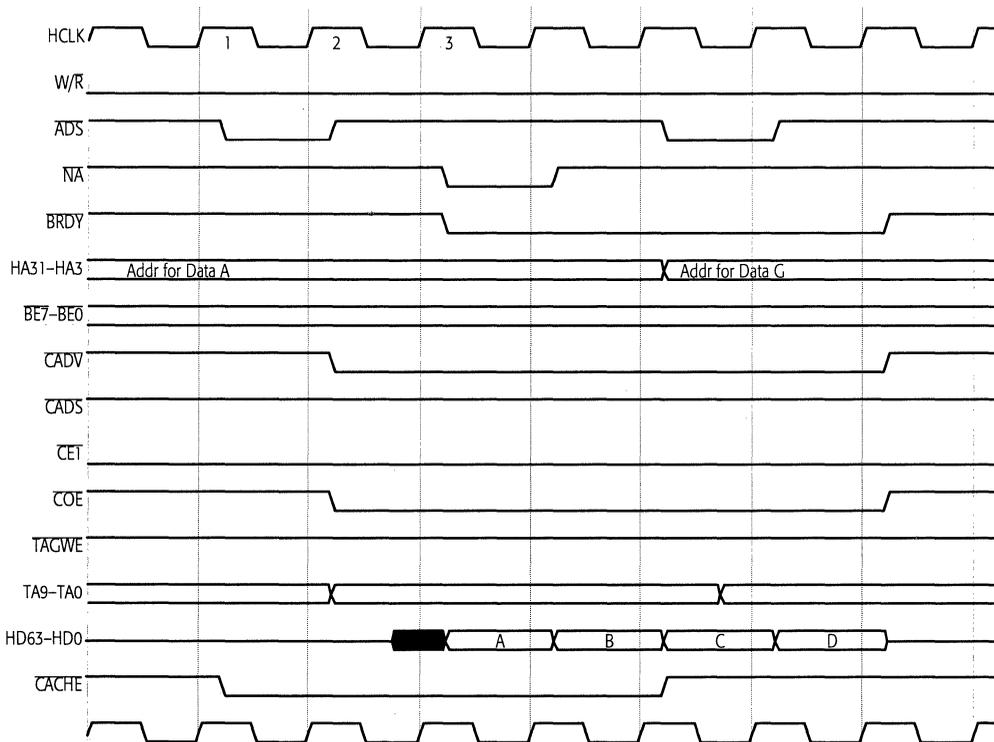
Figure 5-12. Pipelined Burst Read Cycle
