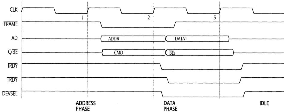
Figure 5-18. PCI Write
