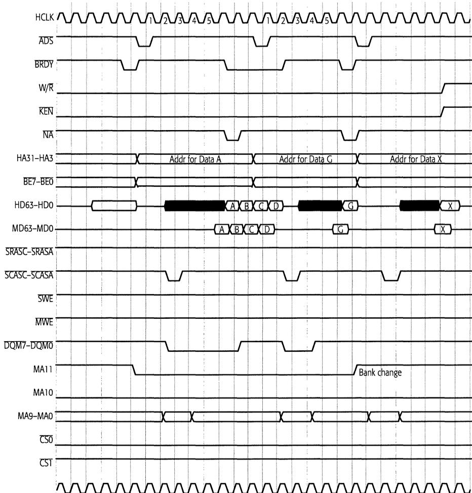
Figure 5-10. SDRAM Burst Read Cycle
