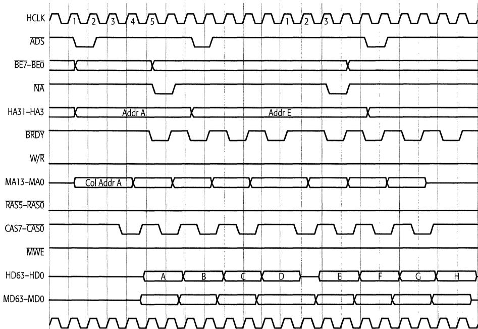
Figure 5-8. Pipelined EDO Read (5-2-2-2, 3-2-2-2)
