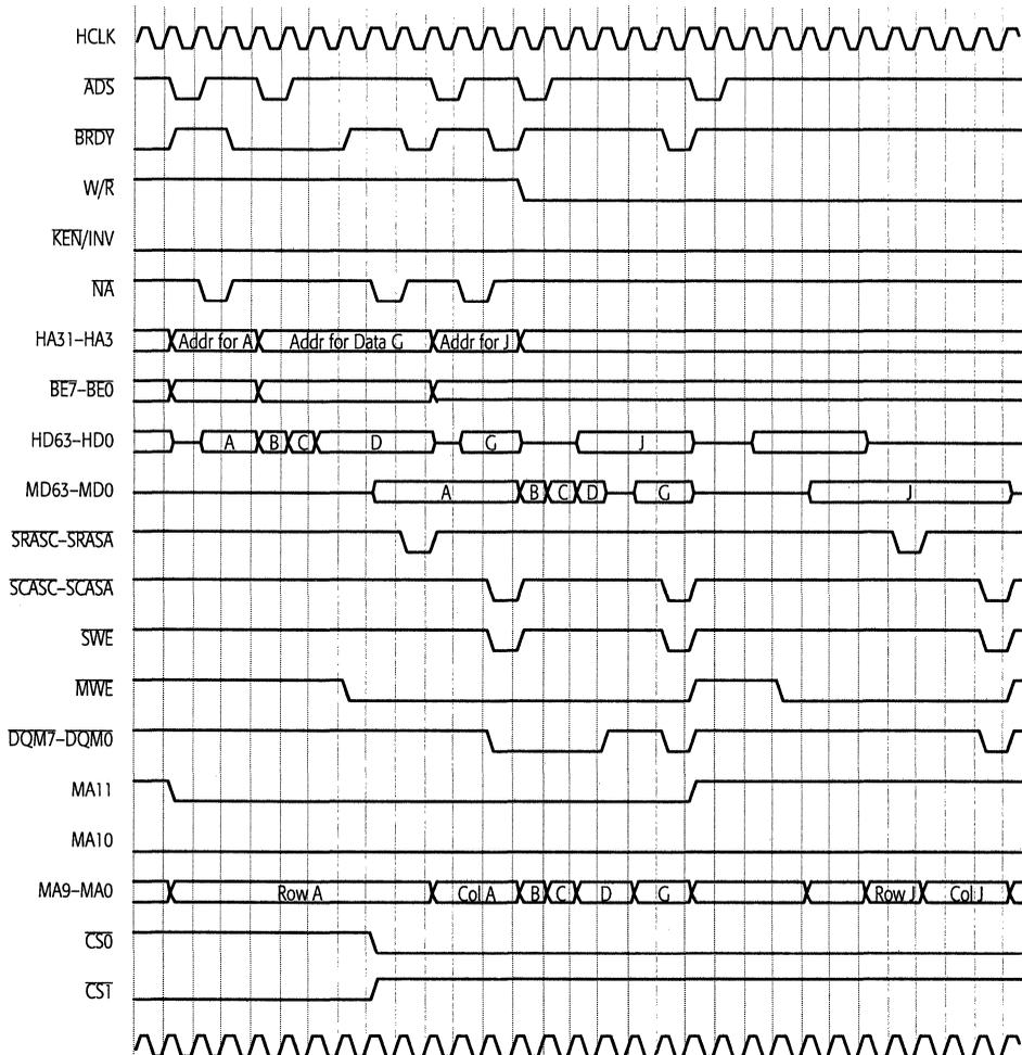
Figure 5-11. SDRAM Write Cycle
