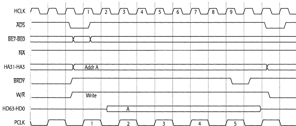
Figure 5-20. Configuration Write
