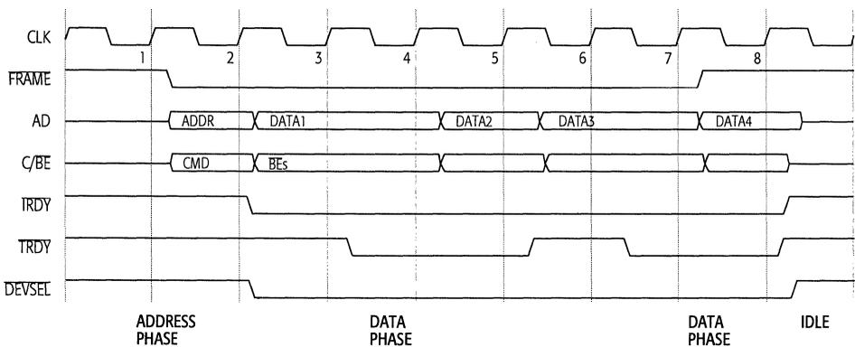
Figure 5-19. PCI Burst Write
