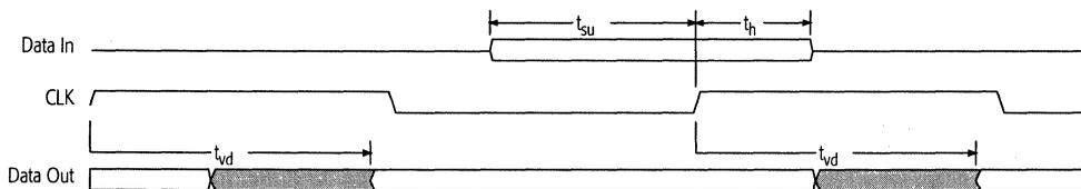
Figure 9-2. Setup, Hold, and Valid Delay Timing Diagram
