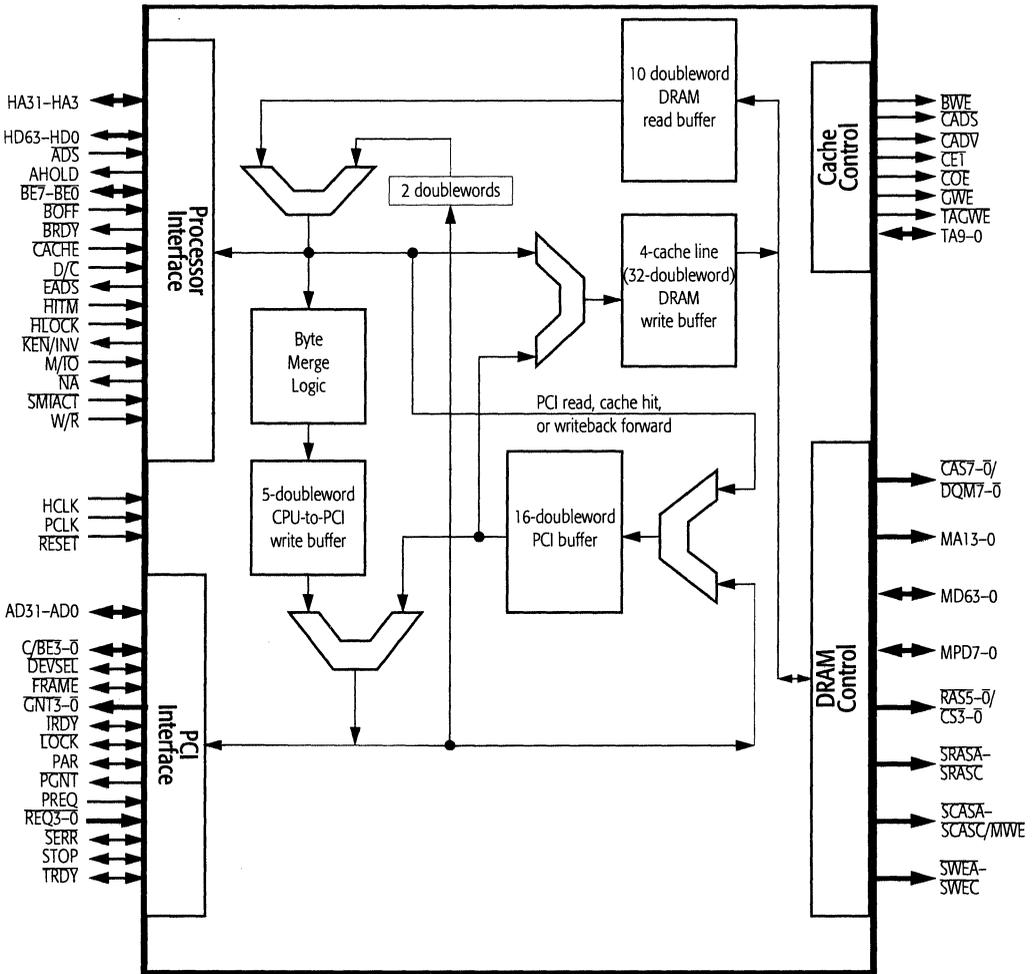
Figure 2-1. AMD-640 System Controller Block Diagram
