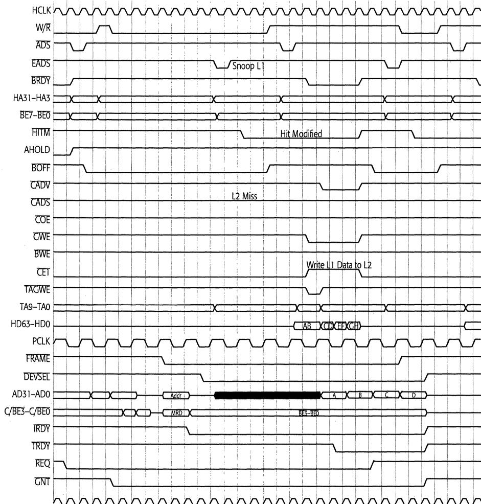
**Figure 5-27. PCI Bus Initiator Read: Modified L1 Hit**
