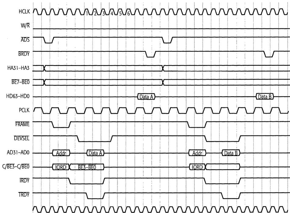
**Figure 5-22. Processor Read from PCI Target**
