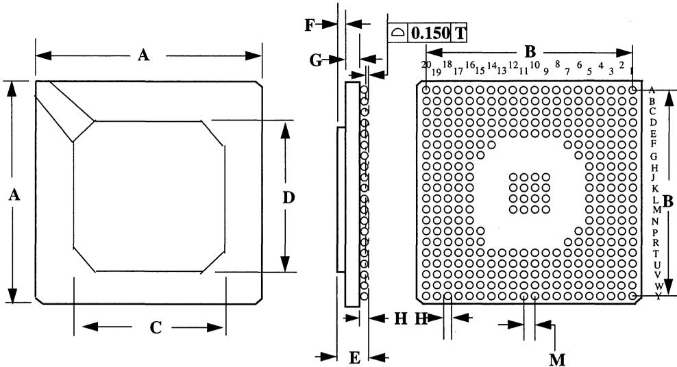
Figure 12-1. 328-Pin BGA Package Preliminary Specification
