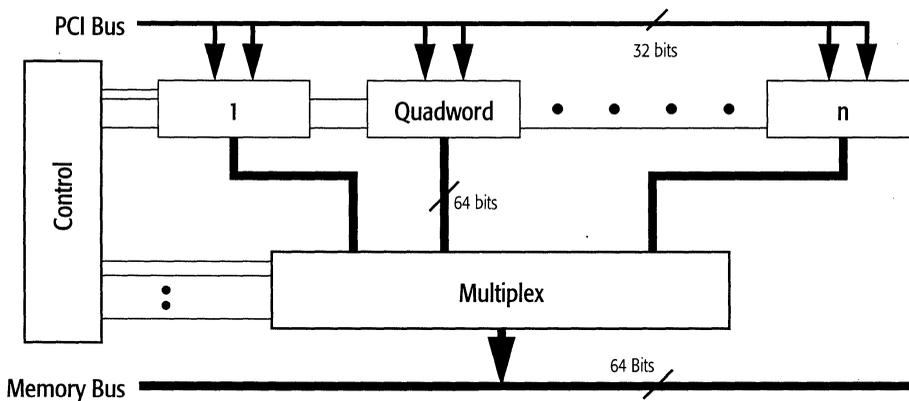
**Figure 2-3. PCI-to-Memory Buffer**
