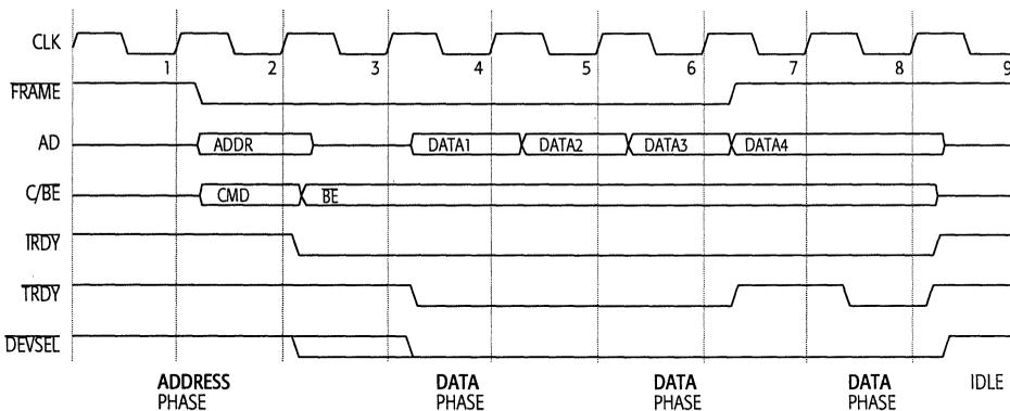
**Figure 5-17. PCI Burst Read Operation**
