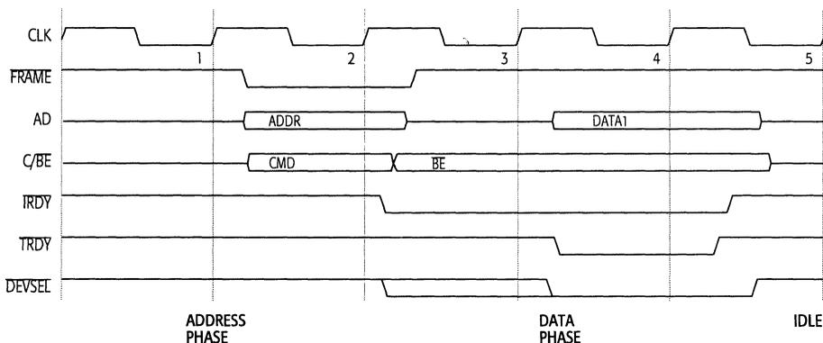
**Figure 5-16. Basic PCI Read Operation**
