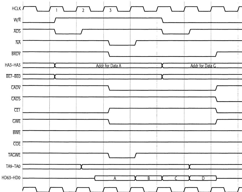
Figure 5-13. Pipelined Burst Write Cycle
