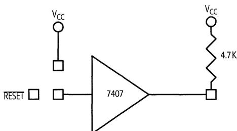
**Figure 7-1. Strap Option Circuit**
