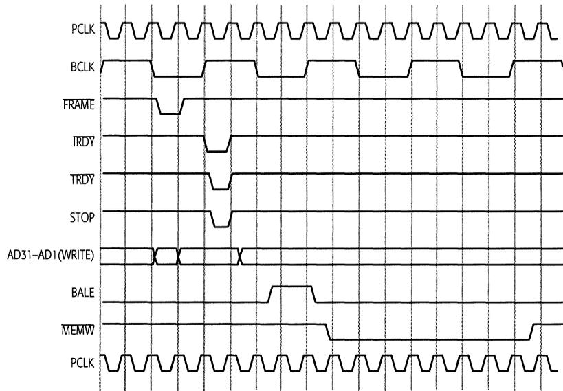
**Figure 5-4. Posted PCI-to-Memory Write**
