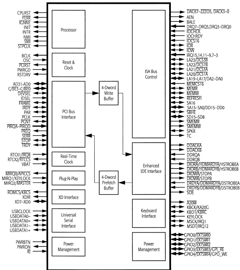
Figure 2-1. AMD-645 Peripheral Bus Controller Block Diagram
