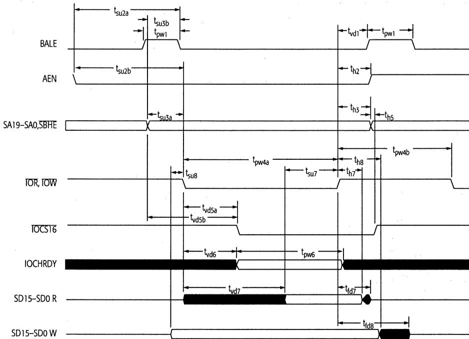
Figure 9-5. ISA 16-Bit Slave Interface Timing
