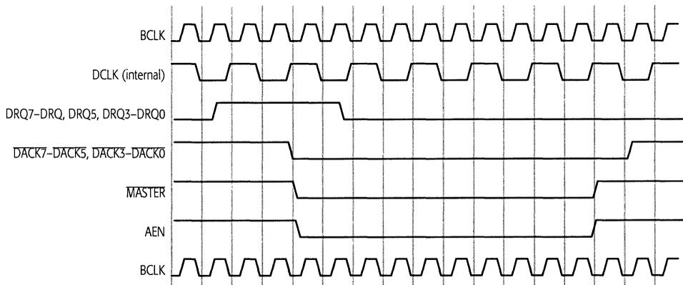
**Figure 5-15. ISA Bus Master Arbitration Timing**
