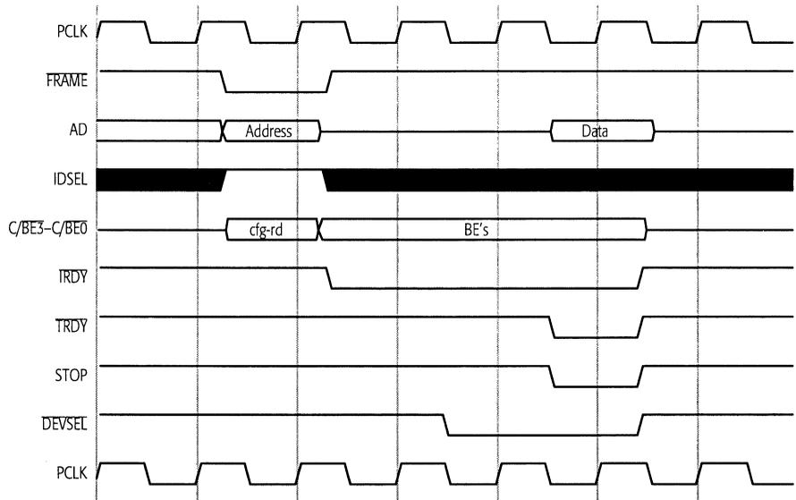
**Figure 5-11. Configuration Read Cycle**
