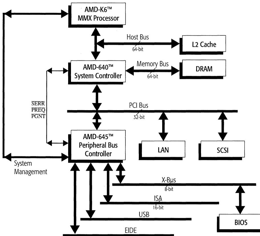
Figure 1-1. AMD-640 Chipset System Block Diagram
