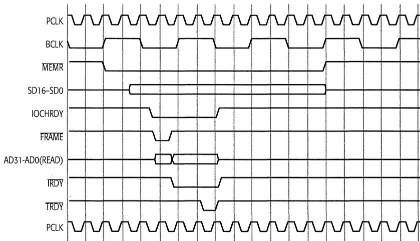
**Figure 5-17. ISA Bus Master-to-PCI Memory (Memory Write)**
