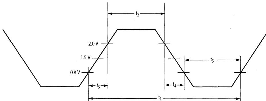
**Figure 9-1. PCLK Waveform**
