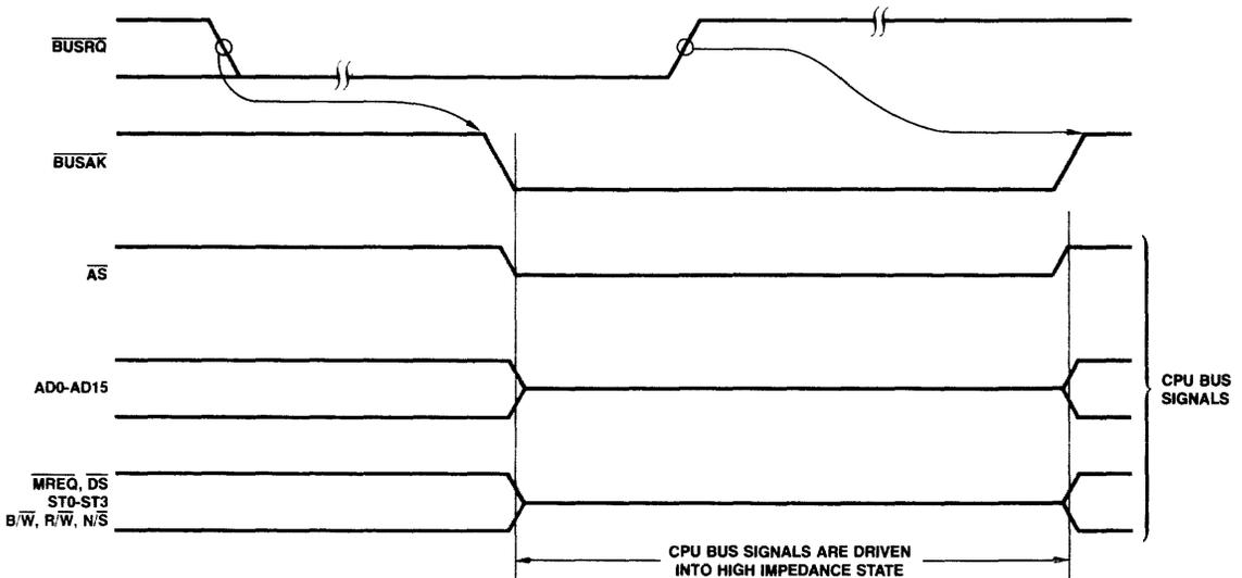
Figure 3-10. Bus Request/Acknowledge Timing.
