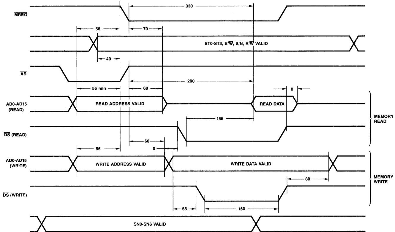
Figure 2-2. Memory Transaction Timing.
