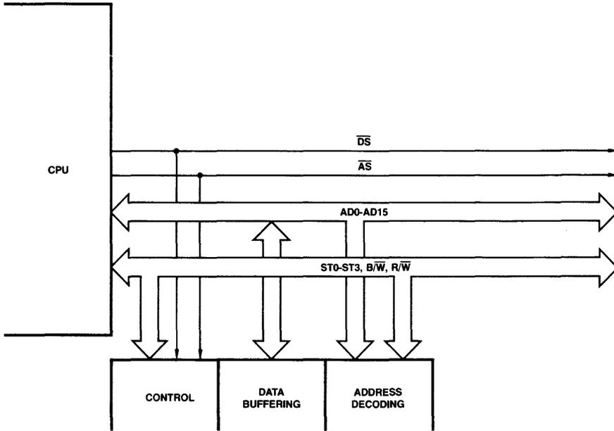
Figure 3-1. Programmed I/O Interface.
