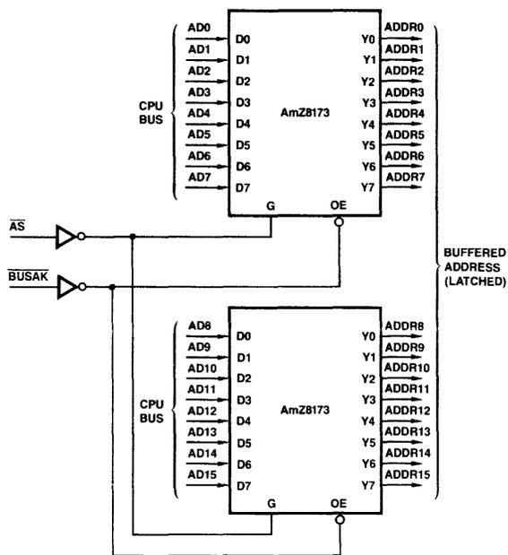
Figure 1-6. CPU Address Latching.
