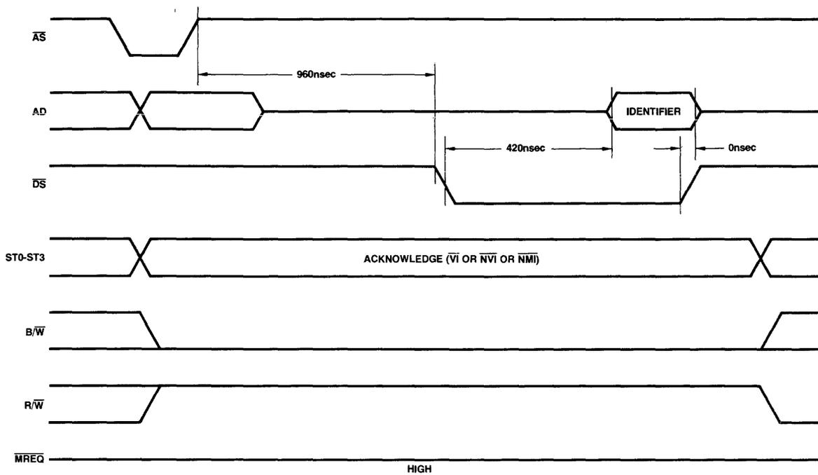
Figure 3-7. Interrupt Acknowledge Cycle.
