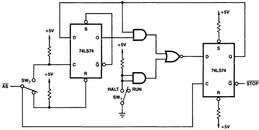
Figure 1-7. CPU Single Step Circuit.
