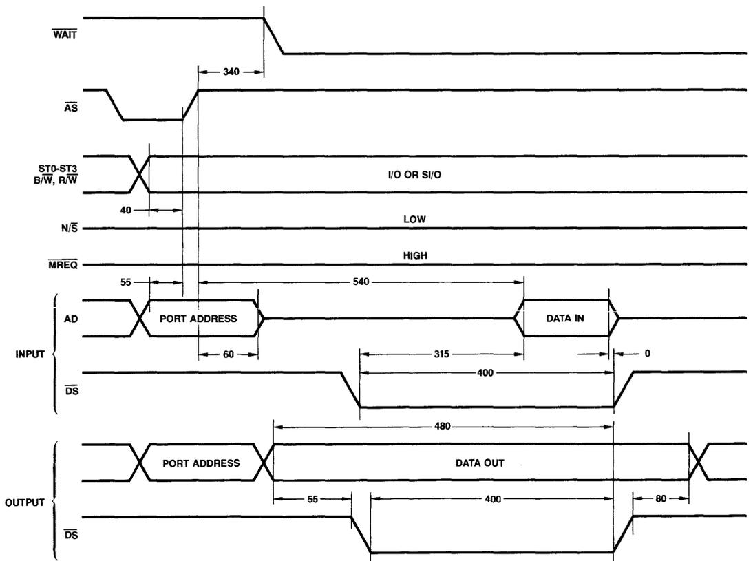
Figure 3-5. Programmed I/O Timing.
