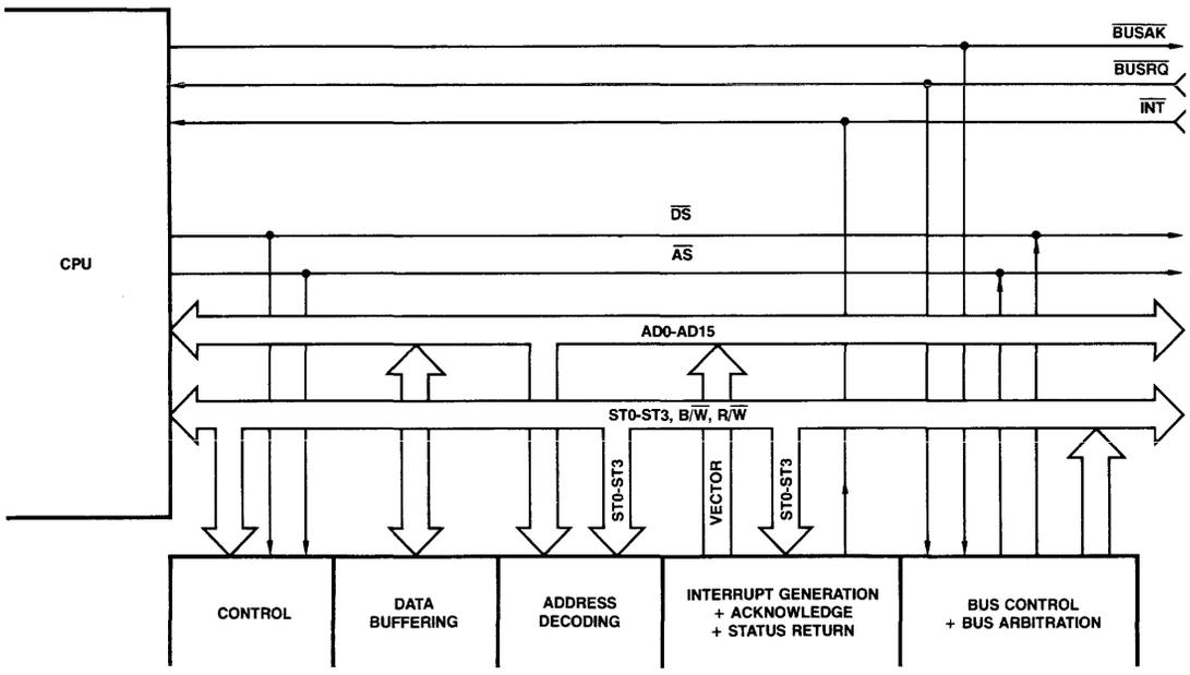
Figure 3-3. Programmed I/O and Interrupts and DMA.
