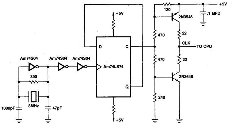
Figure 1-2. CPU Clock Generation.
