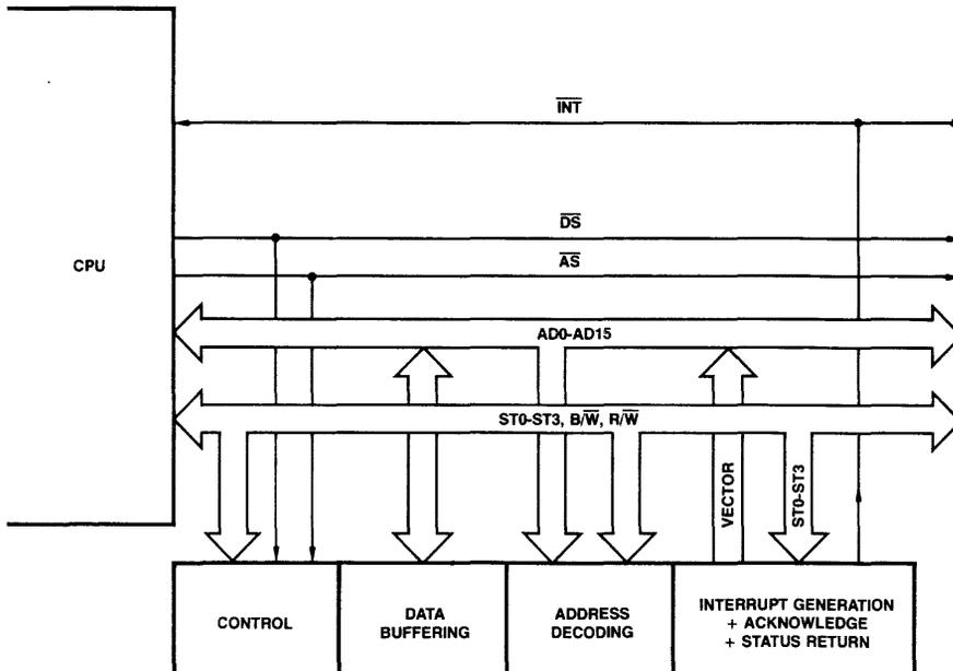
Figure 3-2. Programmed I/O and Interrupts.
