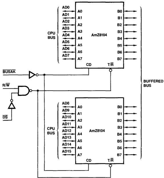
Figure 1-4. Bidirectional CPU Buffering.
