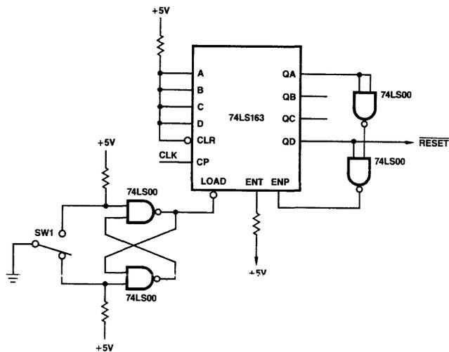
Figure 1-3. CPU Initialization Circuit.
