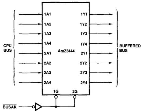
Figure 1-5. CPU Unidirectional Buffering.
