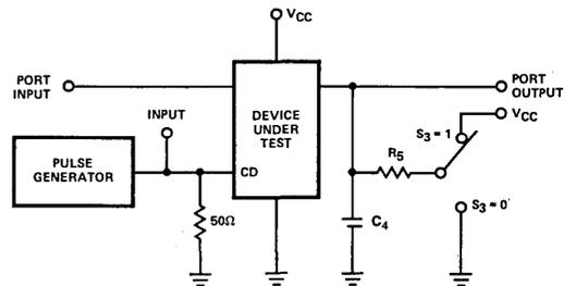
Note:  $C_4$  includes test fixture capacitance.
