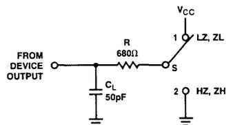
Figure 2. Three-State Enable/Disable.
