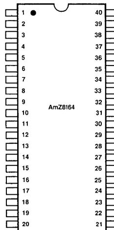
Note: Pin 1 is marked for orientation.
