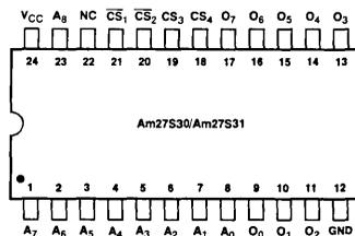
Note: Pin 1 is marked for orientation.
