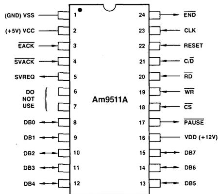
Pin 1 is marked for orientation.
