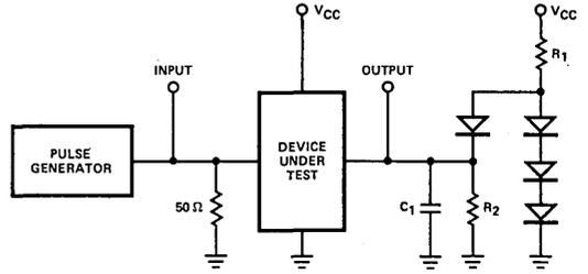
Note:  $C_1$  includes test fixture capacitance.
