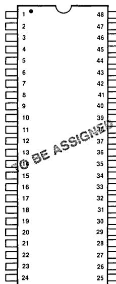
Note: Pin 1 is marked for orientation.
