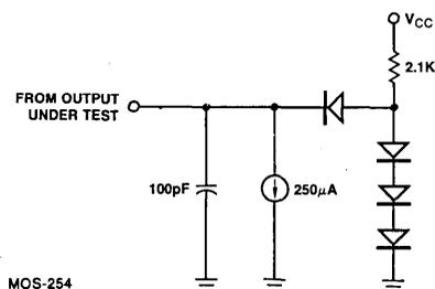
All AC parameters assume a load capacitance of 100pF max, except for parameter 6, T<sub>dC</sub>(SNv) (50pF max). Timing references between two output signals assume a load difference of 50pF max.
