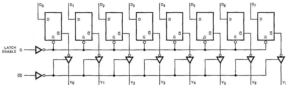
Inputs  $D_0$  through  $D_7$  are inverted on the AmZ8133.
