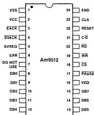
Note: Pin 1 is marked for orientation.
