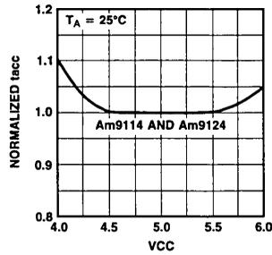
Typical C Load Versus Normalized tacc Characteristics
