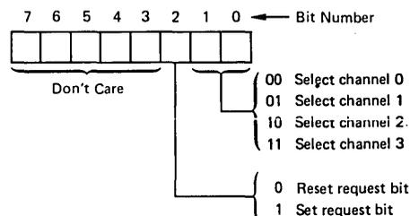
Software requests will be serviced only if the channel is in Block mode. When initiating a memory-to-memory transfer, the software request for channel 0 should be set.
