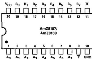
Note: Pin 1 is marked for orientation.
