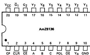
Note: Pin 1 is marked for orientation.
