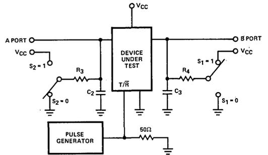
Note:  $C_2$  and  $C_3$  include test fixture capacitance.
