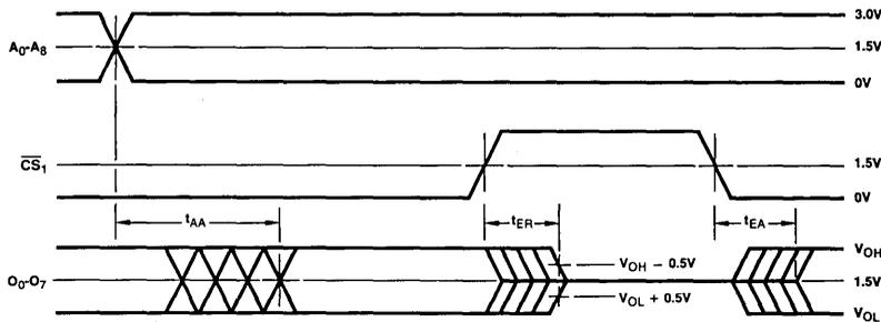
Note: Level on output while CS is HIGH is determined externally.
