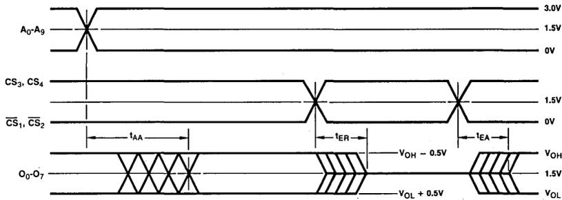
Note: Level on output while chip is disabled is determined externally.
