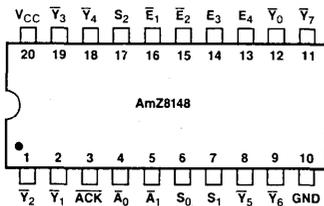
Note: Pin 1 is marked for orientation.
