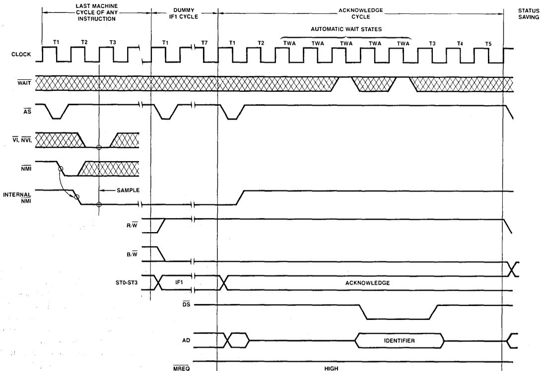
Figure 6. CPU Interrupt and Segment Trap Request Acknowledge Timing.
