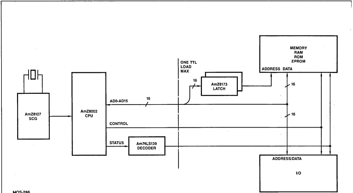
Figure 9. Simple AmZ8002 System Requires Few MSI Circuits, but has Limited Drive Capability.
