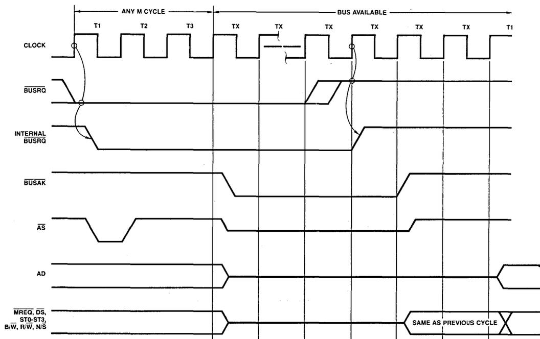
Figure 9. Bus Request/Acknowledge Cycle.
