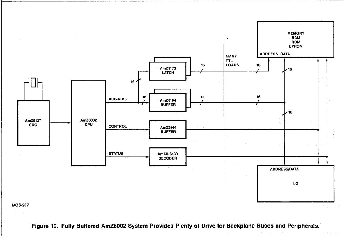
Figure 10. Fully Buffered AmZ8002 System Provides Plenty of Drive for Backplane Buses and Peripherals.
