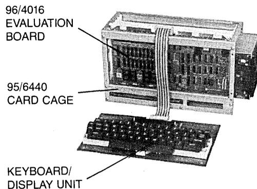
Photo showing use of the AMC 95/6440 Card Cage to house and power the 96/4016 Evaluation Board. Optional Keyboard/Display Unit shown above (or standard CRT Terminal) attaches via cable to edge-card connector. This arrangement provides both convenience and expansion capabilities for specific project and product development.
