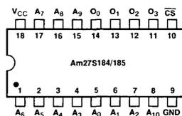
Note 1: Pin 1 is marked for orientation.
