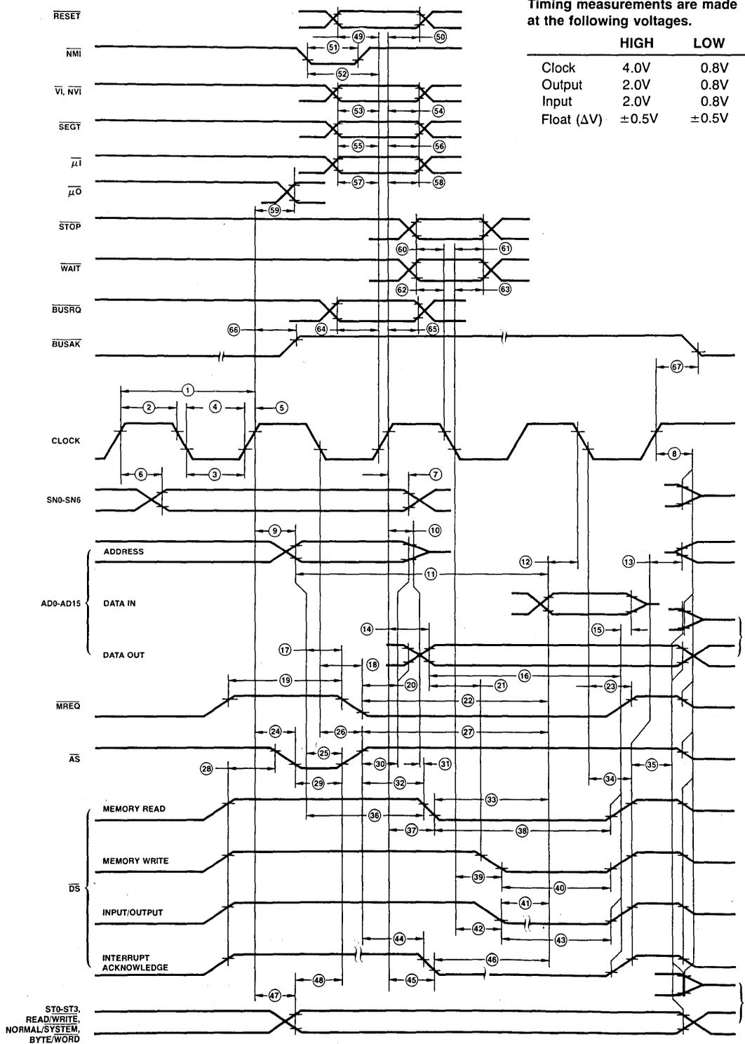
This composite timing diagram does not show actual timing sequences. Refer to this diagram only for the detailed timing relationships of individual edges. Use the preceding illustrations as an explanation of the various timing sequences.
