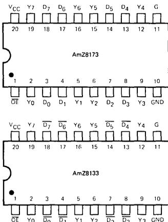
Note: Pin 1 is marked for orientation.
