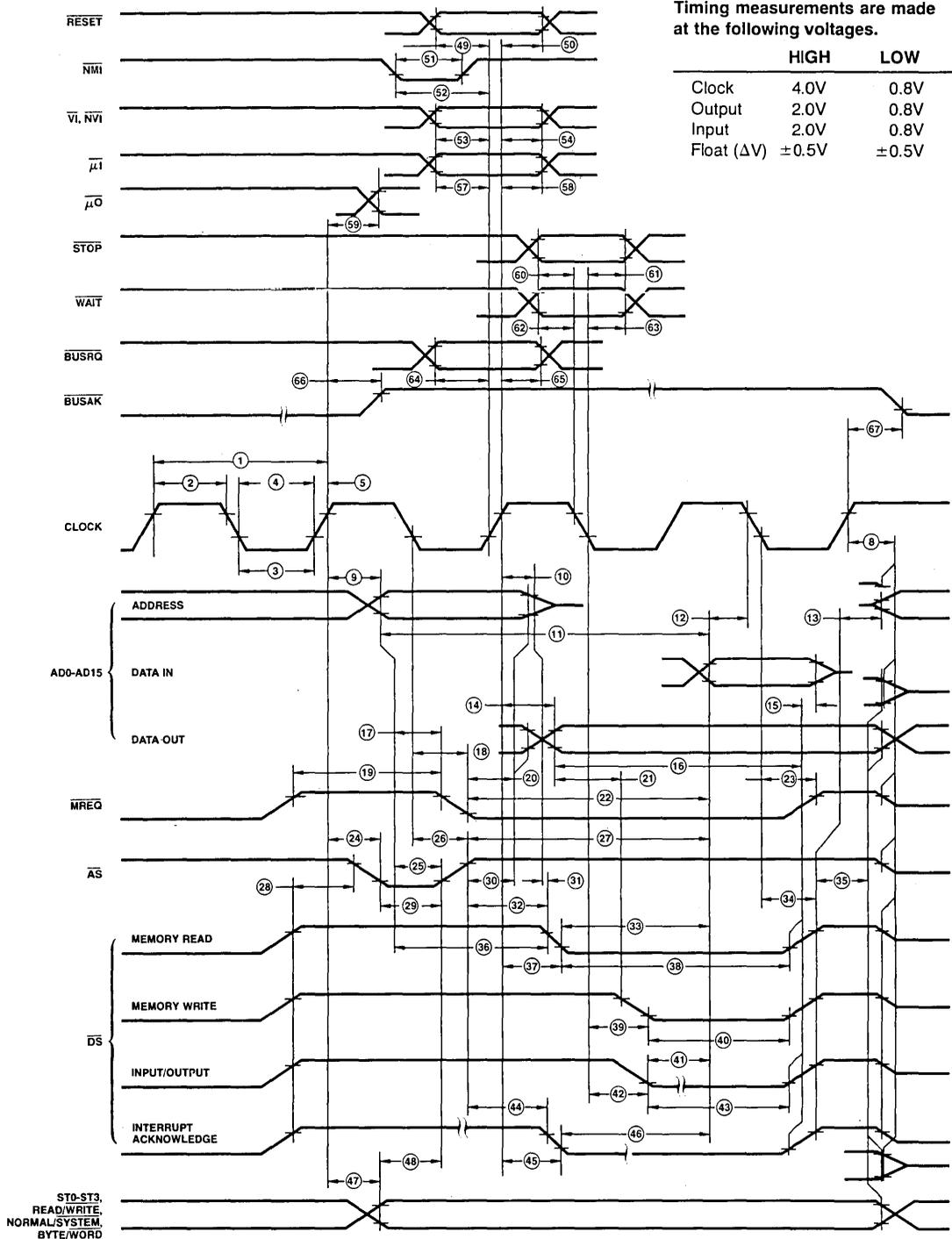
This composite timing diagram does not show actual timing sequences. Refer to this diagram only for the detailed timing relationships of individual edges. Use the preceding illustrations as an explanation of the various timing sequences.
