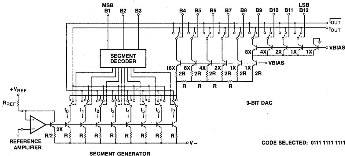
Figure 3. Segmented DAC Functional Diagram Used in Am6012.
