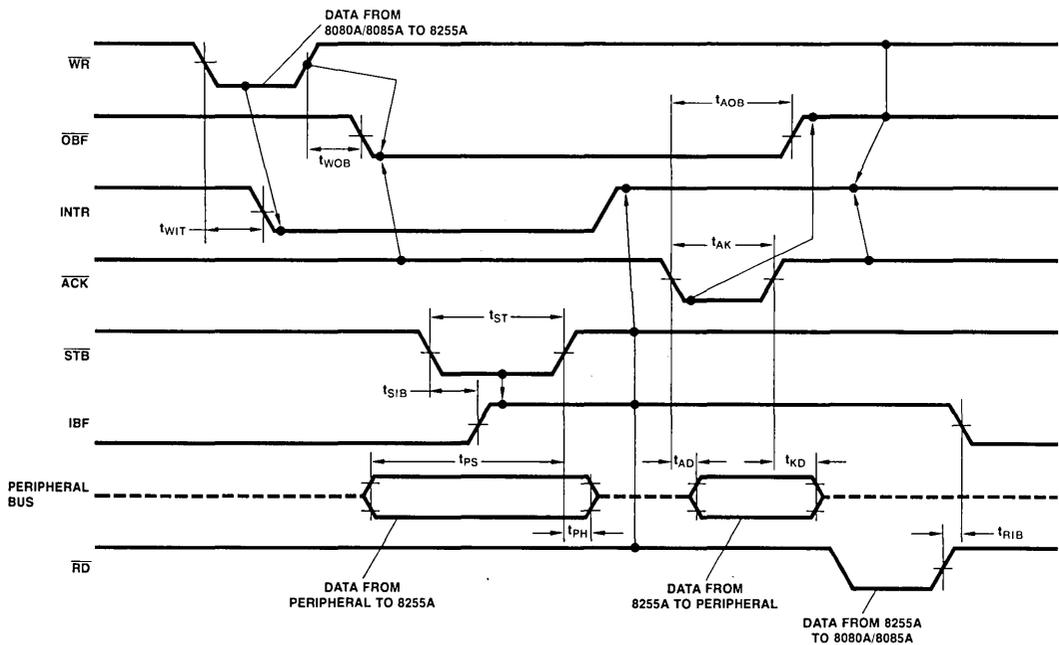
Note: Any sequence where  $\overline{WR}$  occurs before  $\overline{ACK}$  and  $\overline{STB}$  occurs before  $\overline{RD}$  is permissible.
