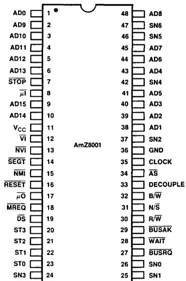
Note: Pin 1 is marked for orientation.
