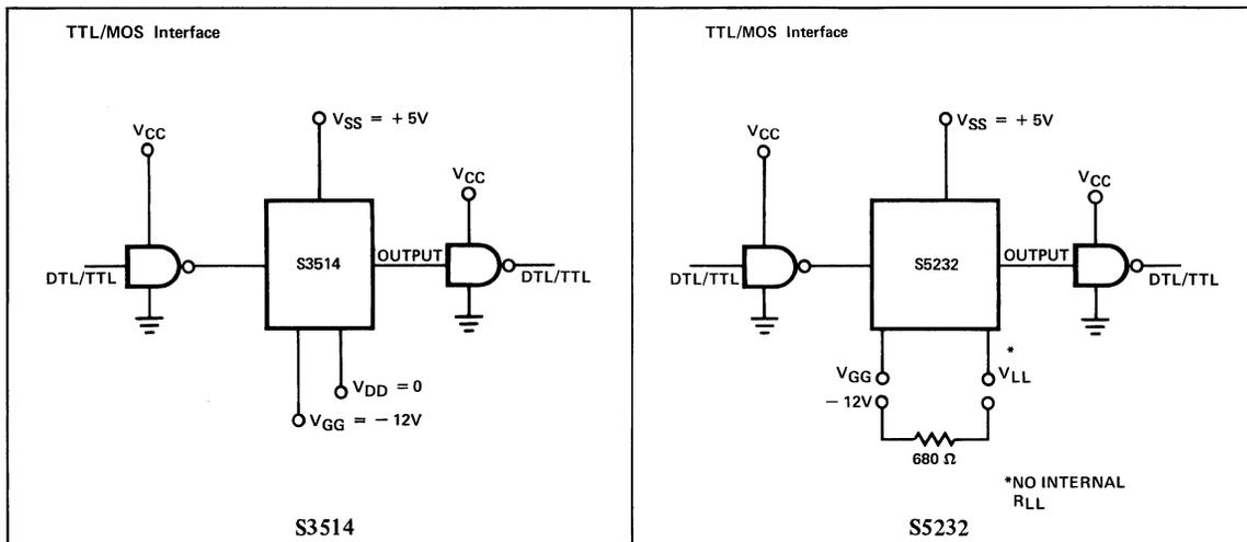
\*For applications where  $V_{GG}$  is connected to  $V_{LL}$ , where low power dissipation is required on outputs and where a constant external resistance is preferred, the internal resistor can be programmed out and an external 680Ω resistor can be connected as shown.
