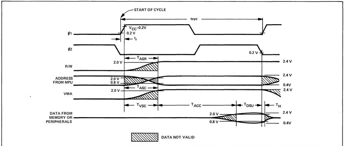
FIGURE 3 – WRITE DATA IN MEMORY OR PERIPHERALS
