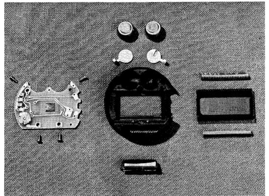
The above photo shows all parts that make up the HMM and CWM watch modules. It demonstrates the dramatic simplification of the second generation CWM (right) over the earlier HMM (left).
