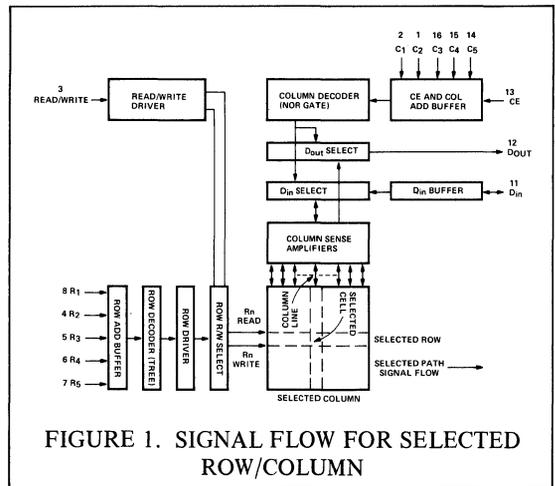
FIGURE 1. SIGNAL FLOW FOR SELECTED ROW/COLUMN
