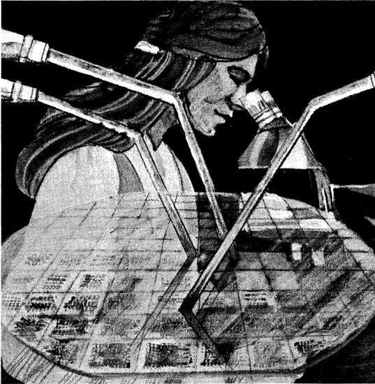
Once Step Two devices are approved, Step Three starts a multifaceted operation. Manufacturing documentation is generated, including test programs; wafer probe cards and program boards for the testing equipment are built; wafer reproducibility runs are made and then evaluated for yield factors. When it's all over, assembled tested devices are delivered to you for your evaluation. There is a charge for Step Three, based upon the complexity of the test program and the number of units delivered.
