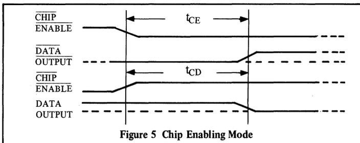
A LOW logic level on the  $\overline{CE}$  enables the chip. Output data becomes valid within  $t_{CE}$  time. Return of the  $\overline{CE}$  input to logic HIGH disables the chip; data remains for  $t_{CD}$  time.
