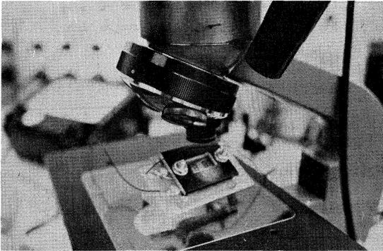
The Viewing Angle is Checked on Display Cells with a Digital Photometer.
