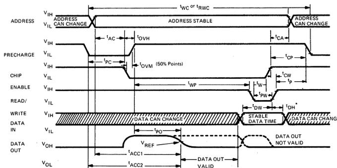
\*  $t_{DW}$  and  $t_{DH}$  are referenced to the rising edge of Chip Enable or Read/Write, whichever occurs first.
