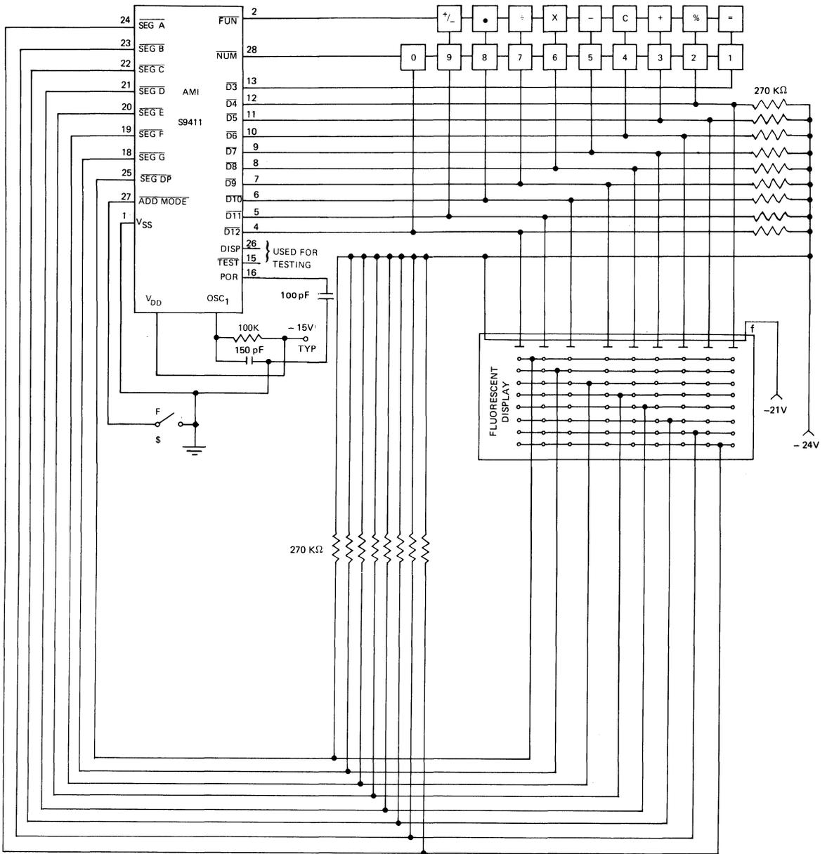
TYPICAL SCHEMATIC DIAGRAM W/FLUORESCENT DISPLAY
