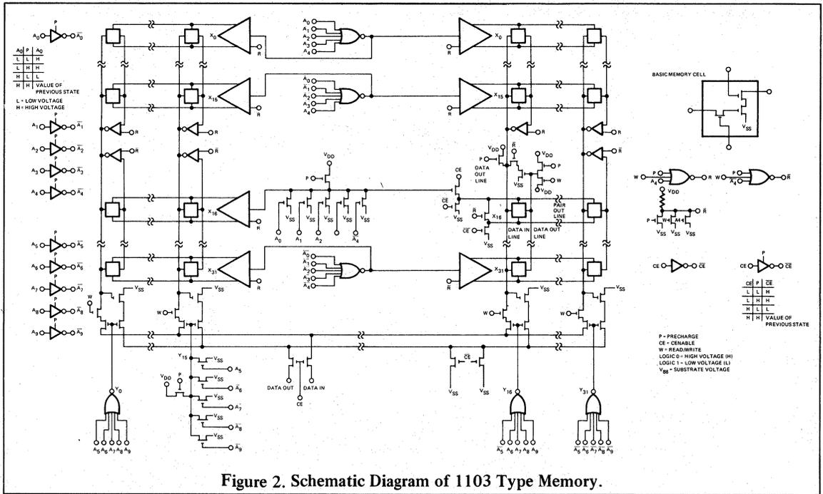
Figure 2. Schematic Diagram of 1103 Type Memory.
