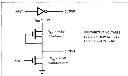
Where  $V_{BS}$  is the substrate-to-source back bias the  $\gamma$  is the *body effect* term (a constant that typically varies from 0.5 to 0.75, depending on the process and the doping concentrations). Thus, the effective  $V_T$  in this example is  $-2 - (0.5\sqrt{5}) \approx -3.1$  volts (using  $\gamma = 0.5$ ).
