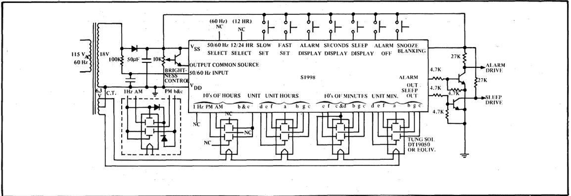
FIGURE 7. TUBE DISPLAY CLOCK
