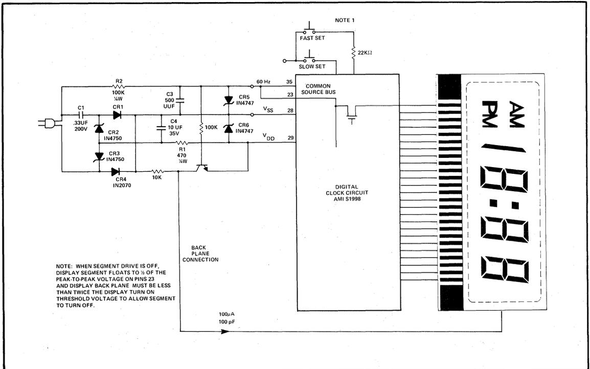
FIGURE 8 LCD DISPLAY CLOCK
