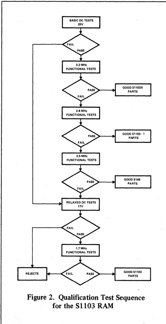
Figure 2. Qualification Test Sequence for the S1103 RAM
