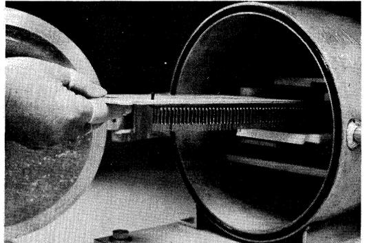
Display Cells Ready for Filling with Liquid Crystal Material.
