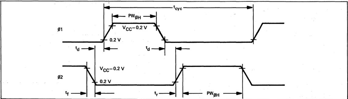
FIGURE 2 – READ DATA FROM MEMORY OR PERIPHERALS
