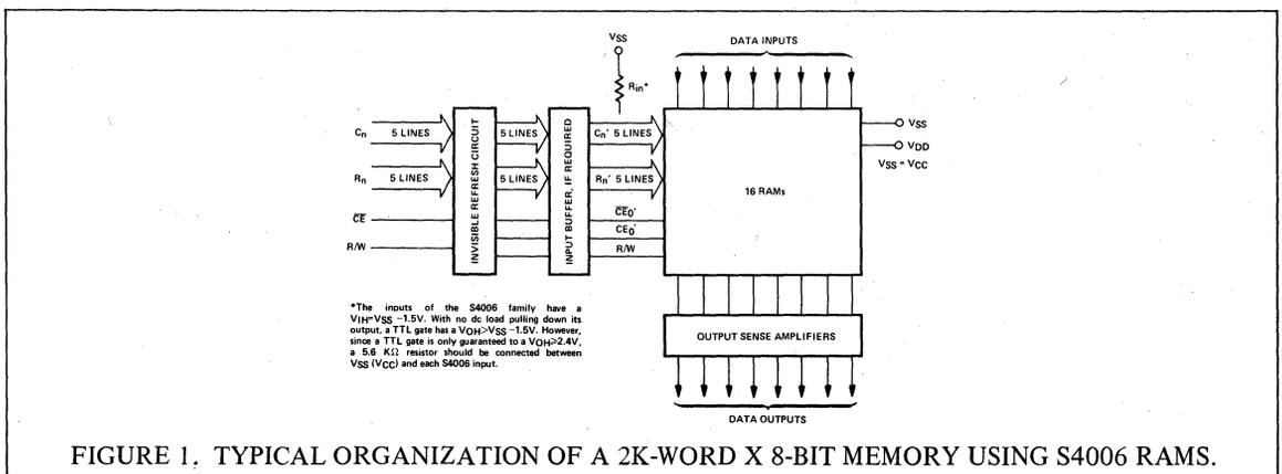
FIGURE 1. TYPICAL ORGANIZATION OF A 2K-WORD X 8-BIT MEMORY USING S4006 RAMS.
