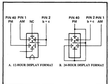
FIGURE 6. WIRING TEN'S-OF-HOURS DIGIT
