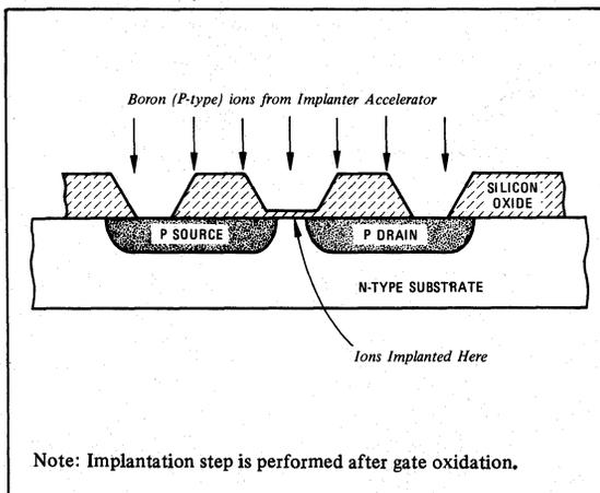
Because of its low  $V_T$ , it offers the designer a choice of using low power supply voltages to conserve power or increase supply voltages to get more driving power and thus increase speed. At low power levels it is more feasible to implement clock generating and gating circuits on the chip. In most circuit designs only a single power supply voltage is required.
