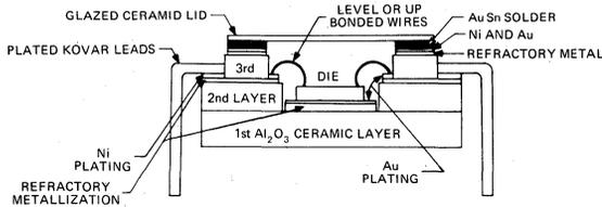
Industry standard high performance, high reliability package, made of three layers of Al<sub>2</sub>O<sub>3</sub> ceramic and nickel-plated refractory metal. The cavity is sealed with a glazed ceramic lid, using a controlled devitrified low temperature glass sealant. Package leads are of Kovar, nickel-plated and solder dipped for socket insertion or soldering.
