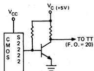
**FIGURE 1 (b) CMOS TO TTL INTERFACE**
