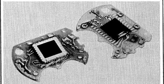
PC Boards Ready for Insertion into Modules.
