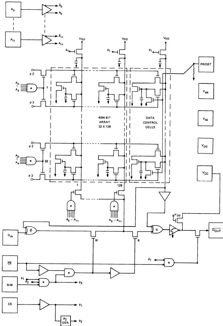
FIGURE 1 – LOGIC DIAGRAM OF 4096-BIT RAM
