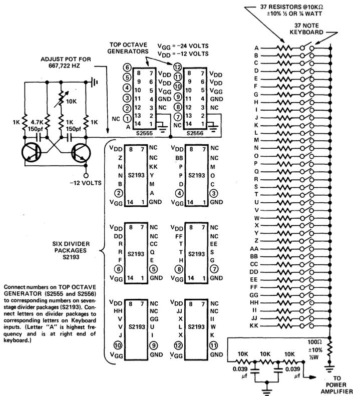
FIGURE 9. SCHEMATIC DIAGRAM FOR SINGLE-VOICE 37-NOTE KEYBOARD ELECTRONIC ORGAN
