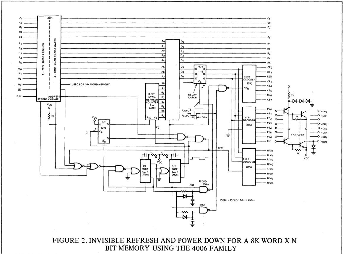
FIGURE 2. INVISIBLE REFRESH AND POWER DOWN FOR A 8K WORD X N BIT MEMORY USING THE 4006 FAMILY
