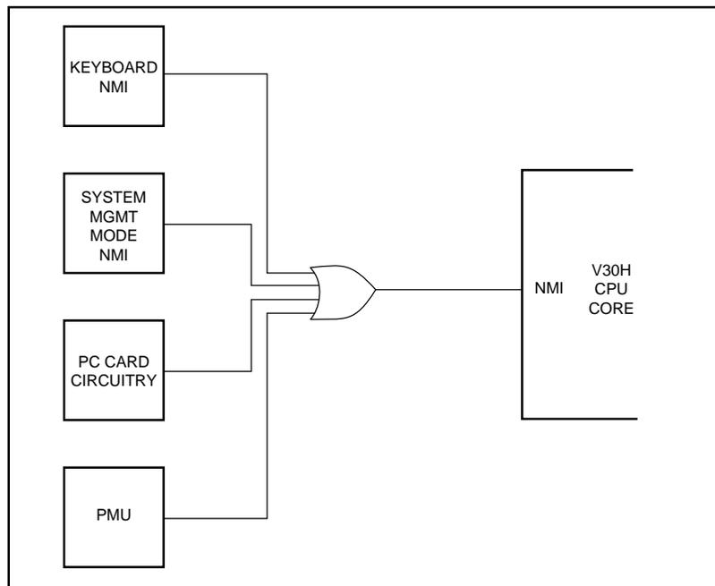
There are several NMI sources within the VG230. When an NMI occurs the NMI handler can determine the source of the NMI by first reading the Main NMI Status Register located at index 19H. The method of clearing the NMI depends on the source of the NMI.
