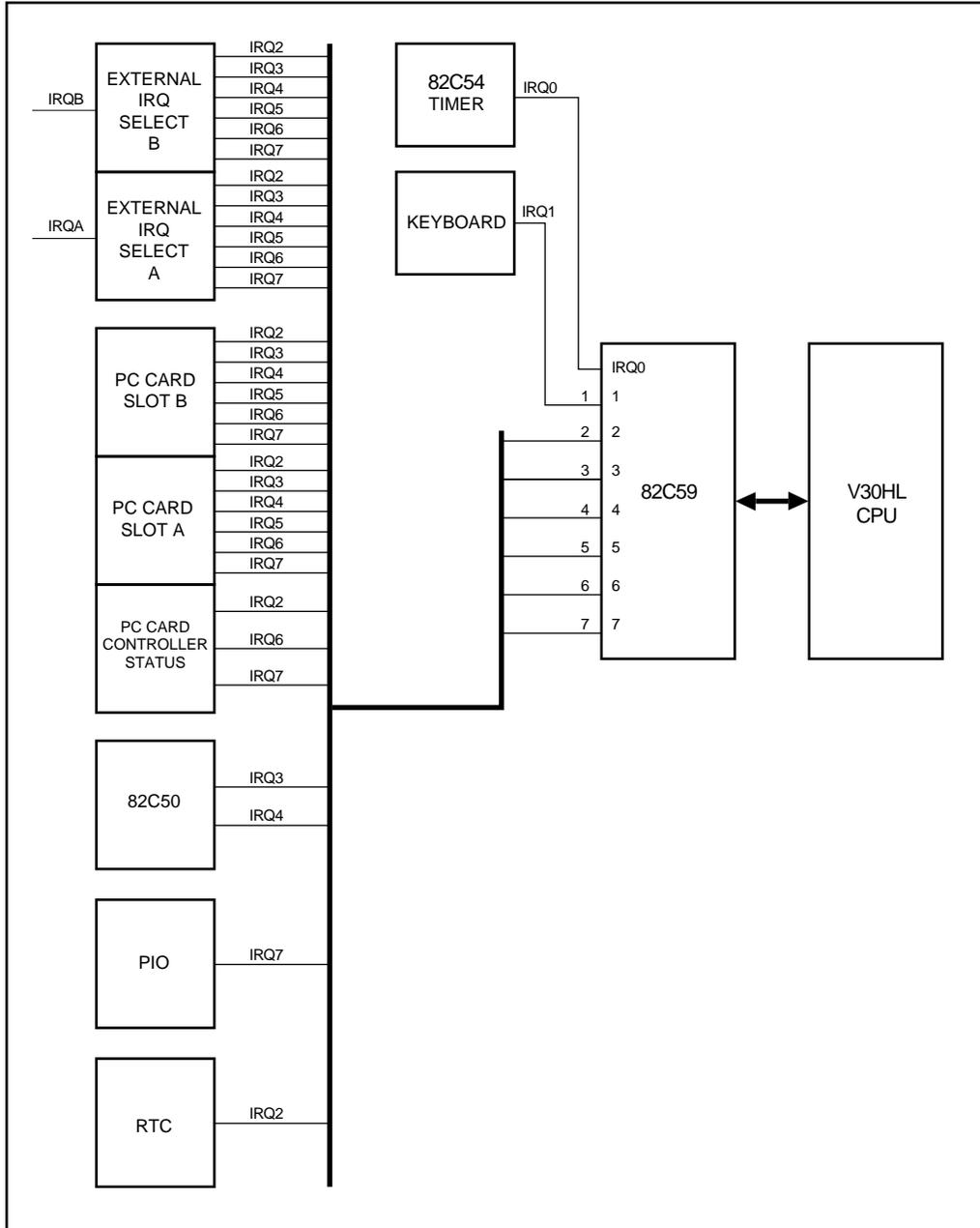
Two pins, IRQA and IRQB, provide support for the standard IRQ inputs. Each one of these inputs can support IRQ2-IRQ7. The selection of which IRQ input level is gated to the IRQA or IRQB inputs is controlled through the ICU mode register at index 0DH.
