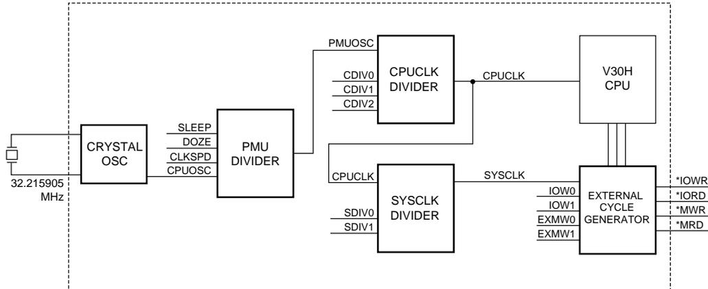
CPUCLK is derived from CPUOSC, and is configured through the BCG mode register at offset 01H. CDIV[2:0] select the divisor for CPUCLK. The default is CPUOSC/4.
