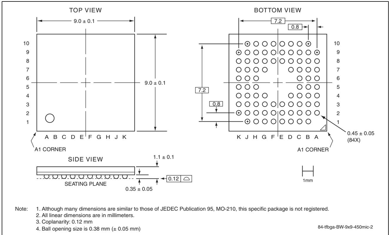
**FIGURE 15-3: 84-ball Thin, Fine-pitch, Ball Grid Array (TFBGA)**
