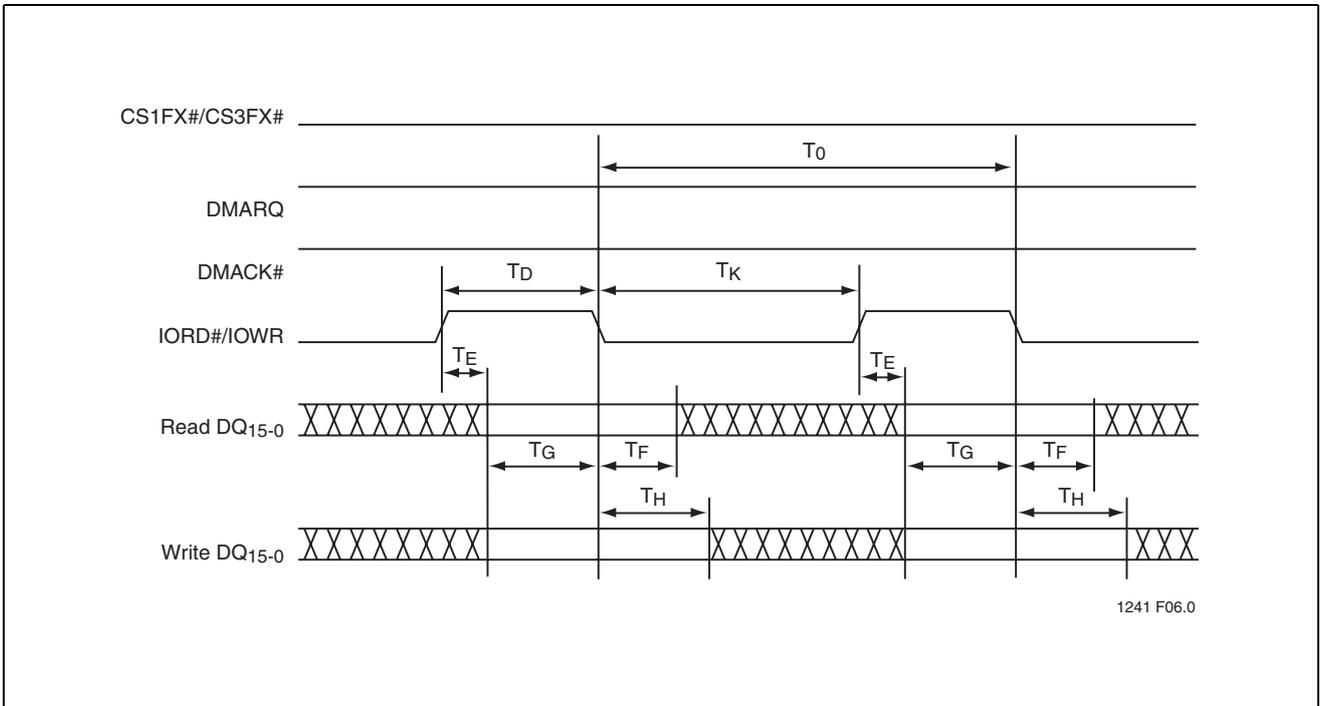
**FIGURE 12-5: Sustaining a Multi-word DMA Data Transfer**
