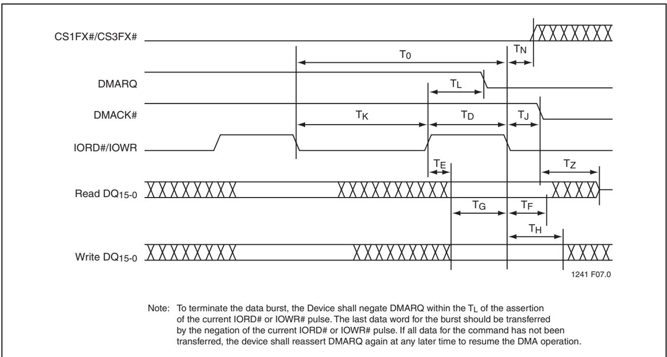
**FIGURE 12-6: Device Terminates a Multi-word DMA Data Transfer**
