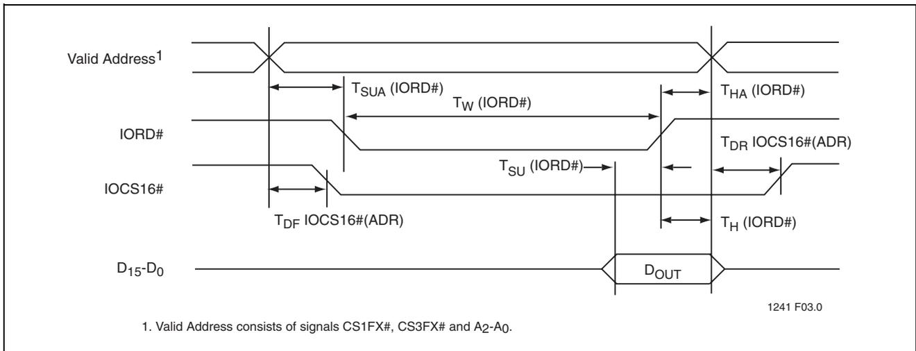
FIGURE 12-2: Host Side Interface I/O Read Timing Diagram
