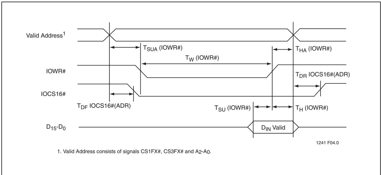
**FIGURE 12-3: Host Side Interface I/O Write Timing Diagram**
