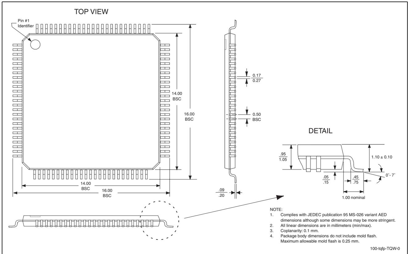
**FIGURE 15-1: 100-lead Thin Quad Flat Pack (TQFP)
