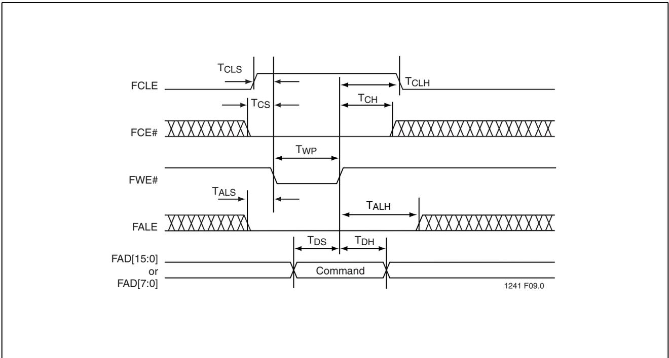
FIGURE 12-8: Media Command Latch Cycle
