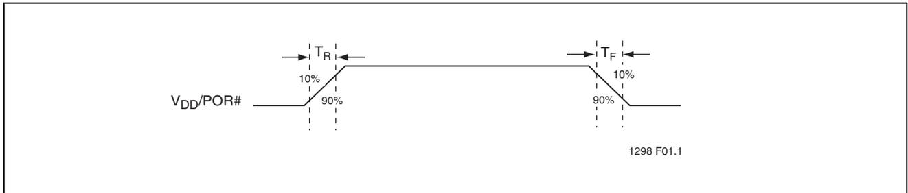
**FIGURE 9-1: Power-on and Brown-out Reset Timing (Commercial Temperature)**
