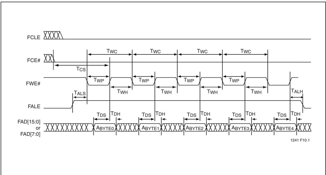
FIGURE 12-9: Media Address Latch Cycle
