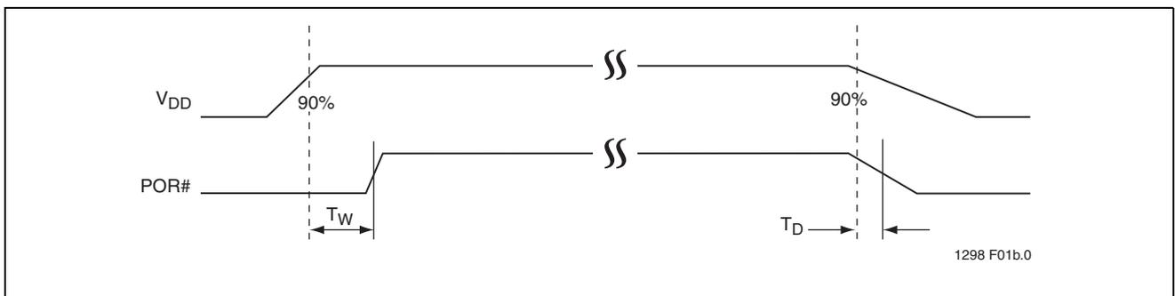
**FIGURE 9-2: Power-on and Brown-out Reset Timing (Industrial Temperature)**
