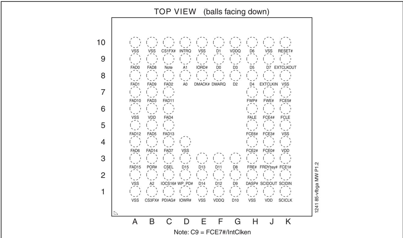
FIGURE 3-3: Pin Assignments for 85-ball VFBGA (MVW)
