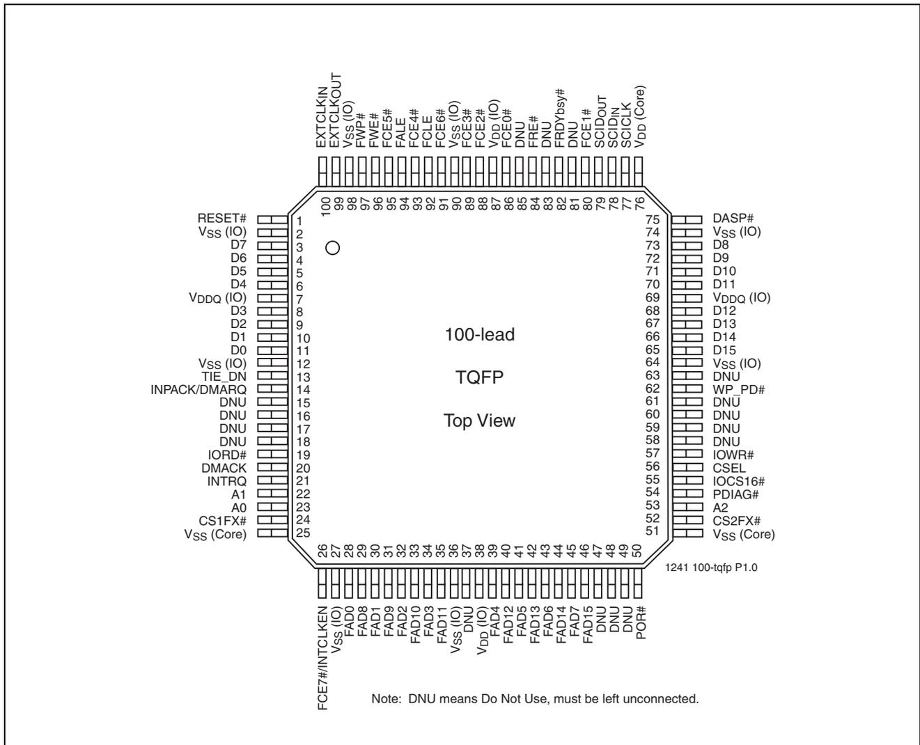
**FIGURE 3-1: Pin Assignments for 100-lead TQFP (TQW)**
