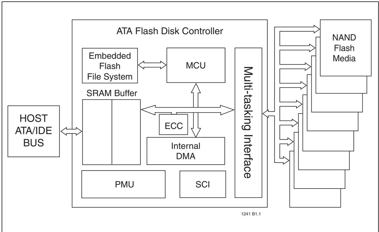
FIGURE 2-1: ATA Flash Disk Controller Block Diagram
