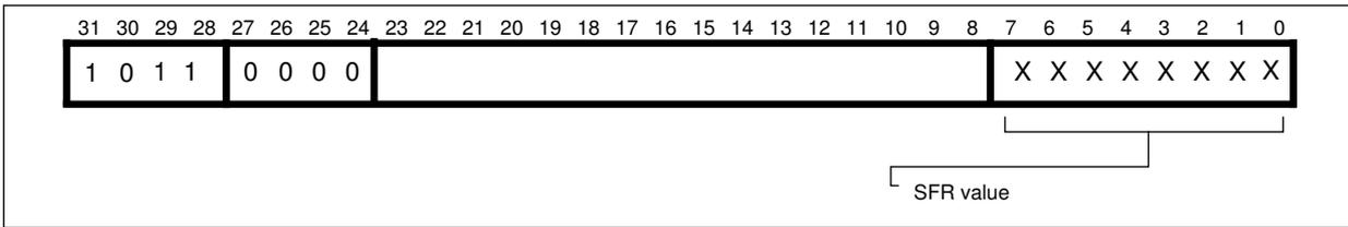
If a sample rate of N  $\mu$ s is required, then N-2 should be programmed into the SFR. N may take any value between 3 and 256.
