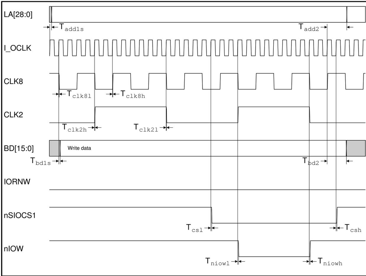
Figure 15-8: 'Sync' 8MHz Simple I/O write cycle timing
