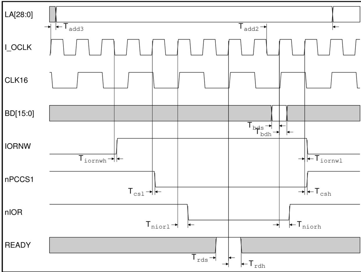
Figure 15-13: 16 MHz Type C read I/O cycle
