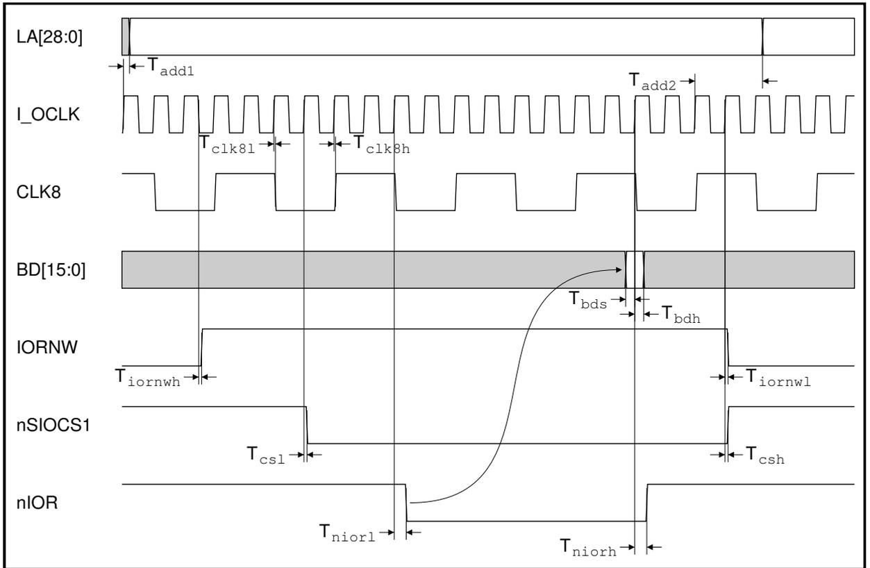
Figure 15-1: 'Fast' 8MHz Simple I/O read cycle timing
