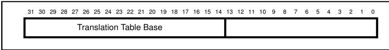
Register 2 is a write-only register which holds the base of the currently active Level One page table.
