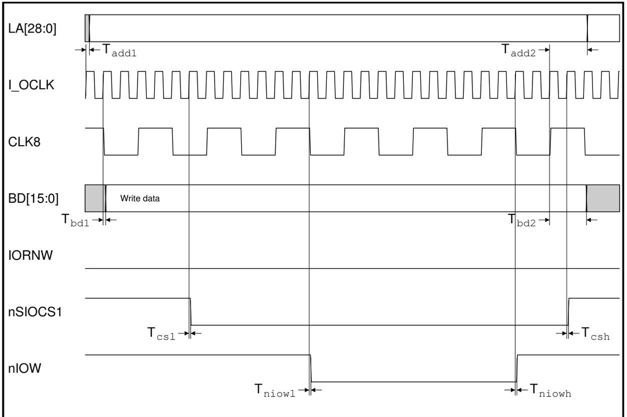
Figure 15-7: 'Slow' 8MHz Simple I/O write cycle timing
