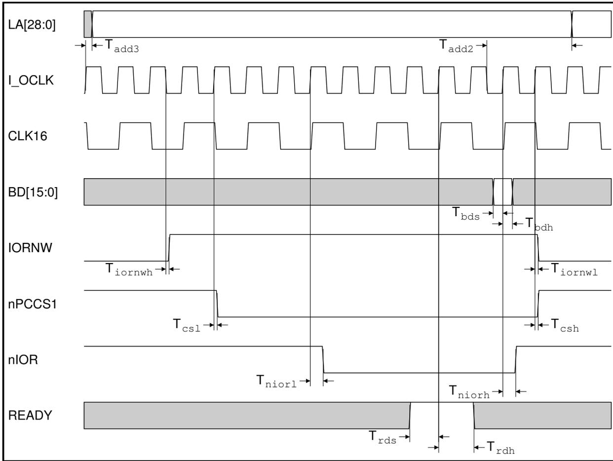
Figure 15-15: 16 MHz Type B read I/O cycle
