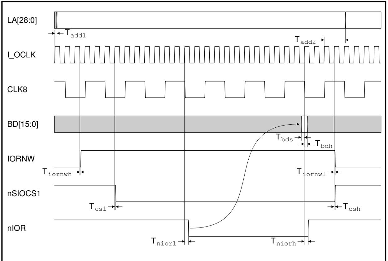
Figure 15-3: 'Slow' 8MHz Simple I/O read cycle timing
