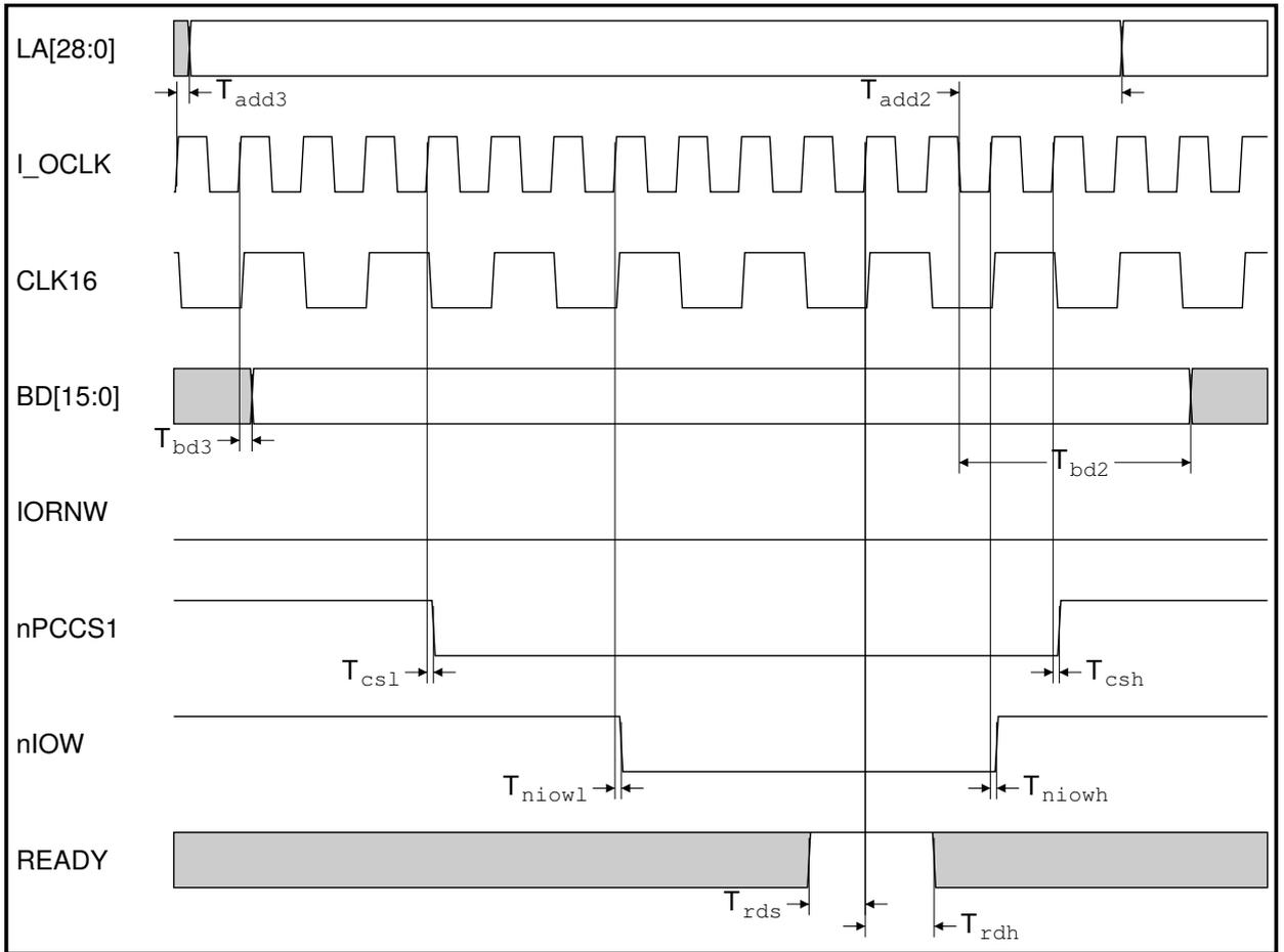
Figure 15-16: 16 MHz Type B write I/O cycle
