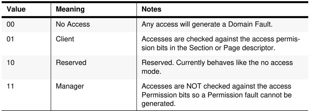
defines how the bits within each domain are interpreted to specify the access permissions.
