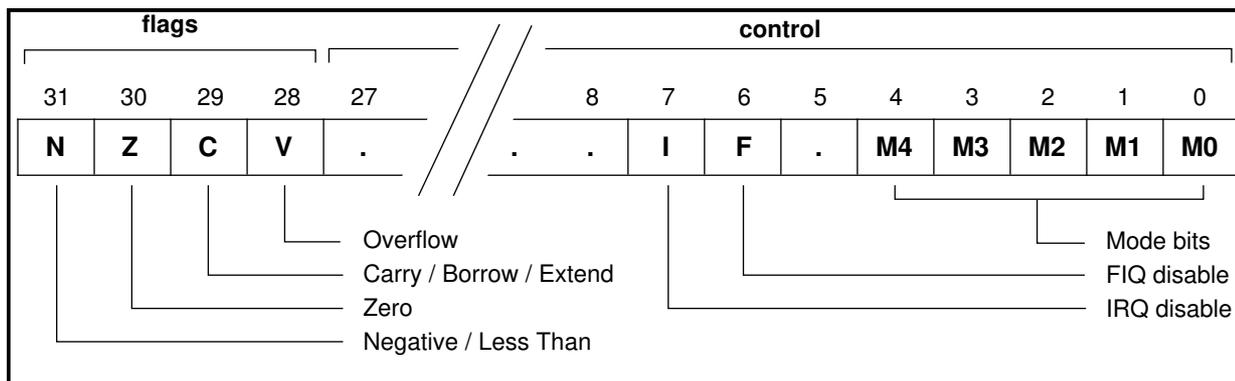
**Figure 4-4: Format of the Program Status Registers (PSRs)**
