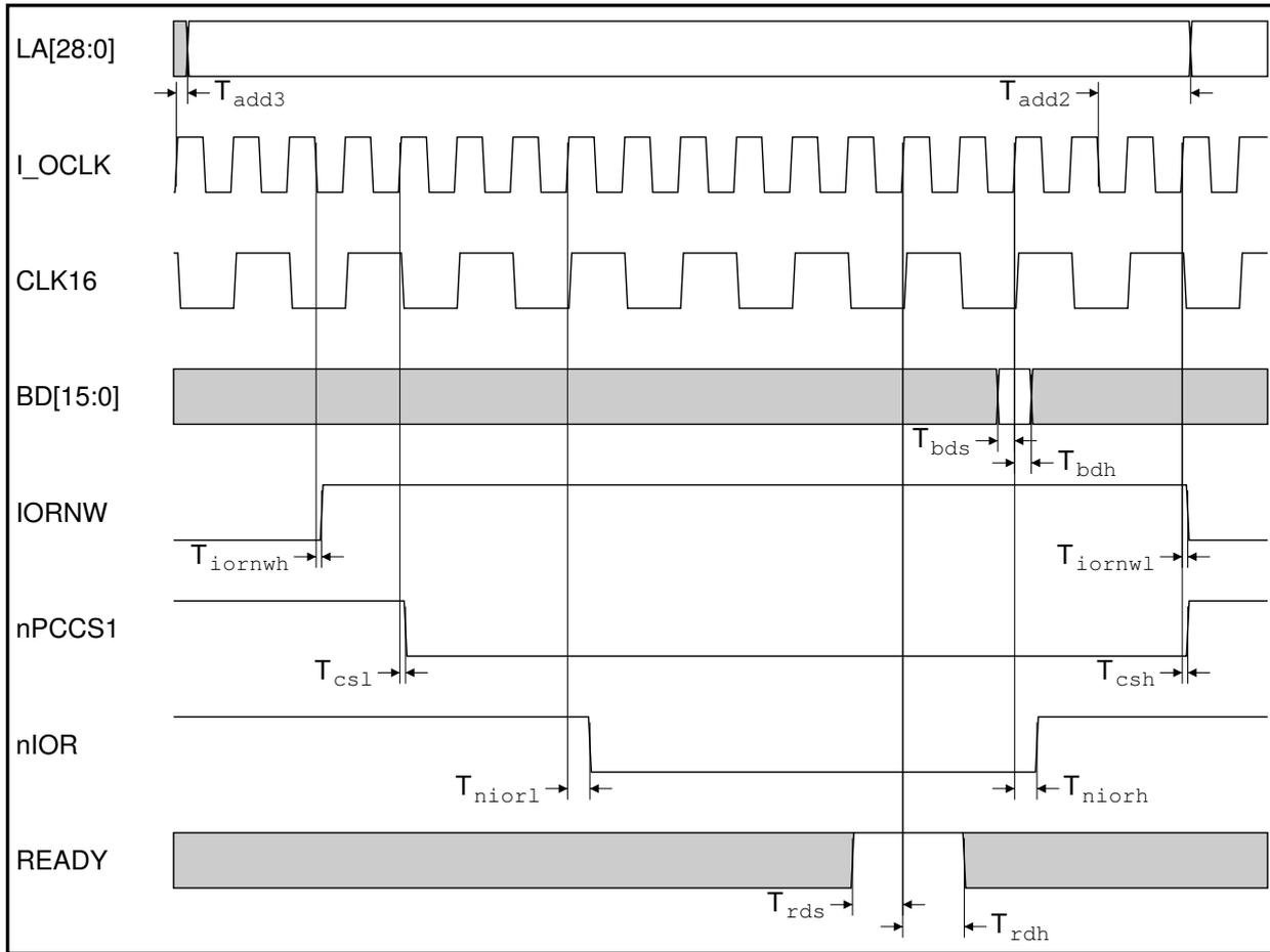
Figure 15-17: 16 MHz Type A read I/O cycle
