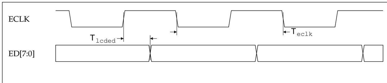
**Figure 11-2: Timing relationship between ECLK and ED in LCD greyscale mode**
