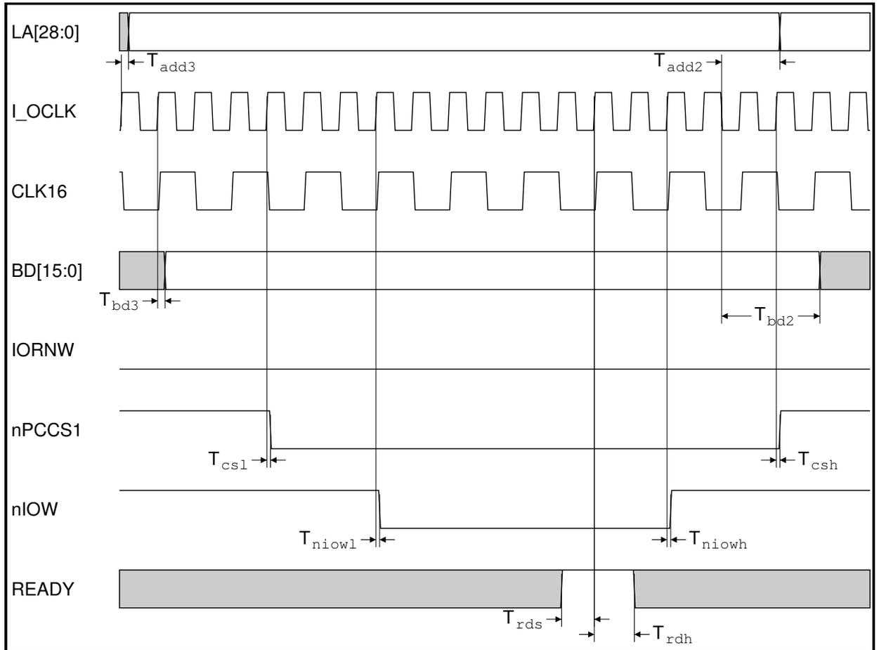
Figure 15-18: 16 MHz Type A write I/O cycle
