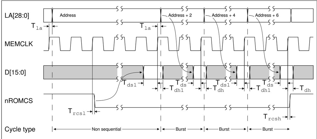
Figure 14-3: ROM access timing with burst mode—16-bit mode
