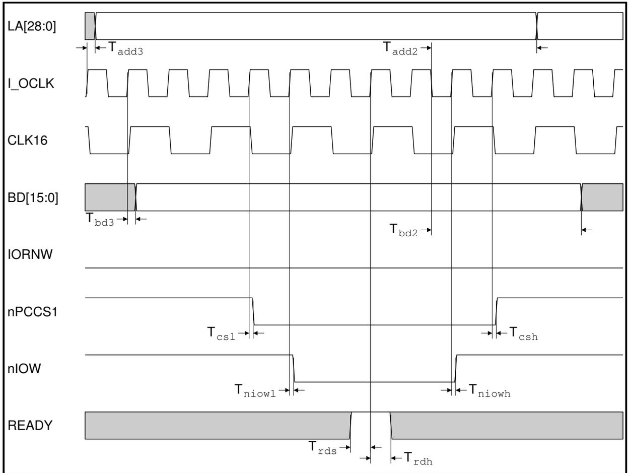
Figure 15-14: 16 MHz Type C write I/O cycle
