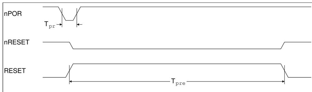
Figure 16-1: nPOR timing diagram
