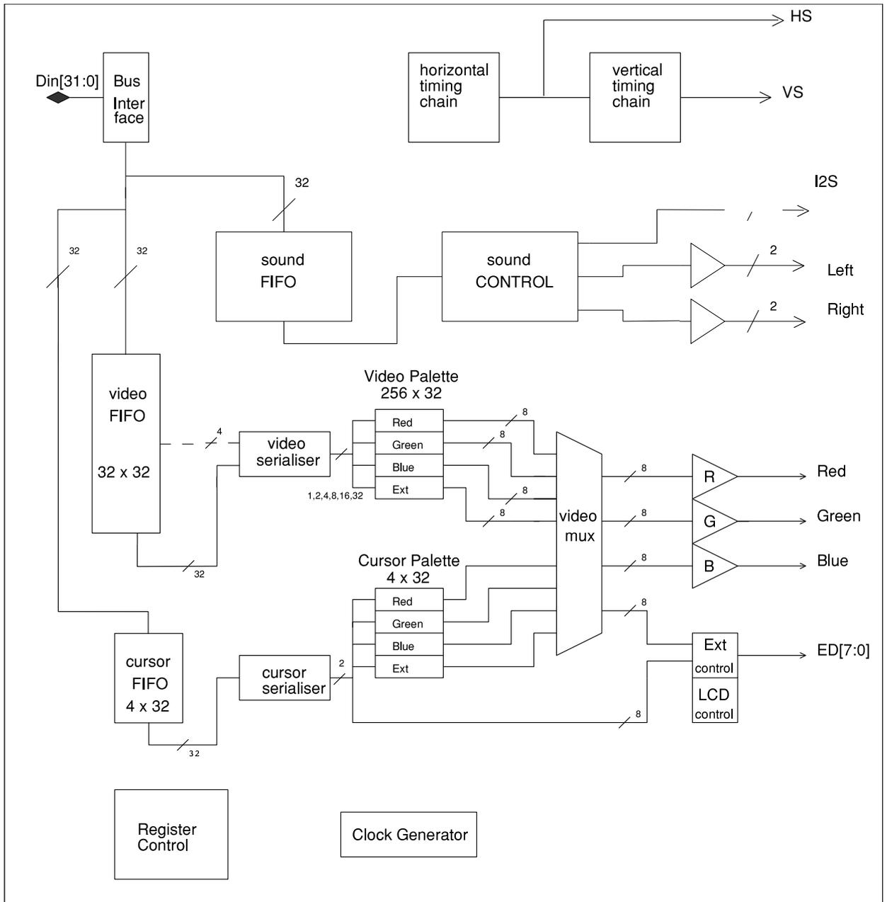
Figure 8-1: Video and sound macrocell block diagram
