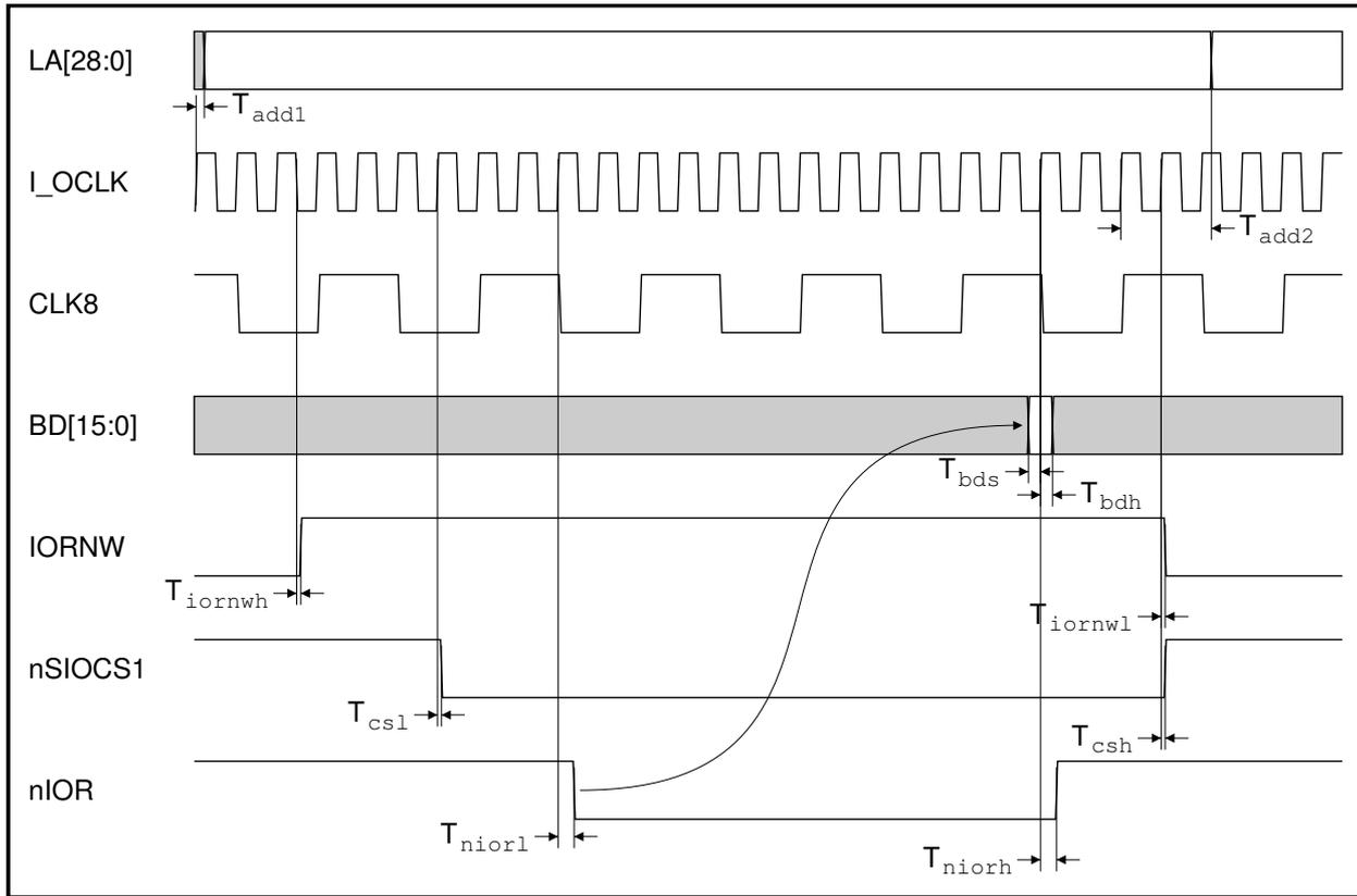
Figure 15-2: 'Medium' 8MHz Simple I/O read cycle timing
