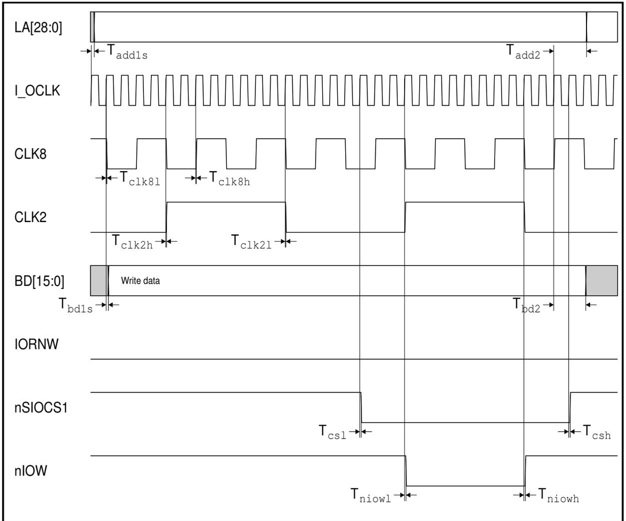
Figure 15-5: 'Fast' 8MHz Simple I/O write cycle timing
