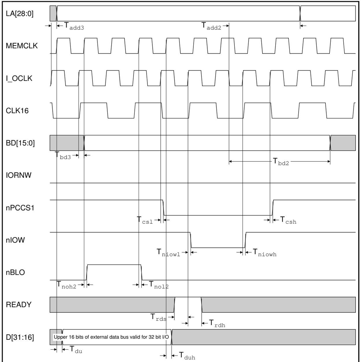
Figure 15-12: 16 MHz Type D write I/O cycle
