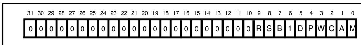
Register 1 is write only and contains control bits. All bits in this register are forced LOW by reset.
