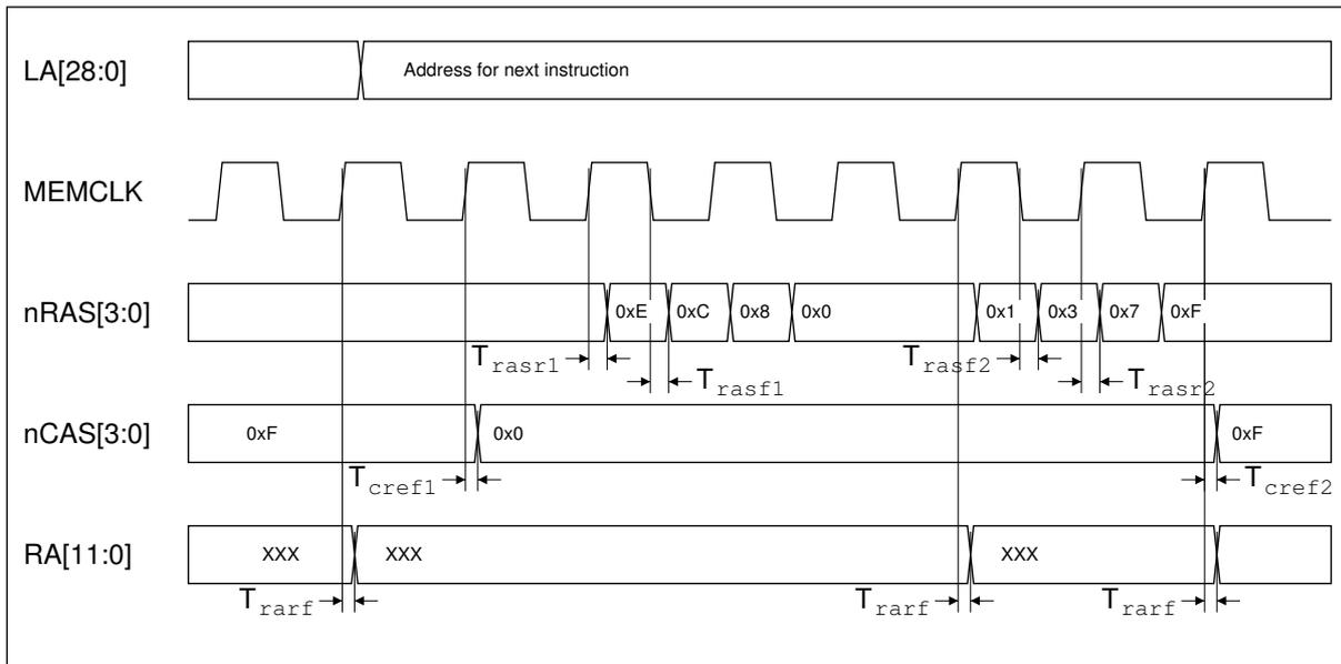
**Figure 14-8: Refresh cycle timing**
