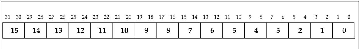
illustrates how the 32 bits of the register are allocated to define the sixteen 2-bit domains.
