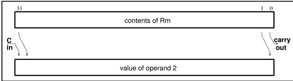
Figure 5-10: Rotate right extended
