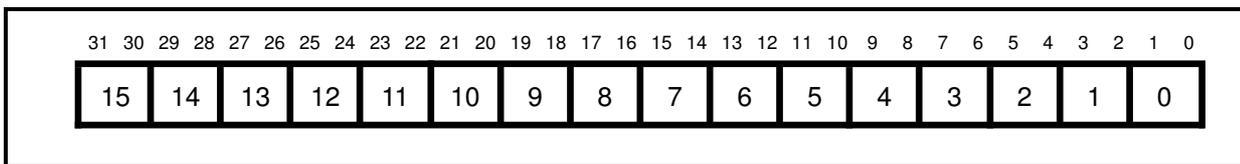
Register 3 is a write-only register which holds the current access control for domains 0 to 15. See [7.10 Domain access control](#) on page 7-13 for the access permission definitions and other details.
