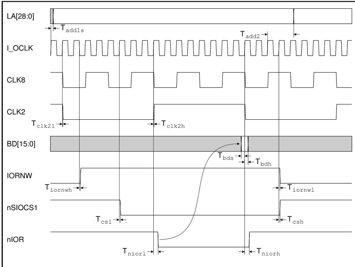
Figure 15-4: 'Sync' 8MHz I/O read cycle timing
