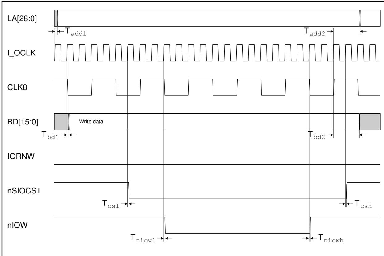
Figure 15-6: 'Medium' 8MHz Simple I/O write cycle timing
