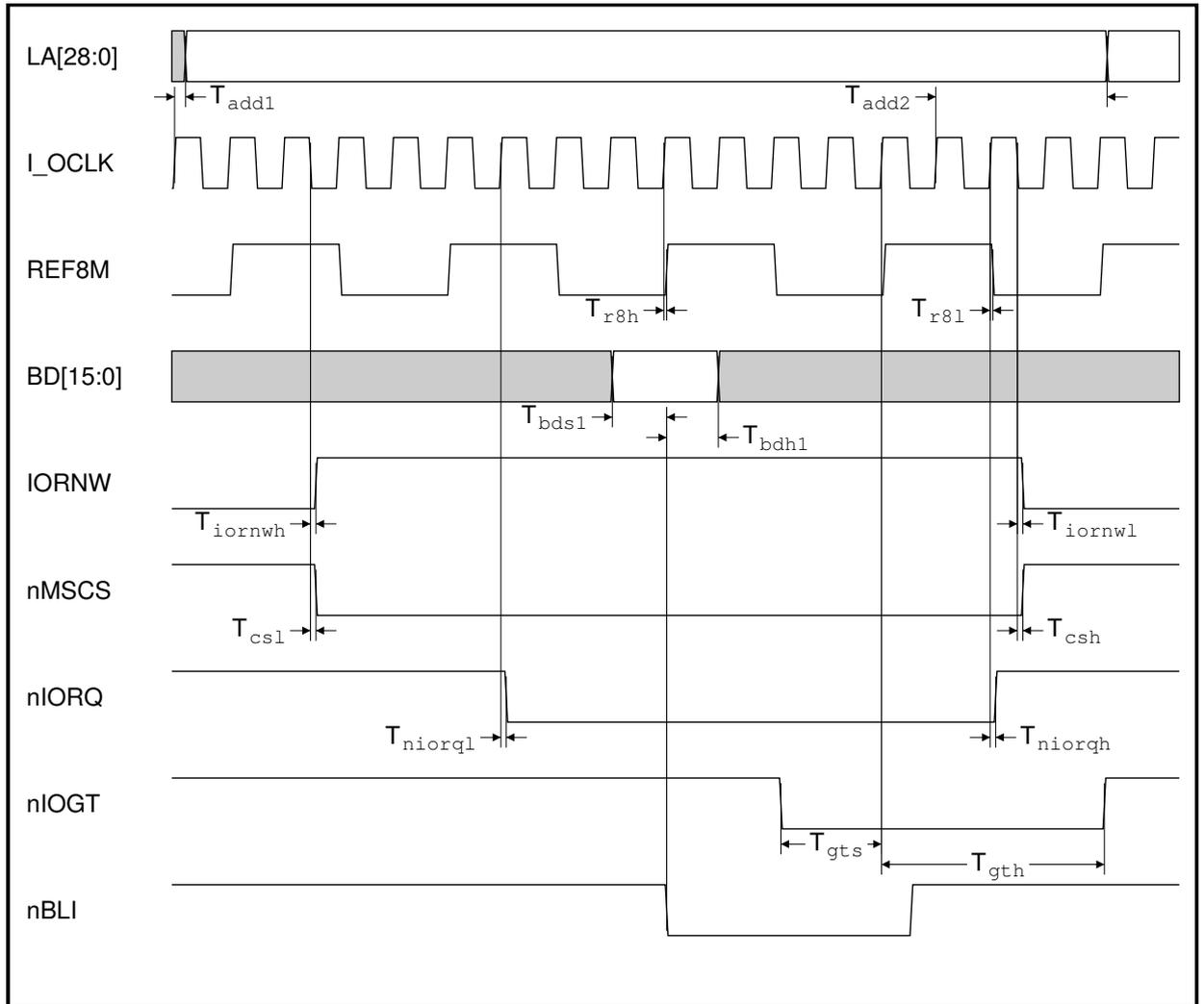
Figure 15-9: 8 MHz Module read I/O cycle
