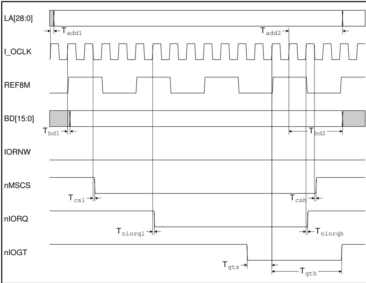
Figure 15-10: 8 MHz Module write I/O cycle
