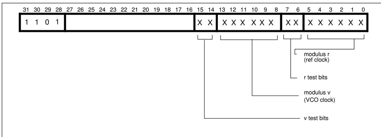
Associated with each counter are 2 test bits which should normally be programmed to 0.
