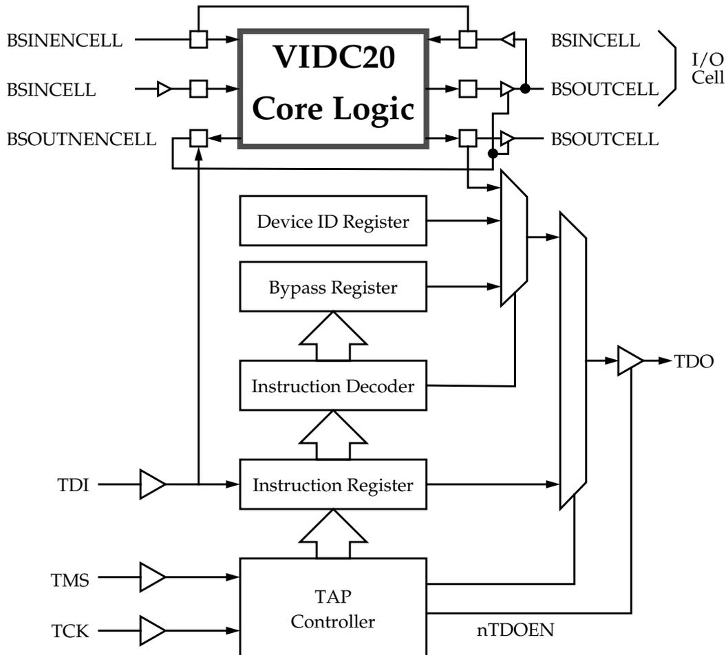
Figure 12: Boundary Scan Block Diagram
