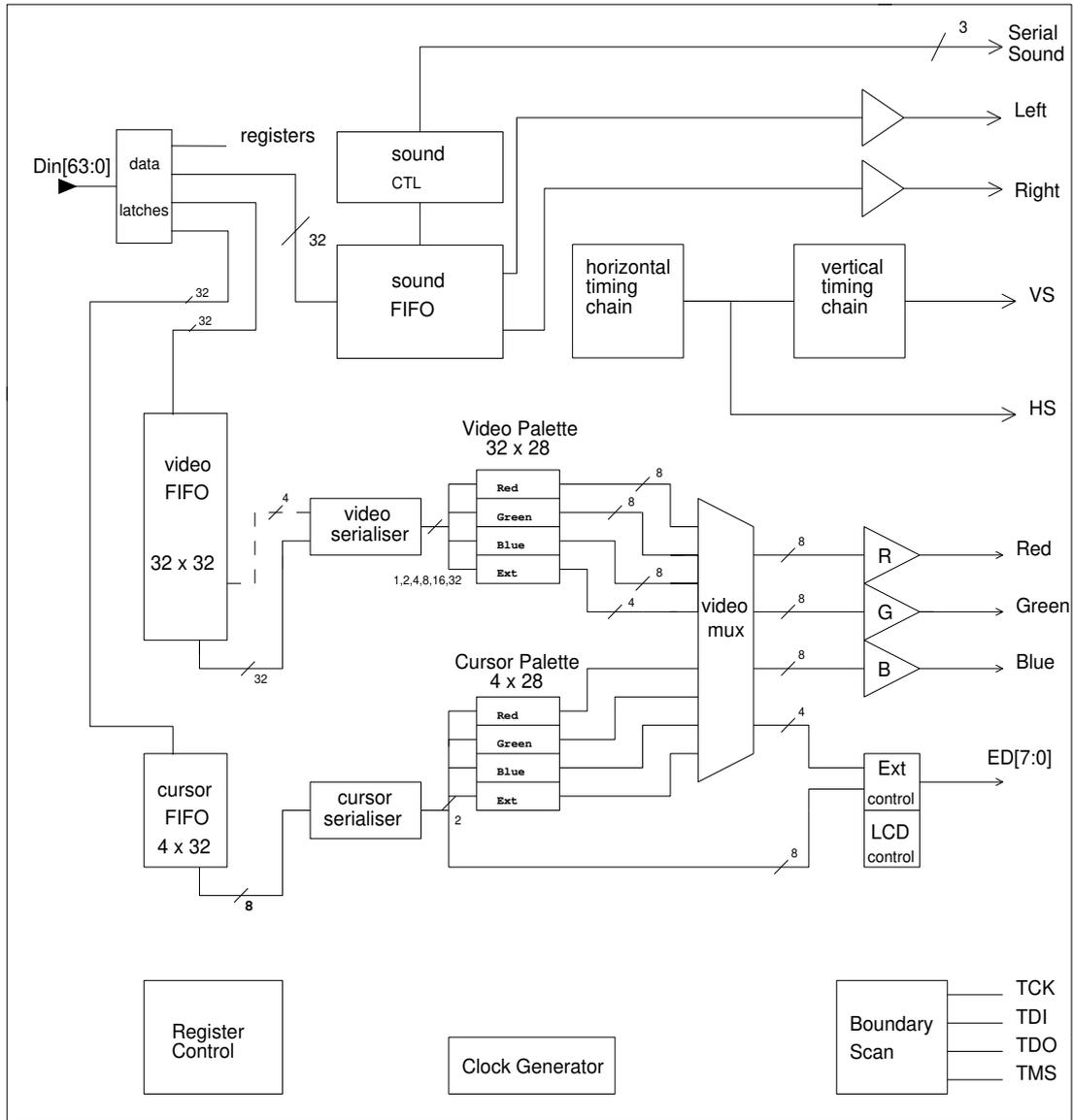
Figure 2: VIDC20 Block Diagram
