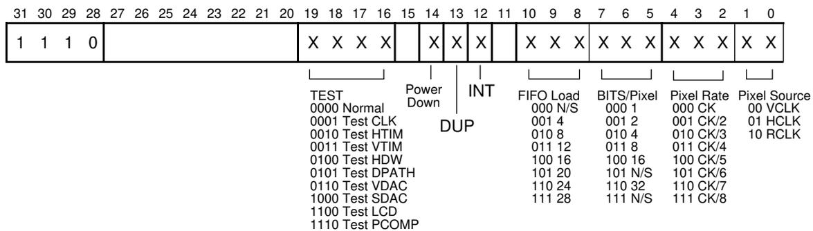
The pixel clock (`pixclk`) is selected from one of 3 sources, corresponding to the respective input pins, and the selected clock is then fed through a prescaler as defined by the 3 bits `conreg[4:2]`. The output of this prescaler is the actual pixel clock. See *Chapter 5.0 Pixel Clock* for more detail.
