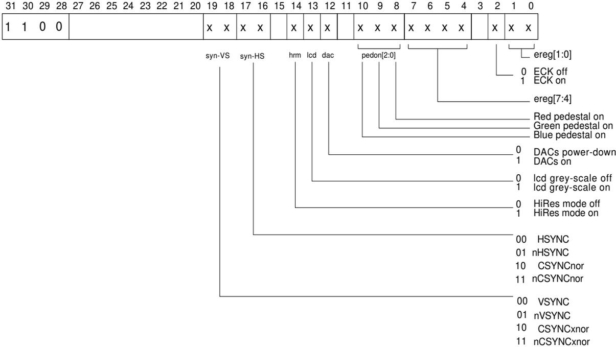
VIDC20 can export a variety of sync configurations on the pins **HSYNC** and **VSYNC**, as specified by the bits **syn-HS** and **syn-VS** respectively. For further explanation see *Chapter 11.0 External Support*.
