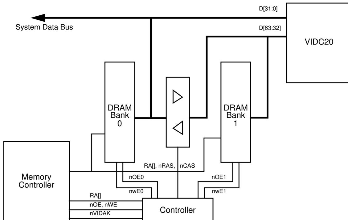
Figure 4: VIDC20 connected in 64 bit mode
