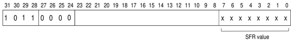
If a sample rate of N  $\mu$ s is required, then N-2 should be programmed into the SFR. N may take any value between 3 and 256.
