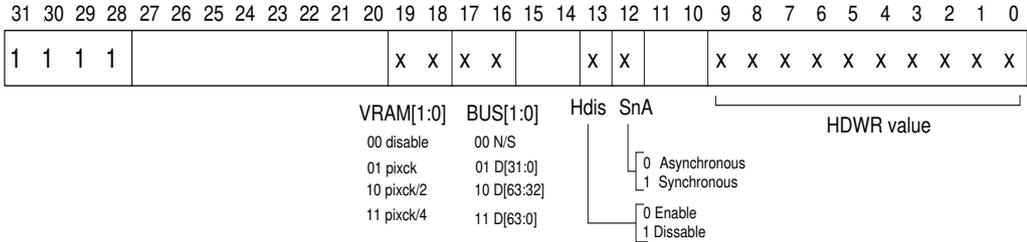
When using VIDC20 with VRAM, bits [19:18] must be programmed. These define the division of the pixel clock that is used to clock the VRAM (refer to *Chapter 3.0 System Configurations* for details). When the system memory does not contain Video RAM, these bits must be programmed to zero to save on power.
