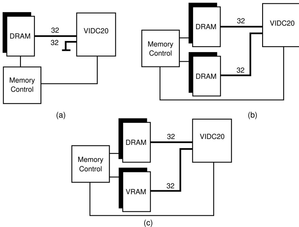
Figure 1: Typical Memory System Configurations
