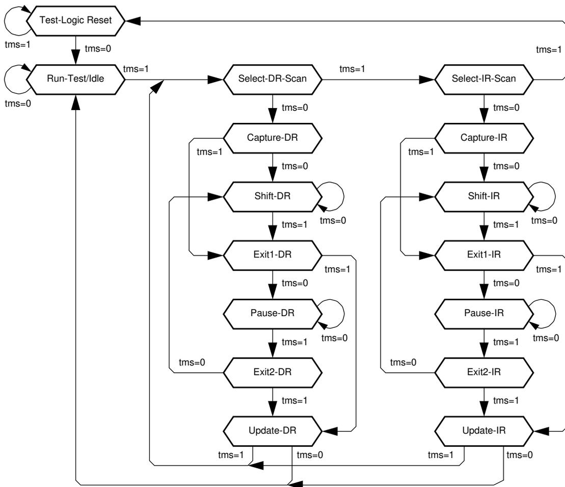
Figure 11: Test Access Port (TAP) Controller State Transitions
