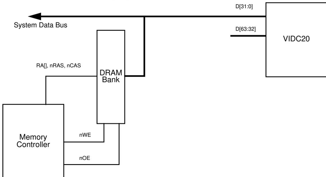
Figure 3: VIDC20 connected in Asynchronous 32 bit mode
