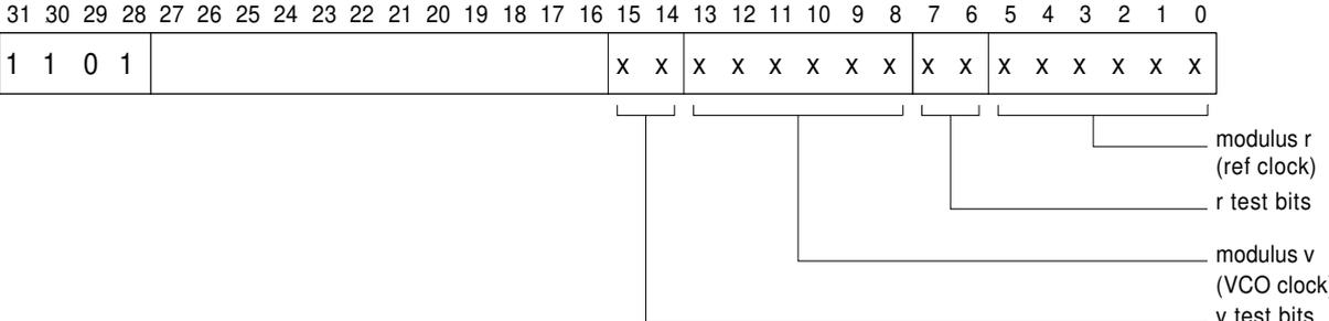
Associated with each counter are 2 test bits which should normally be programmed to 0.
