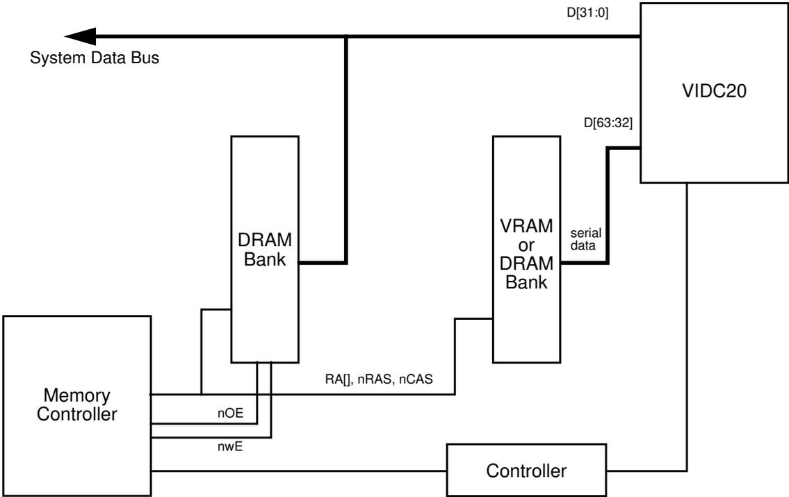
Figure 5: VIDC20 connected in Split Bank mode
