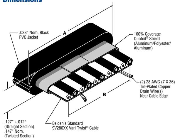
NOTE: the transition area is included in the twisted section to assure a full 2 inches of flat termination area.
