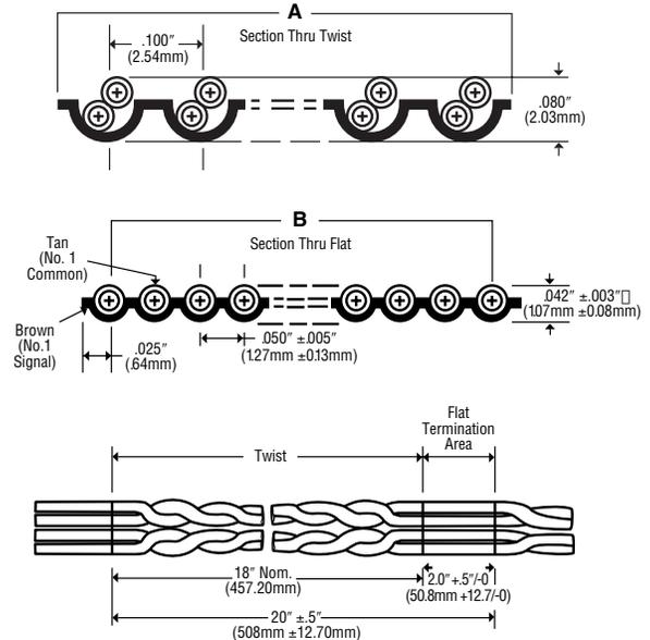
NOTE: the transition area is included in the twisted section to assure a full 2 Inches of flat termination area.
