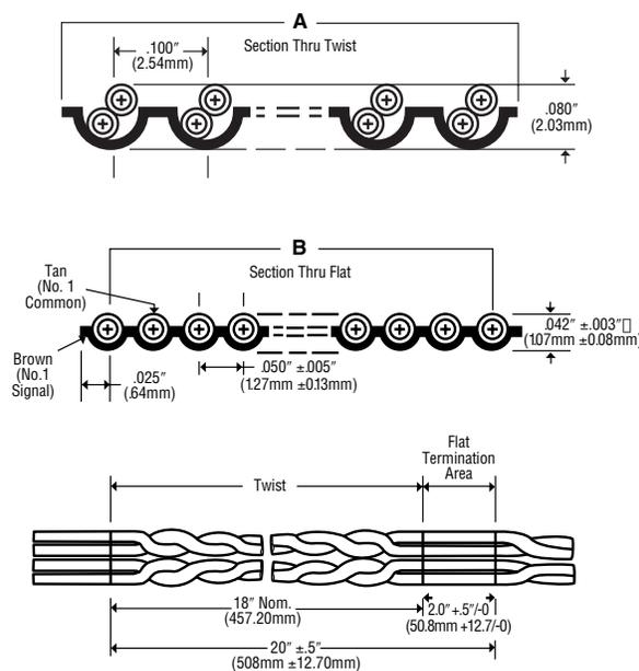
NOTE: the transition area is included in the twisted section to assure a full 2 inches of flat termination area.
