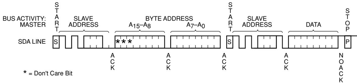
Figure 10. Sequential Read Timing
