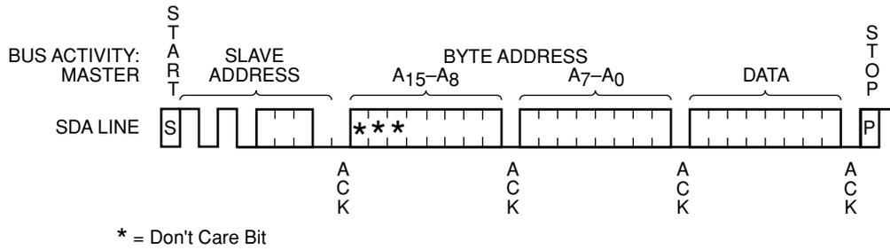
Figure 6. Write Cycle Timing
