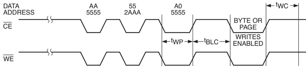
**Figure 12. Resetting Software Data Protection Timing**
