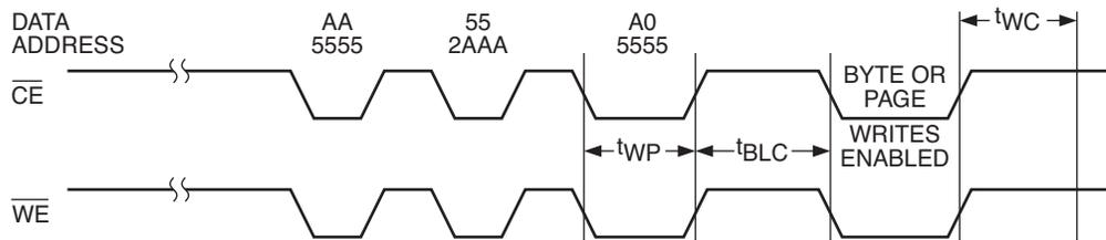
**Figure 12. Resetting Software Data Protection Timing**
