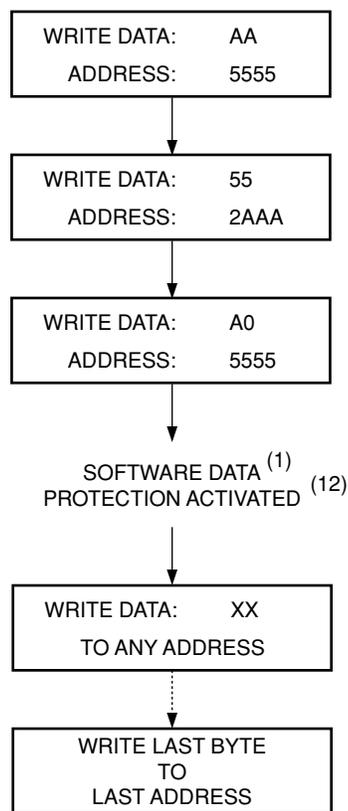
**Figure 10. Write Sequence for Deactivating Software Data Protection**
