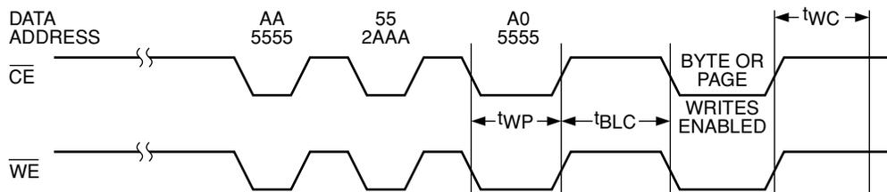
**Figure 12. Resetting Software Data Protection Timing**
