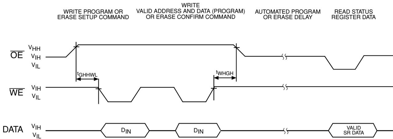
Figure 9. Alternate AC Waveform for Write Operations
