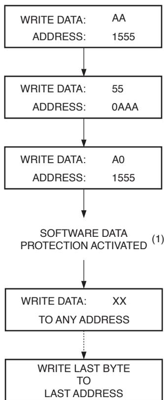
**Figure 10. Write Sequence for Deactivating Software Data Protection**
