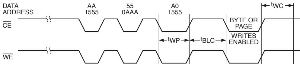
**Figure 12. Resetting Software Data Protection Timing**
