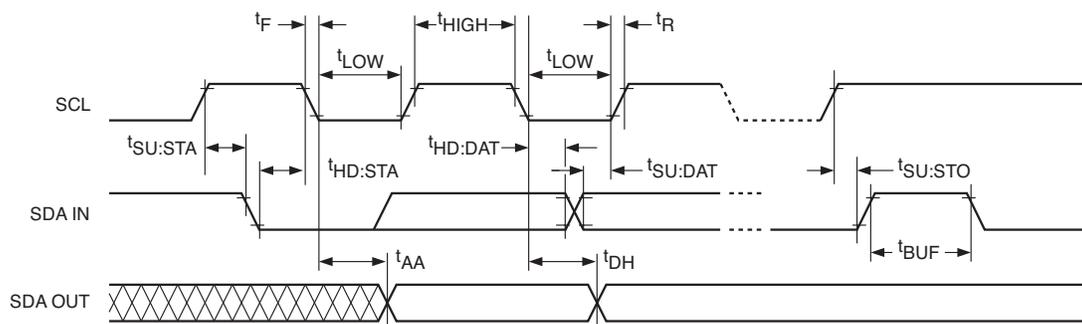
Figure 5. Write Cycle Timing
