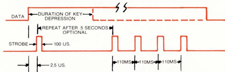
**10 Strobe Pulse Width** — The keyboard as supplied will generate a STROBE and  $\overline{\text{STROBE}}$  pulse width of approximately 100 microseconds. To vary the pulse width, change the value of R8 and/or C3. R8 may be any value from 4.7K to 47K. The pulse width will change in proportion to the resistor value. For large changes in pulse width, change C3 to .002 mfd for approximately a 10 microsecond pulse ... or change C3 to .2 mfd for a pulse width of approximately 1 millisecond.
