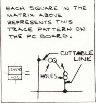
**6 Flexible Key Assignments** — When it is desired to change the code of a key which comes factory wired, first locate the key module terminal solder connections on the bottom of the printed circuit board. There is a trace coming from each of the key's solder connections to two pads with two plated-through holes.
