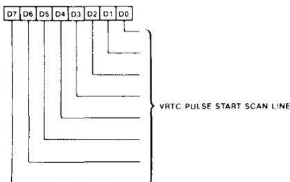
The Vertical Retrace Start Register is a 9-bit address which defines the scan line position of the VRTC pulse. The low order 8 bits are programmed through this register, while the high order ninth bit is programmed through the Overflow Register, CR7.
