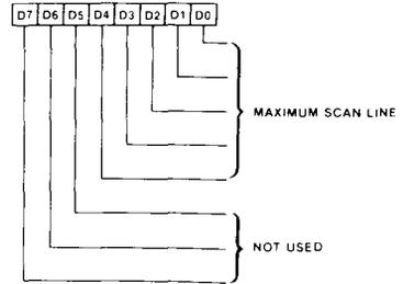
The contents of the Maximum Scan Line Register specifies the number of scan lines per character row. This actual number of scan lines per row is the contents of this register plus one.
