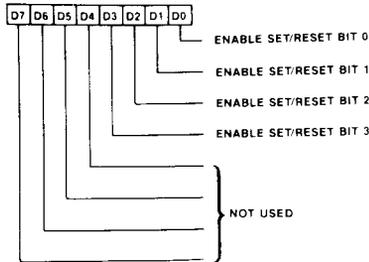
The Enable Set/Reset Register works in conjunction with the Set/Reset Register. If the Graphics Mode Register is programmed to write mode 0, and Set/Reset is enabled (=1), then the contents of the Set/Reset Register determine the data to be written to the respective display memory planes. If write mode 0 is selected and Set/Reset is not enabled (= 0) on a plane, the plane is written with the data from the CPU data bus.
