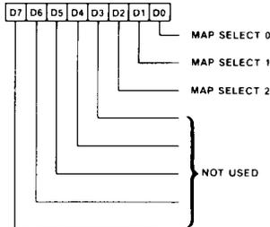
The contents of the Read Map Select Register represent the memory plane from which the CPU reads the data in read mode 0. This register does not effect the read operation performed through the Color Compare Register (read mode 1). The four memory maps are selected as follows:
