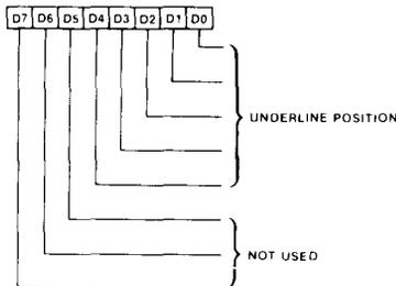
The Underline Location Register specifies the scan line within a character row at which the underline will appear for underlined characters. The value in the register should be one less than the desired scan line number.
