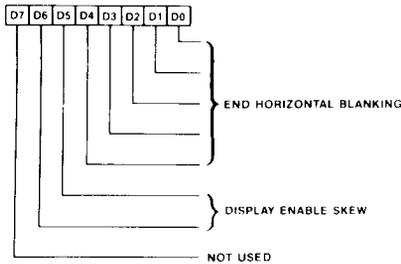
The contents of the End Horizontal Blanking Register define the time when the horizontal blanking will terminate. The register is defined in terms of the number of character clocks.
