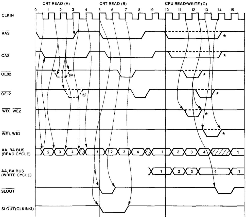
@ NOE<sub>x</sub> ACTIVE DURING CRT READ CYCLE A ONLY FOR HIGH CRT BANDWIDTH MODE (SR0-D1=0)
