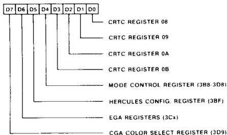
Tag Registers 0 and 1 are located at offset 0F7h (Tag Register 0) and 0F8h (Tag Register 1) in the CRT Controller. They can be accessed by first writing 0F7h/0F8h in the CRTC Address Register (I/O address 3B4h/3D4h) and then accessing the CRTC Data Register (I/O address 3B5h/3D5h).
