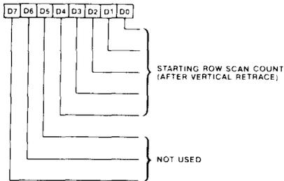
D0-D4 of the Preset Row Scan Register specify the starting row scan count after a vertical retrace. Each horizontal retrace increments the character row scan line counter. The horizontal row scan counter is cleared at maximum row scan count, which is programmed through register CR9. This register is used for soft scrolling in text modes and in the Hercules Graphics or CGA graphics modes.
