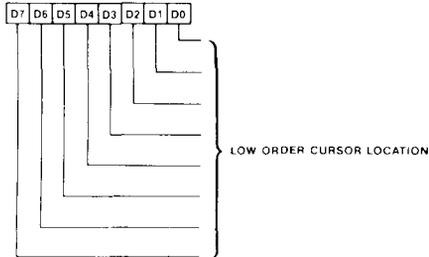
In conjunction with the Cursor Location High Register, the Cursor Location Low Register defines the low order 8 bits of the cursor location.
