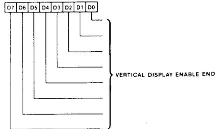
The Vertical Display Enable End Register defines 8 bits of the 9-bits address which specifies the scan line position where the display on the screen ends. The ninth bit is located in the Overflow Register CR7.
