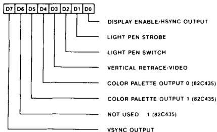
The Input Status Register I exists in both the 82C435 and the 82A436. This register changes address and format in the EGA, CGA and Hercules modes. In EGA mode this register is located at I/O address 3BAh/3DAh. In CGA mode this register is located at I/O address 3DAh. In Hercules mode this register is located at I/O address 3BAh. When this register is read, the 82C435 and 82A436 drive different bits in the three modes as follows:
