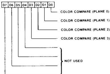
If the Graphics Mode Register is set to Read Mode 1, each bit of data read from the display memory planes 0-3 is compared to bits D0 through D3 programmed in the Color Compare Register and the Color Don't Care Register. A match between the memory data and the Color Compare Register (for the bits as specified in the Color Don't Care Register) results in a logical 1 being output on the corresponding data bus bit. Following is an
