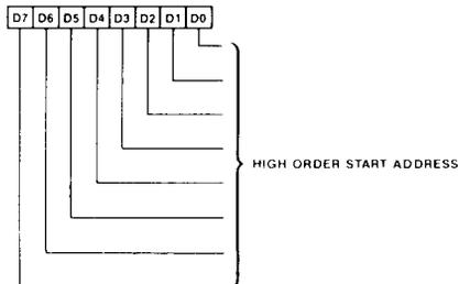
The Start Address is a 16-bit value which specifies the first word address in the display buffer for the screen refresh process. This display buffer address is mapped to the upper left corner of the screen. The Start Address High Register contains 8 high order bits of the address, while the Start Address Low Register specifies the other 8 low order bits. Byte resolution on this address can be achieved through the Extended Mode Register (CRF9 - bit D1).
