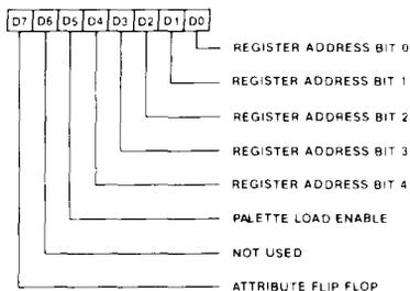
D0-D4 are used to point to the internal data registers in the Attributes Controller.
