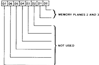
The Graphics B Position Register selects the CPU data bus signals and directs them to/from display memory planes 2 and 3. This register should normally be programmed to 01h to select D2 and D3 for display memory planes 2 and 3 respectively.
