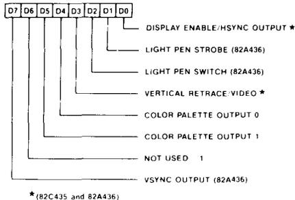
Parts of the Input Status Register I exist in both the 82C435 and the 82A436. The data path to the CPU from the 82C435 always goes through the 82A436. When the CPU reads this register, depending on the current emulation mode, the 82A436 reformats the status data output by the 82C435 and passes the final status to the CPU.
