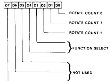
The Data Rotate Register is used to perform a rotate function on the data written by the CPU. If the Graphics Mode Register is programmed for write mode 0, then the value in the Rotate Count Field represents the number of bits the CPU data will be rotated (right) during the CPU write cycles. The CPU data bits are first rotated and then subject to the logical operation as specified in the Function Select Field.
