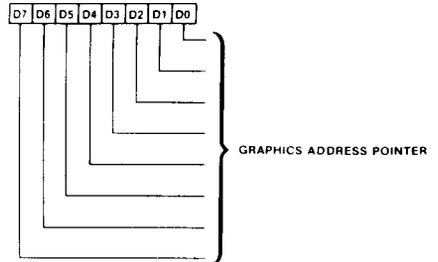
The Graphics Address Register is used to point to other registers in the Graphics Controller. The four least significant bits determine the register which will be pointed to in the next register write operation. When this register is read, D5, D6 and D7 are always '1'. D4 is '1' if D5, D6 and D7 were written as 1. D4 is '0' if D5, D6 or D7 were written as '0'.
