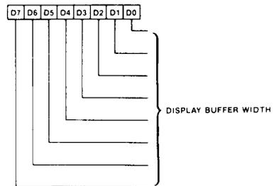
The Offset Register contents define the width of the Display Buffer currently used. This register is used to compute the memory starting address for the next display row (or scan line in graphics modes). The byte starting address of the next display row is computed as follows:
