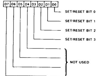
When the Graphics Mode Register selects write mode 0, and the Set/Reset mode is enabled through the Enable Set/Reset Register, bit 0 of this register is written to the entire addressed byte in display memory plane 0. Similarly bits 1, 2 and 3 determine the data to be written into display memory planes 1, 2 and 3 respectively.
