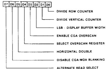
The 400 Line Register is located at offset 0F9h in the CRT Controller. This register can be accessed by first writing 0F9h in the CRTC Address Register (I/O address 3B4h/3D4h) and then accessing the CRTC Data Register (I/O address 3B5h/3D5h).
