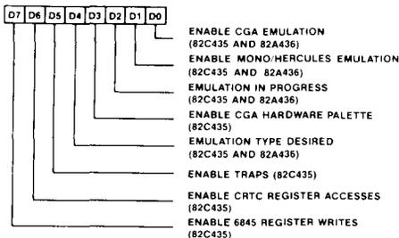
The Emulation Mode Register exists in both the 82C435 and the 82A436. This register is located at offset 0FFh in the CRT Controller register space. In the 82A436 this is a write only register and only bits 0, 1 and 2 are implemented. These bits are also present in the 82C435. When this register is read, the 82C435 drives the local data bus and the 82A436 transfers the contents of the local data bus to the CPU.
