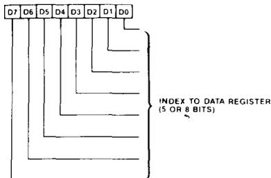
The CRT Controller Registers are all located at two byte addresses in the CPU I/O space. The registers are accessed by first writing a pointer to the actual data register into the CRT Controller Address Register and then accessing the CRT Controller Data Register. The Address Register is located at I/O address 3B4h/3D4h. The data registers are all located at I/O address 3B5h/3D5h. The exact address 3Bx/3Dx is selected through bit D0 of the EGA Misc. Output Register.
