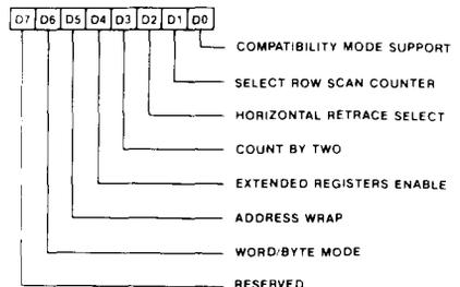
The CRT Mode Control Register is a multi-function register, with each bit defining a different option. Following is a description of these bits:
