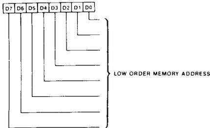
The Light Pen Low Register contains the 8 low order bits of the memory address displayed when the light pen strobe signal was triggered. The high order 8 bits are stored in the Light Pen High Register (CR10).
