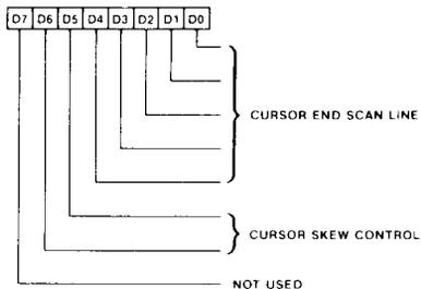
The Cursor End Register defines the scan line within a character row where the cursor block is to end. It also controls the cursor skew as described below:
