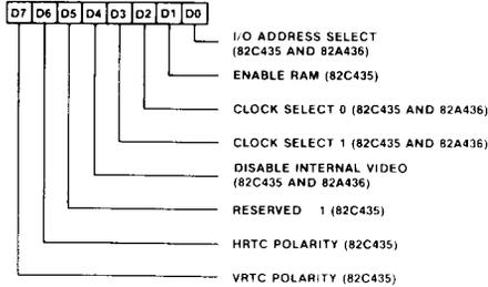
The EGA Miscellaneous Register exists in both the 82C435 and the 82A436. This register is located at I/O address 3C2h. In the 82A436, this is a write only register and only bits 0, 2, 3, and 4 are implemented. These bits are also present in the 82C435. When this register is read, the 82C435 drives the local data bus and the 82A436 transfers the contents of the local data bus to the CPU.
