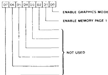
The Hercules Configuration Register is effective only when Hercules emulation is in progress (CRFF bit D2 = 1) and EGA Misc Output Register bit D0 = 0. Bits D0 and D1 are read at bits D6 and D7 respectively in the Sequencer Address Register (I/O Address 3C4h).
