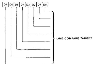
The Line Compare Register is used to implement a split screen function. When the scan line counter value is equal to the contents of this register, the memory address generator is cleared to 0. The display buffer address generator then sequentially addresses the display buffer starting at address 0. Each subsequent row address is generated by the addition of Offset Register contents.
