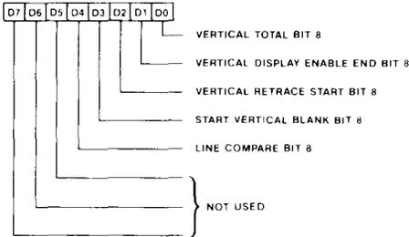
The CRT Controller Overflow Register contains the ninth bit (D8) of Vertical Total, Vertical Retrace Start, Start Vertical Blanking and Line Compare Registers.
