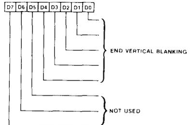
The End Vertical Blanking Register specifies the scan line count at which vertical blanking becomes inactive. The vertical blanking width,  $W$ , is determined as follows:
