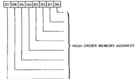
The Light Pen High Register contains the 8 high order bits of the memory address that was displayed when the light pen strobe signal was triggered. The low order 8 bits are stored in the Light Pen Low Register (CR11).
