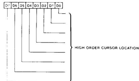
The Cursor Location address is a 16-bit value. The 8 high order bits are programmed in the Cursor Location High Register. The other 8
