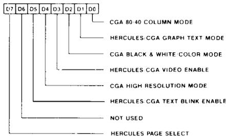
All the bits in the Hercules/CGA Mode Control Register are effective only when emulation is in progress (CRFF bit D2 = 1). When CGA emulation is in progress (EGA Misc. Output Register bit D0 = 1), then this register functions as the CGA Mode Register and is located at I/O address 3D8h. When Hercules emulation is in progress (EGA Misc. Output Register bit D0 = 0), then this register functions as the Hercules Mode Register and is located at I/O address 3B8h.
