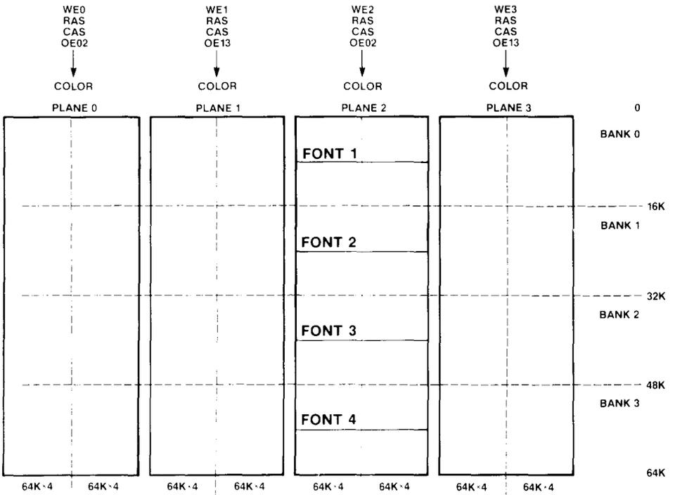
IN GRAPHICS MODE: PLANES 0-3 CONTAIN 1 BIT EACH OF A 4 BIT PIXEL. A TOTAL OF 64K PIXELS CAN BE STORED IN MEMORY IN THIS MODE.
