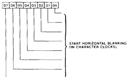
The contents of the Start Horizontal Blanking Register define the time when the horizontal
