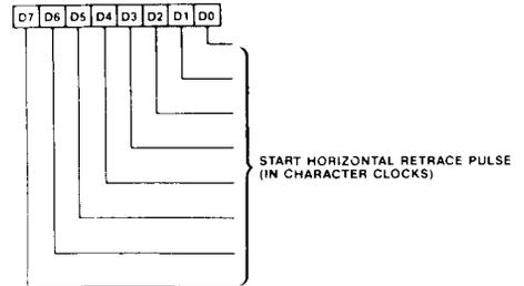
The Start Horizontal Retrace Pulse Register defines the character position at which the Horizontal Retrace Pulse becomes active. It is used to center the monitor screen horizontally. The value in the register is the character count at which the Horizontal Retrace Pulse becomes active.
