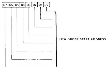
The Start Address Low Register contains the 8 low order bits of the Start Address (word address).
