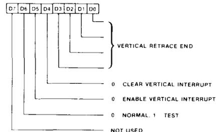
The Vertical Retrace End Register performs multiple functions, as described below:
