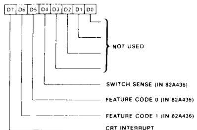
Parts of the Input Status Register 0 exist in both the 82C435 and the 82A436. The data path to the CPU from the 82C435 always goes through the 82A436. When the CPU reads this register, the 82A436 reformats the status data put out by the 82C435 and passes the final status to the CPU.
