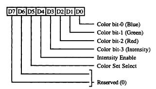
This register is a copy of the CGA color select register 3D9h. Writes to this register will change the copy at 3D9h. It is effective in CGA emulation mode. The copy at 3D9h is visible only in CGA emulation mode. The copy at XR7E is always visible.
