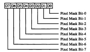
The contents of this register are logically ANDed with the 8 bits of video data coming into the external color palette. Zero bits in this register therefore cause the corresponding address input to the external color palette to be zero. For example, if this register is programmed with 7, only external color palette registers 0-7 would be accessible; video output bits 3-7 would be ignored and all color values would map into the lower 8 locations in the color palette.
