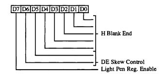
This register is used for all VGA and EGA modes. It is also used for 640 column CGA modes and MDA/Hercules text mode. In all 320 column CGA modes and Hercules graphics mode, the alternate register is used.
