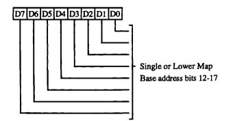
7-0 These eight bits define the Single or Lower Map (in Dual Map Mode) base address bits 17-12. The map starts on a 1K boundary in planar modes and on a 4K boundary in packed pixel modes. In case of dual mapping this register controls the CPU window into the display memory based on the contents of GR06 bits 2-3 as follows:
