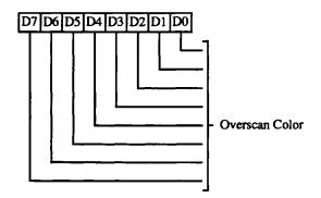
7-0 Overscan Color. These 8 bits define the overscan (border) color value. For monochrome displays, these bits should be zero.
