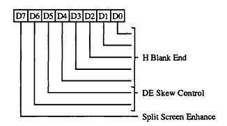
This register is used in low resolution (320-pixel) CGA modes and Hercules graphics modes.
