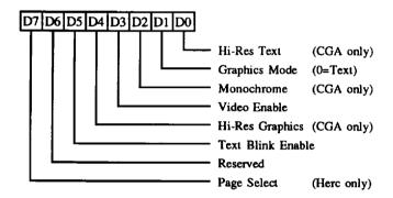
This register is effective only in CGA and Hercules modes. It is accessible if CGA or Hercules emulation mode is selected or the extension registers are enabled. If the extension registers are enabled, the address is determined by the address select in the Miscellaneous Outputs register. Otherwise the address is determined by the emulation mode. It is cleared by RESET.
