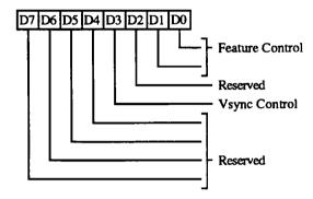
1-0 Feature Control. These bits are used internal to the 82C450 in conjunction with the Configuration Register (XR01). When enabled by XR01 bits 2-3 and Misc Output Register bits 3-2 = 10, these bits determine the pixel clock frequency typically as follows:
