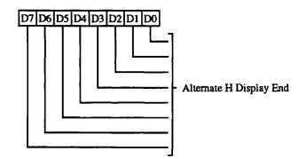
This register is used in low resolution (320-pixel) CGA modes and Hercules graphics modes.
