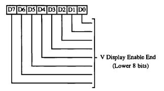
7-0 These are the eight low order bits of a 10-bit register. The 9th and 10th bits are located in the CRT Controller Overflow register. The actual count = Contents of this register + 1.
