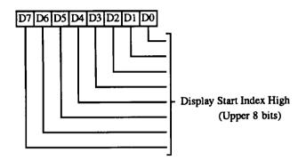
7-0 Upper 8 bits of display start address. In CGA/MDA/Hercules modes, this register wraps around at the 16, 32, and 64 KByte boundaries respectively.
