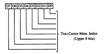
7-0 Upper 8 bits of the memory address where the text cursor is active. In CGA/MDA/Hercules modes, this register wraps around at 16, 32, and 64 KByte boundaries respectively.
