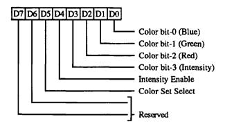
This register is effective only in CGA modes. It is accessible if CGA emulation mode is selected or the extension registers are enabled. This register may also be read or written as an Extension Register (XR7E). It is cleared by RESET.
