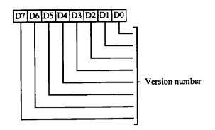
This register contains the version number for the 82C450. Values start at 40h and are incremented for every silicon step. 7-0
