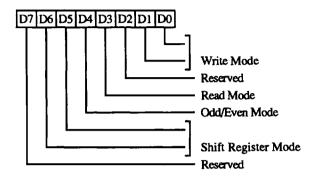
1-0 These bits specify the Write Mode as follows: (For 16-bit writes, the operation is repeated on the lower and upper bytes of CPU data).
