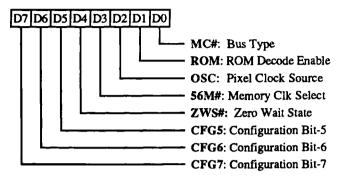
These bits latch the state of the CPU data bus (AD bus) on the falling edge of RESET. The state of bits 0-4 after RESET effect the 82C450 internal logic as indicated below; bits 5-7 are latched from AD5-7 on the falling edge of RESET and may be read in this register, but otherwise have no hardware effect on the 82C450 chip. The AD bus has internal on-chip high-valued pullups and will float high if not driven otherwise during RESET so that the default state of all bits is 'one'.
