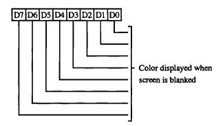
7-0 These bits specify the color to be displayed when the screen is forced to the blank state using SR1 bit-5.
