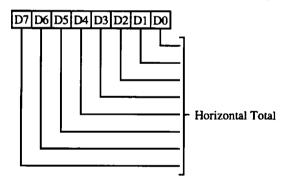
This register is used for all VGA and EGA modes. It is also used for 640 column CGA modes and MDA/Hercules text mode. In all 320 column CGA modes and Hercules graphics mode, the alternate register is used.
