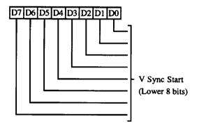
This register is used in all modes. This register is not readable in (Line Compare bit-9) MDA/Hercules emulation or when CR03 bit-7=1.
