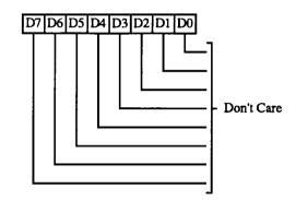
Writing to SR07 with any data will cause the horizontal character counter to be held reset (character counter output = 0) until a write to any other sequencer register with any data value. The write to any index in the range 0-6 clears the latch that is holding the reset condition on the character counter.
