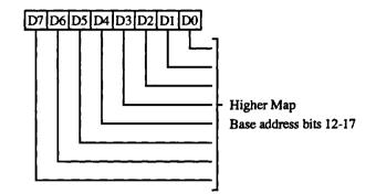
7-0 These eight bits define the Higher Map (in Dual Map Mode) base address bits 17-12. The map starts on a 1K boundary in planar modes and on a 4K boundary in packed pixel modes. This register maps the CPU window into display memory based on the contents of GR06 bits 2-3 as follows:
