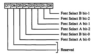
In text modes, bit-3 of the video data's attribute byte normally controls the foreground intensity. This bit may be redefined to control switching between character sets. This latter function is enabled whenever there is a difference in the values of the Character Font Select A and the Character Font Select B bits. If the two values are the same, the character select function is disabled and attribute bit-3 controls the foreground intensity.
