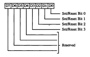
The SET/RESET and ENABLE SET/RESET registers are used to 'expand' 8 bits of CPU data to 32 bits of display memory.
