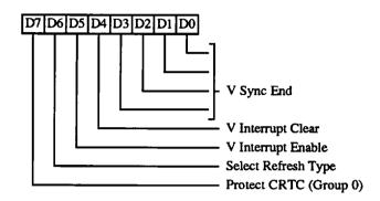
This register is used in all modes. This register is not readable in MDA/Hercules emulation or when CR03 bit-7=1.
