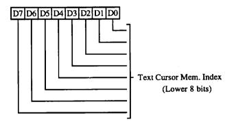
7-0 Lower 8 bits of the memory address where the text cursor is active. In CGA/MDA/Hercules modes, this register wraps around at 16, 32, and 64 KByte boundaries respectively.
