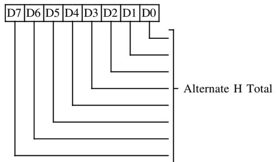
This register is used in CRT low resolution CGA modes, Hercules graphics modes.
