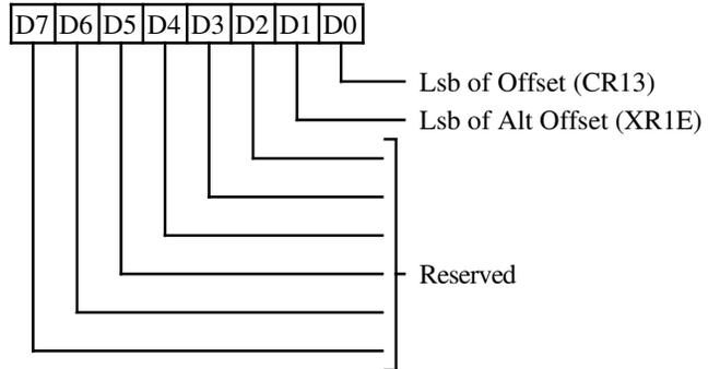
**0** This bit provides finer granularity to the Offset when the word and double word modes are used. This bit is used with the regular Offset register (CR13).
