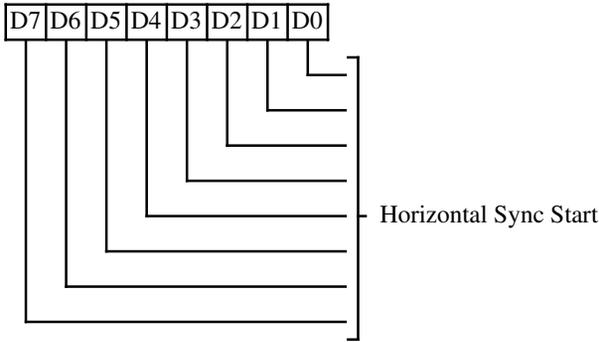
This register is used for all VGA and EGA modes. It is also used for 640 column CGA modes and MDA/Hercules text mode. In all 320 column CGA modes and Hercules graphics mode, the alternate register is used.
