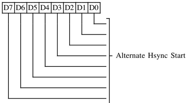
This register is used in CRT low resolution CGA modes, Hercules graphics modes.
