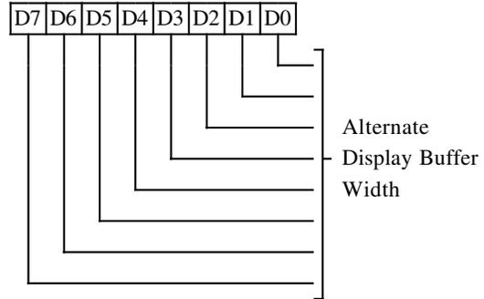
This register is used in low resolution CGA modes and Hercules graphics modes.
