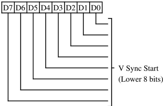
This register is used in all modes. This register is not readable in (Line Compare bit-9) MDA/Hercules emulation or when CR03 D7=1.
