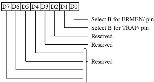
Select bit B determines if the pin should be a general purpose output or perform its normal function.
