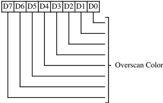
**7-0** Overscan Color. These 8 bits define the overscan (border) color value. For monochrome displays, these bits should be zero.
