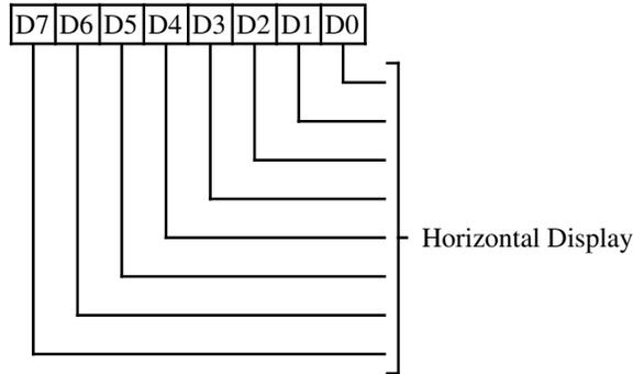
This register is used for all VGA and EGA modes on CRTs. It is also used for 640 column CGA modes and MDA/Hercules text mode. In all 320 column CGA modes and Hercules graphics mode, the alternate register is used.
