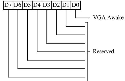
This register is only accessible in Setup Mode. It is cleared by RESET.
