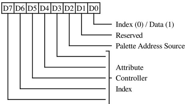
This register may be used to read back the state of the attribute controller index/data latch.
