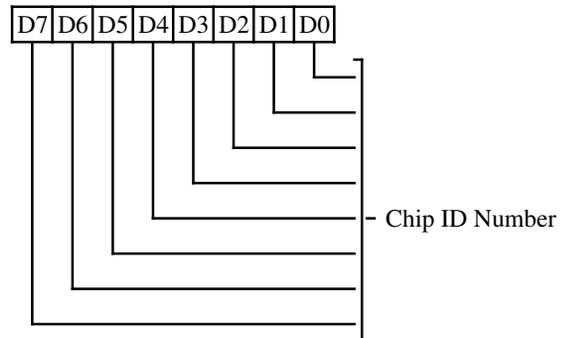
This register is only accessible in Setup Mode.
