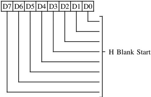
This register is used in CRT low resolution CGA modes and Hercules graphics modes.
