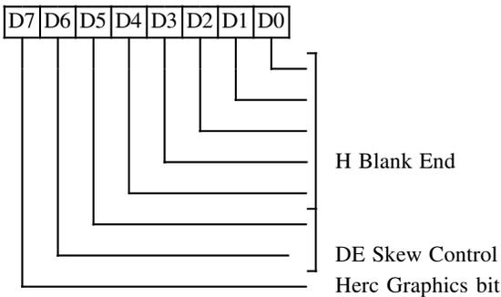
This register is used in CRT low resolution CGA modes and Hercules graphics modes.
