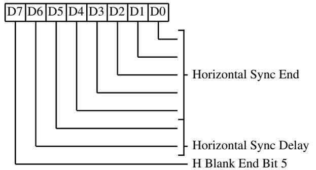
This register is used for all VGA and EGA modes. It is also used for 640 column CGA modes and MDA/Hercules text mode. In all 320 column CGA modes and Hercules graphics mode, the alternate register is used.
