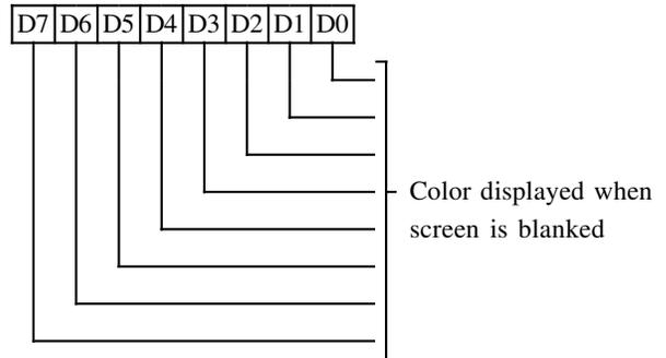
**7-0** Color to be displayed when the screen is forced to blank state (using bit 5 of SR1).
