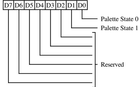
**1-0** Status bits indicate the I/O address of the last CPU write to the external DAC/Color Palette:
