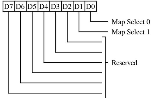
**1-0** This register is also used to 'reduce' 32 bits of memory data to 8 bits for the CPU in the 4-plane graphics mode. These bits select the memory plane from which the CPU reads data in Read Mode 0. In Odd/Even mode, bit-0 is ignored. In Quad mode, bits 0 and 1 are both ignored.
