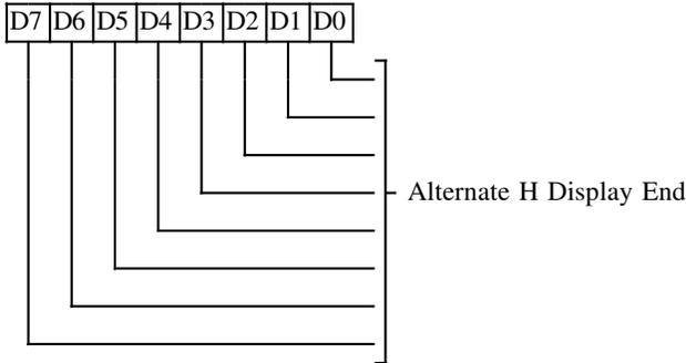
This register is used in CRT low resolution CGA modes, Hercules graphics mode.
