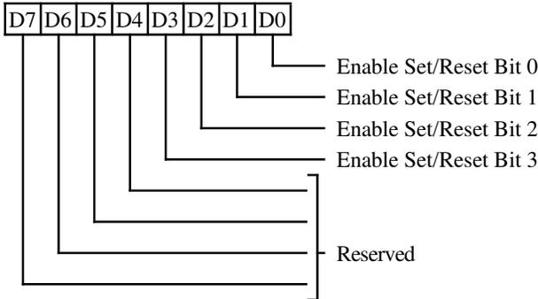
**3-0** This register works in conjunction with the Set/Reset register (GR00). The Graphics Mode register must be programmed to Write Mode 0 in order for this register to have any effect.
