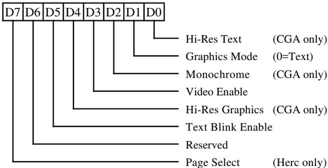
This register is effective only in CGA and Hercules modes. It is accessible if CGA or Hercules emulation mode is selected or the extension registers are enabled. If the extension registers are enabled, the address is determined by the address select in the Miscellaneous Outputs register. Otherwise the address is determined by the emulation mode. It is cleared by RESET.
