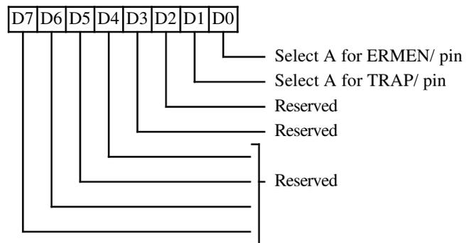
Select bit A determines if the pin should be a general purpose output or perform its normal function.
