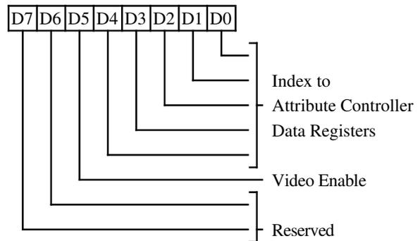
**4-0** These bits point to one of the internal registers of the Attribute Controller
