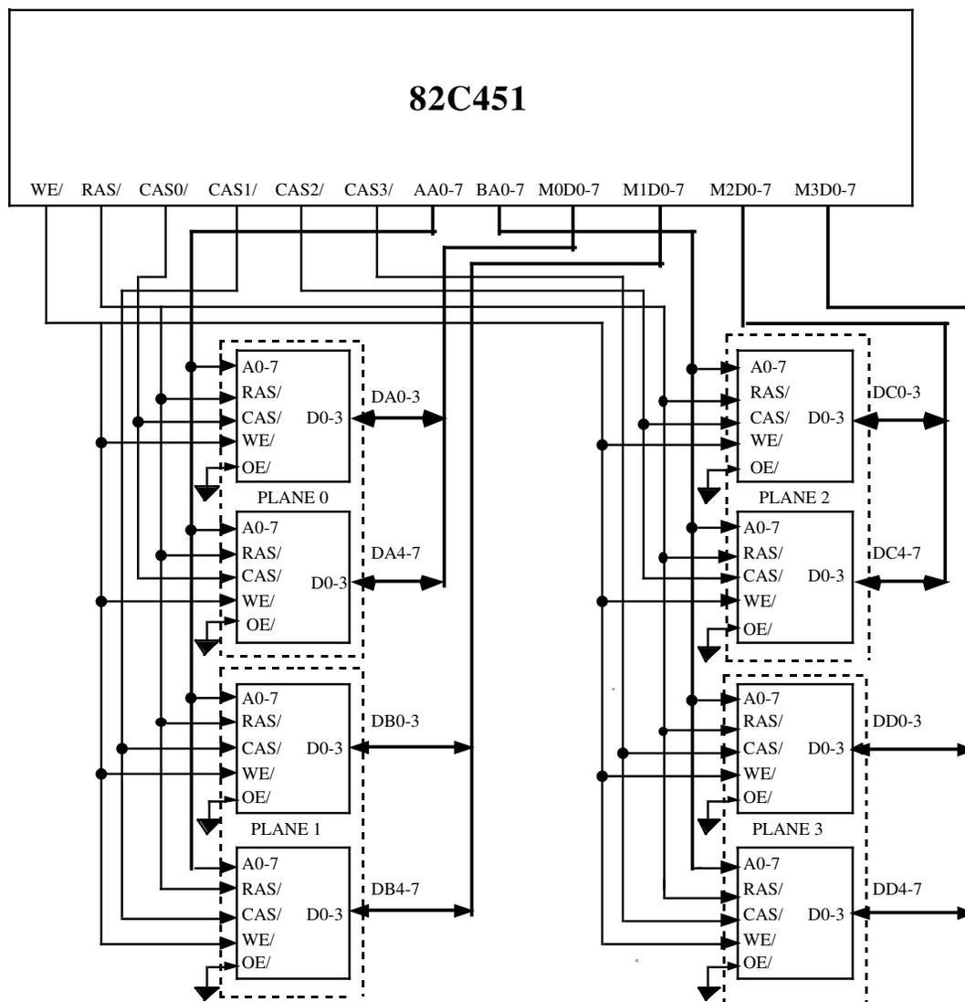
Block Diagram – DRAM Interface for 256 KBytes
