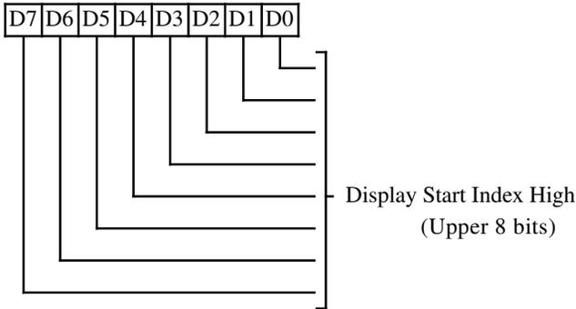
**7-0** Upper 8 bits of display start address. In CGA/MDA/Hercules modes, this register wraps around at the 16, 32, and 64 K byte boundaries respectively.
