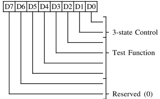
Diagnostic Register (I/O Address 3D7h; Address Pointer: 7Fh). Read - Write Register.
