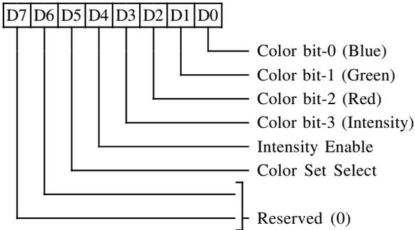
This register is a copy of the CGA color select register 3D9h. Writes to this register will change the copy at 3D9h. It is effective in CGA emulation mode. The copy at 3D9h is visible only in CGA emulation mode. The copy at XR7E is always visible.
