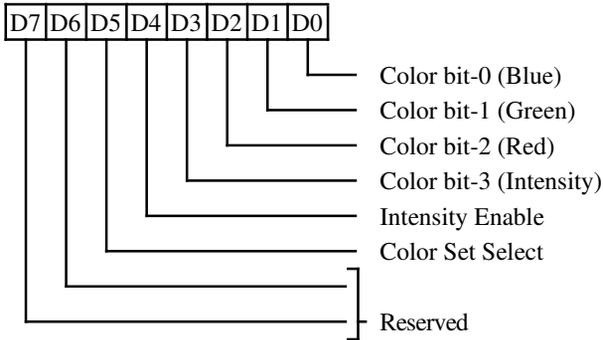
This register is effective only in CGA modes. It is accessible if CGA emulation mode is selected or the extension registers are enabled. This register may also be read or written as an Extension Register (XR7E). It is cleared by RESET. In Hercules Graphics mode, this register should be accessed at 7Eh. A value of 0Fh in 7Eh will work for the Hercules Graphics mode.
