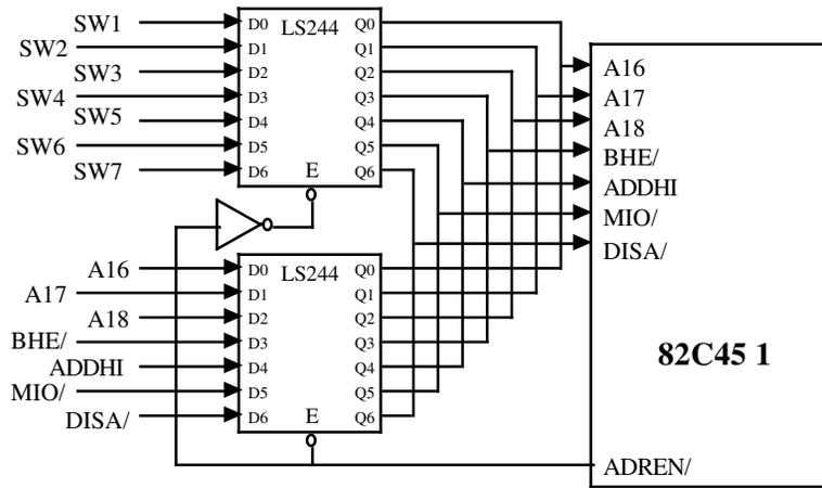
Block Diagram – DIP Switch Interface (MCA Bus)
