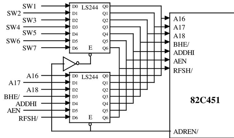
Block Diagram – DIP Switch Interface (EISA/ISA Bus)
