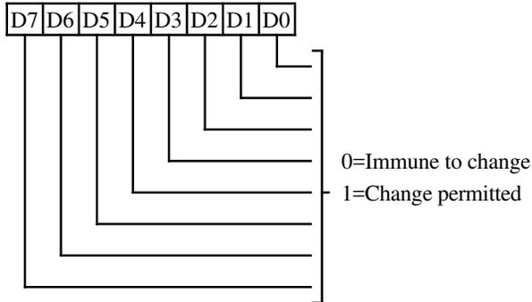
**7-0** This bit mask is applicable to any data written by the CPU, including that subject to a rotate, logical function (AND, OR, XOR), Set/Reset, and No Change. In order to execute a proper read-modify-write cycle into displayed memory, each byte must first be read (and latched by the VGA), the Bit Mask register set, and the new data then written. The bit mask applies to all four planes simultaneously.
