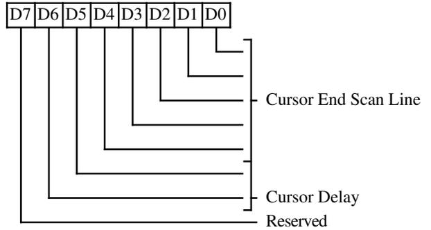
**4-0** These bits specify the scan line of a character row where the cursor display ends: Last scan line for the block cursor = Value + 1.
