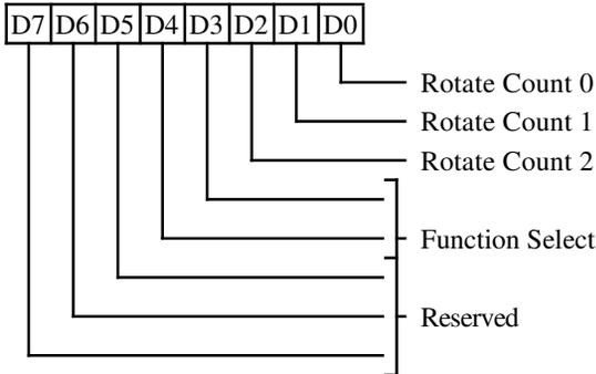
**2-0** These bits specify the number of bits to rotate to the right the data being written by the CPU. The CPU data bits are first rotated, then subjected to the logical operation as specified in the Function Select bit field. The rotate function is active only if the Graphics Mode register is programmed for Write Mode 0.
