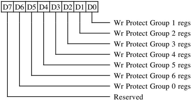
This register controls write protection for various groups of registers as shown. 0 = unprotected, 1 = protected.
