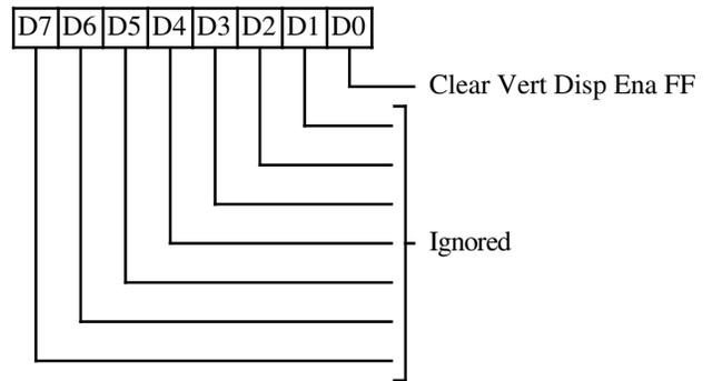
Writing odd data values to CRTC index 30-3Fh causes the vertical display enable flip-flop to be cleared. The flip-flop is automatically set by reaching vertical total. The effect of this is to force a longer vertical retrace period. There are two side effects of terminating vertical display enable early: first, the screen blanks early for one frame causing a minor visual disturbance and second, the sequencer gives more display memory cycles to the CPU because vertical display is not enabled.
