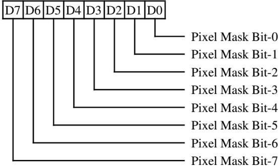
The contents of this register are logically ANDed with the 8 bits of video data coming into the external color palette. Zero bits in this register therefore cause the corresponding address input to the external color palette to be zero. For example, if this register is programmed with 7, only external color palette registers 0-7 would be accessible; video output bits 3-7 would be ignored and all color values would map into the lower 8 locations in the color palette.
