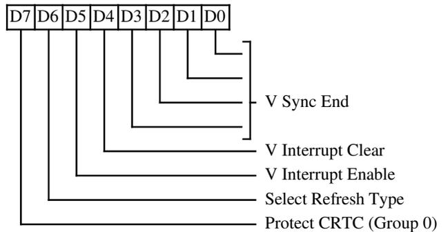
This register is used in all modes. This register is not readable in MDA/Hercules emulation or when CR03 D7=1.
