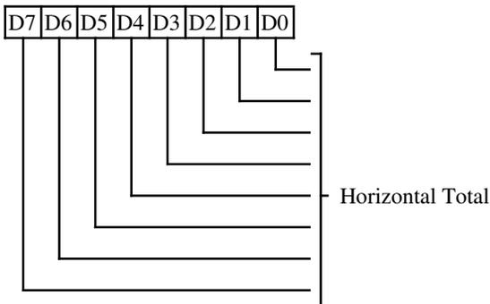
This register is used for all VGA and EGA modes. It is also used for 640 column CGA modes and MDA/Hercules text mode. In all 320 column CGA modes and Hercules graphics mode, the alternate register is used.
