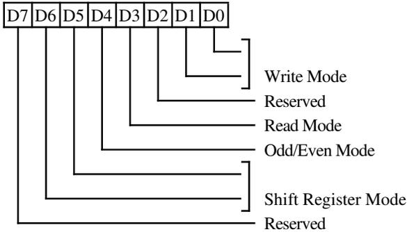
**1-0** These bits specify the Write Mode as follows: (For 16-bit writes, the operation is repeated on the lower and upper bytes of CPU data).
