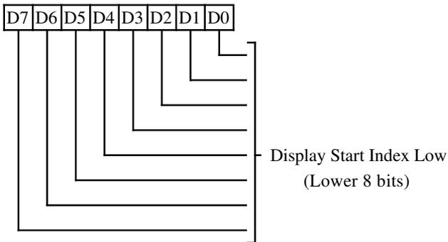
**7-0** Lower 8 bits of the display start address. The display start address points to the memory address corresponding to the top left corner of the screen.
