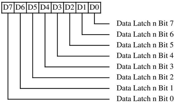
This register may be used to read the state of Graphics Controller Memory Data Latch 'n', where 'n' is controlled by the Graphics Controller Read Map Select Register (GR04 D0 & D1) and is in the range 0-3.
