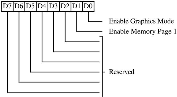
This register is effective only in Hercules mode. It is accessible in Hercules emulation mode or if the extension registers are enabled. It may be read back through XR14 D3 & D2. It is cleared by RESET.
