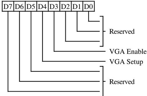
This register is used with the PC-Bus Interface only. It is cleared by RESET. In the MCA interface, the Setup mode and VGA Disable are controlled through the SETUP/ and DISA/ pins, respectively.
