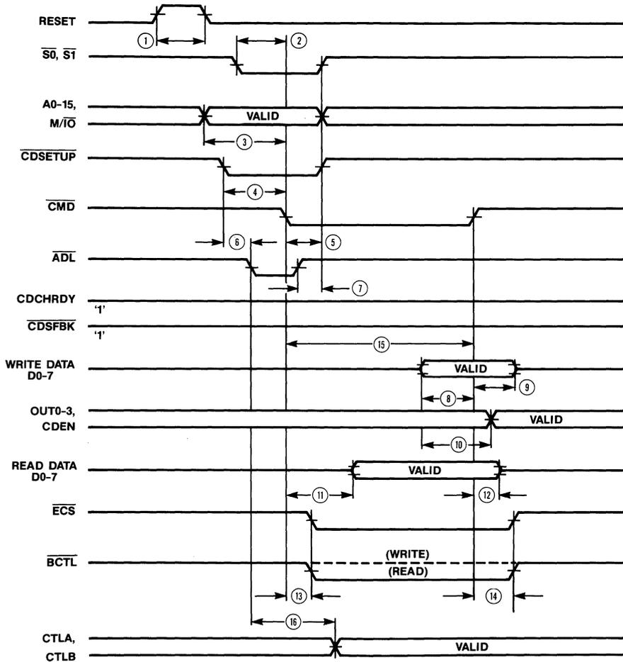
POS Register Setup Cycle Timing
