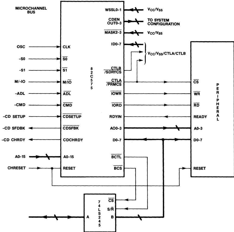
**Figure 2. 82C575 Application Diagram for 8-Bit I/O Slave Peripheral**
