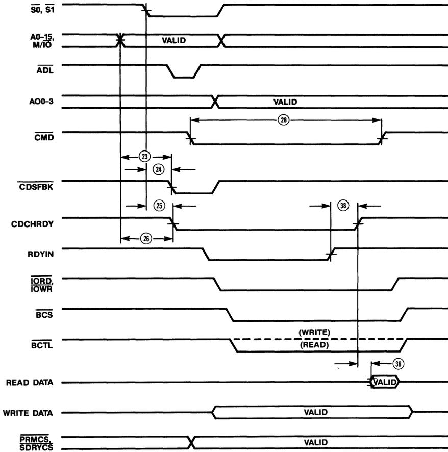
External Asynchronous Extended Cycle Timing
