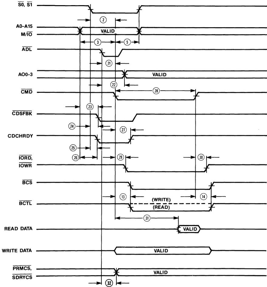
**Synchronous Extended Cycle Timing**
