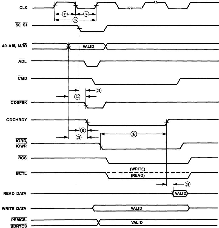
Synchronous Wait State 1 & Wait State 2 Cycle Timing
