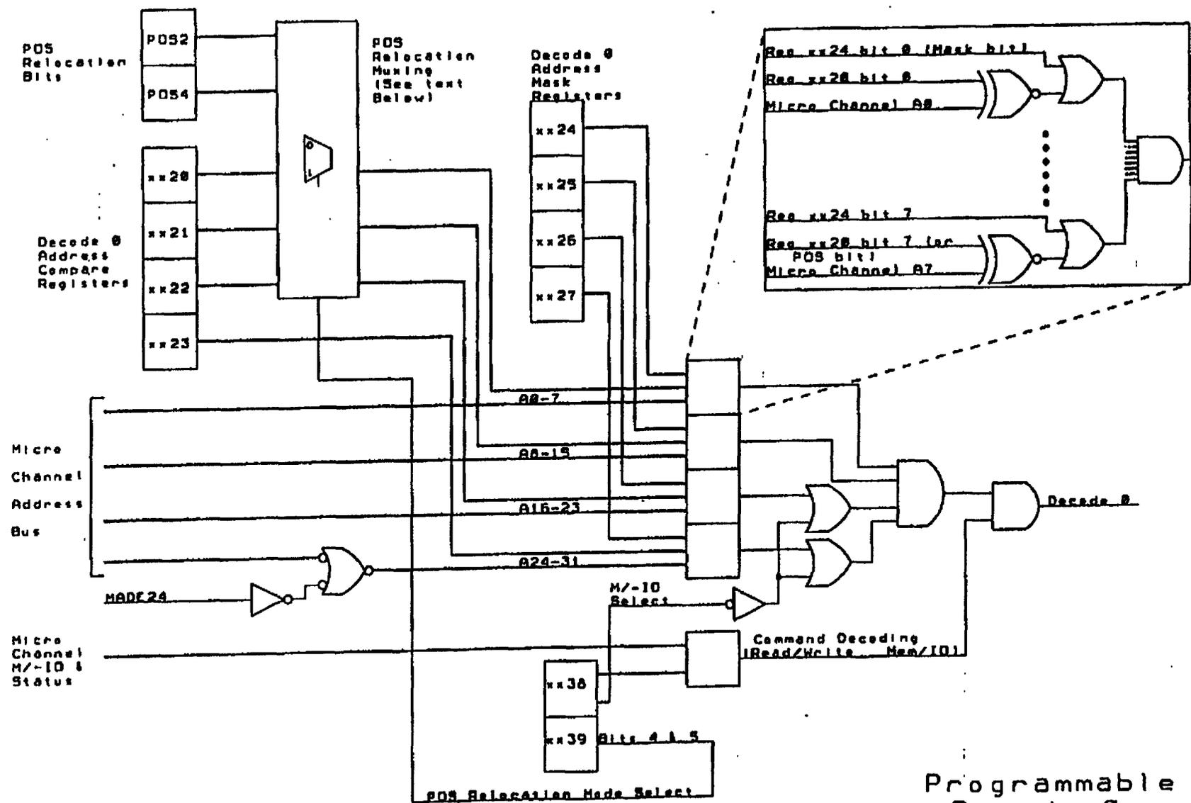
The POS Relocation Muxes replace some of the programmed compare register bits with POS bits. Which bits are replaced is dependent on the POS relocation mode in use. The MASK bits are still in effect for bits controlled by POS relocation.
