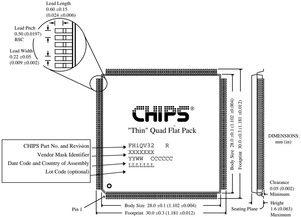
**Figure 18-1: Thin Quad Flat Pack (TQFP)**
