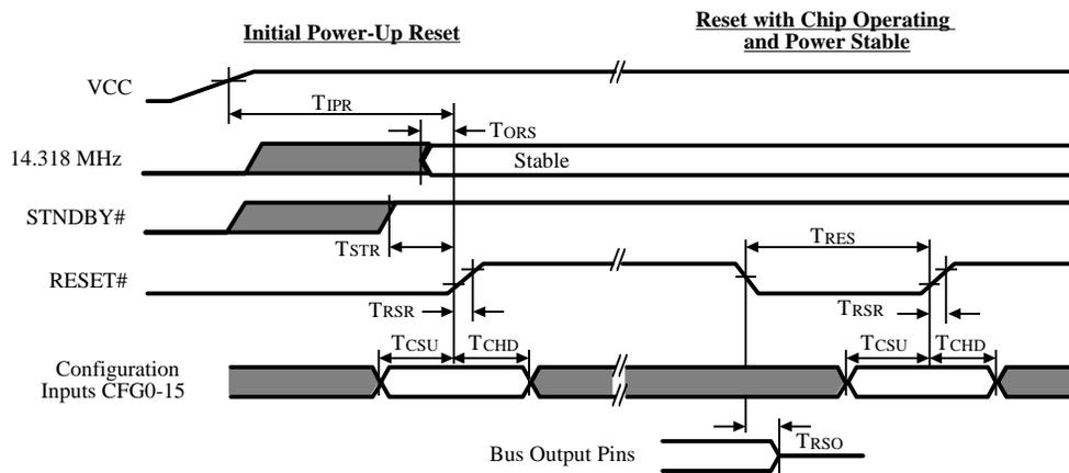
Figure 17-4: Reset Timing
