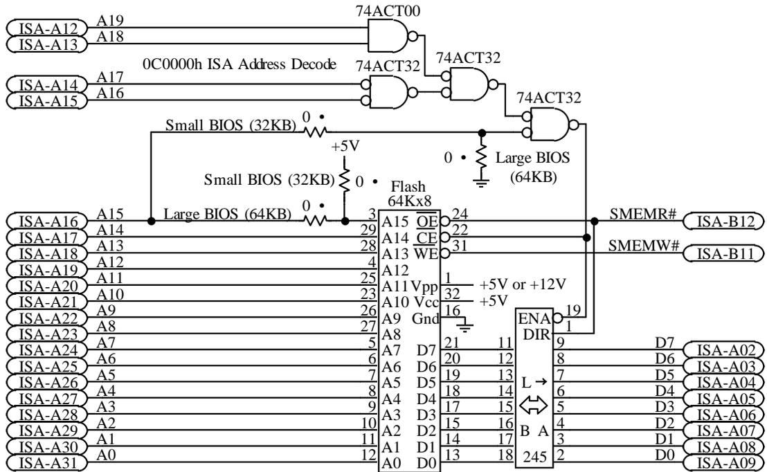
Figure 16-3: Circuit Example - VL-Bus BIOS Interface
