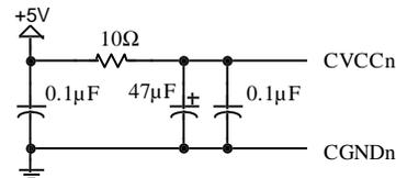
The suggested method for layout assumes a multi-layer board including VCC and GND planes. All ground connections should be made as close to the pin / component as possible. The CVCC trace should route from the 65550 **through the pads** of the filter components. The trace should NOT be connected to the filter components by a stub. All components (particularly the nearest 0.1μF capacitor) should be placed as close as possible to the 65550.
