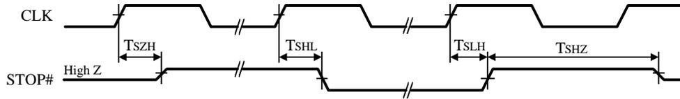
**Figure 17-6: PCI Bus Stop Timing**
