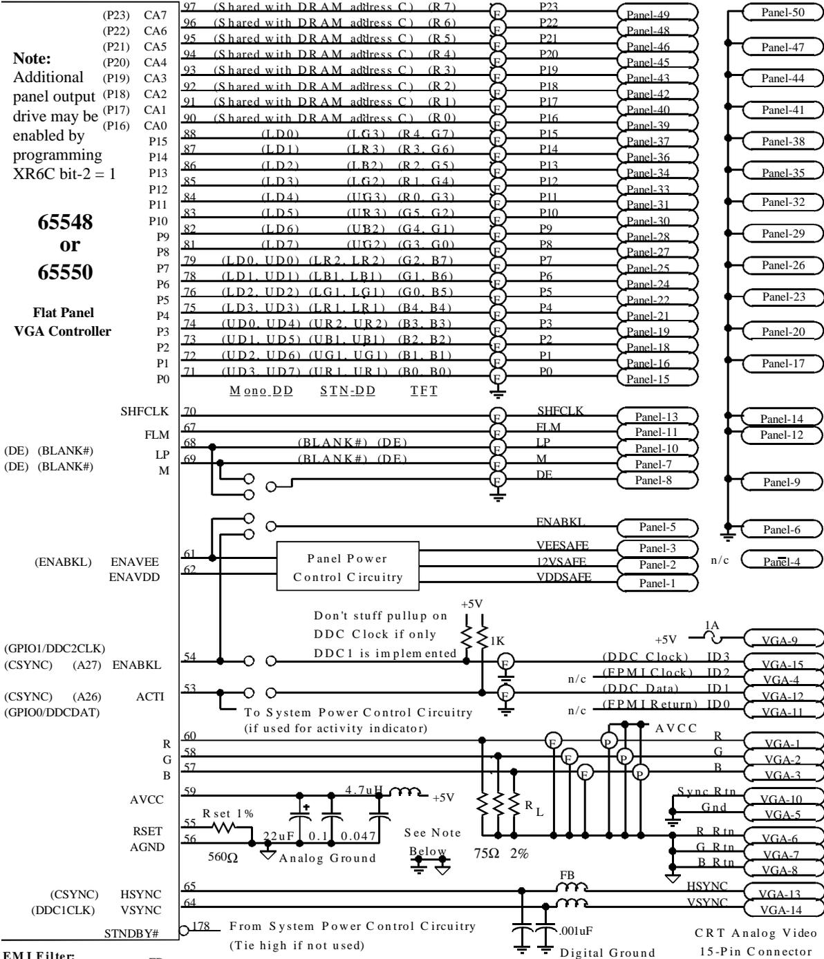
R<sub>SET</sub> is driven by a fixed reference voltage of 1.214V. The full-scale current on each R, G, or B output is proportional to R<sub>SET</sub> current. Use 560Ω to get 17.6mA full-scale on R, G, & B (each), plus 1.43mA optional "pedestal" current if enabled.
