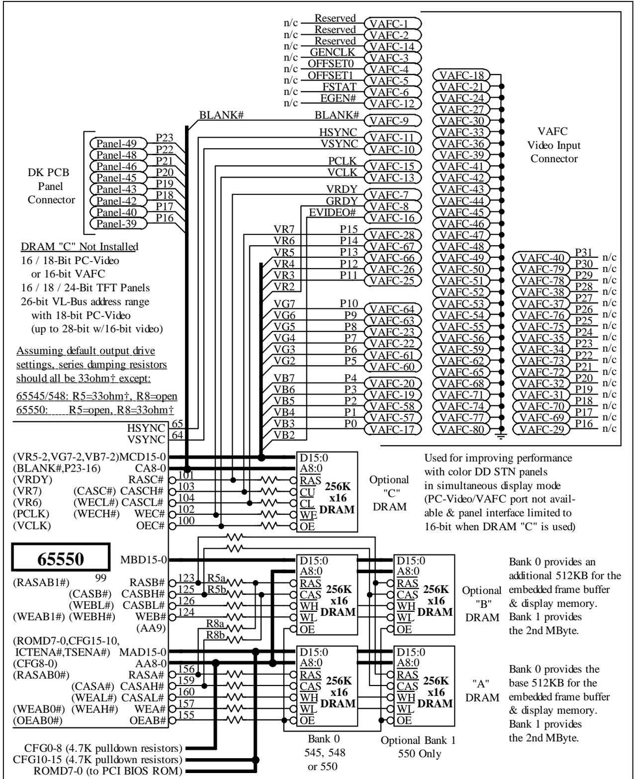
†Typical resistor value. Actual value for a specific PCB layout should be determined by experimentation for optimal signal damping
