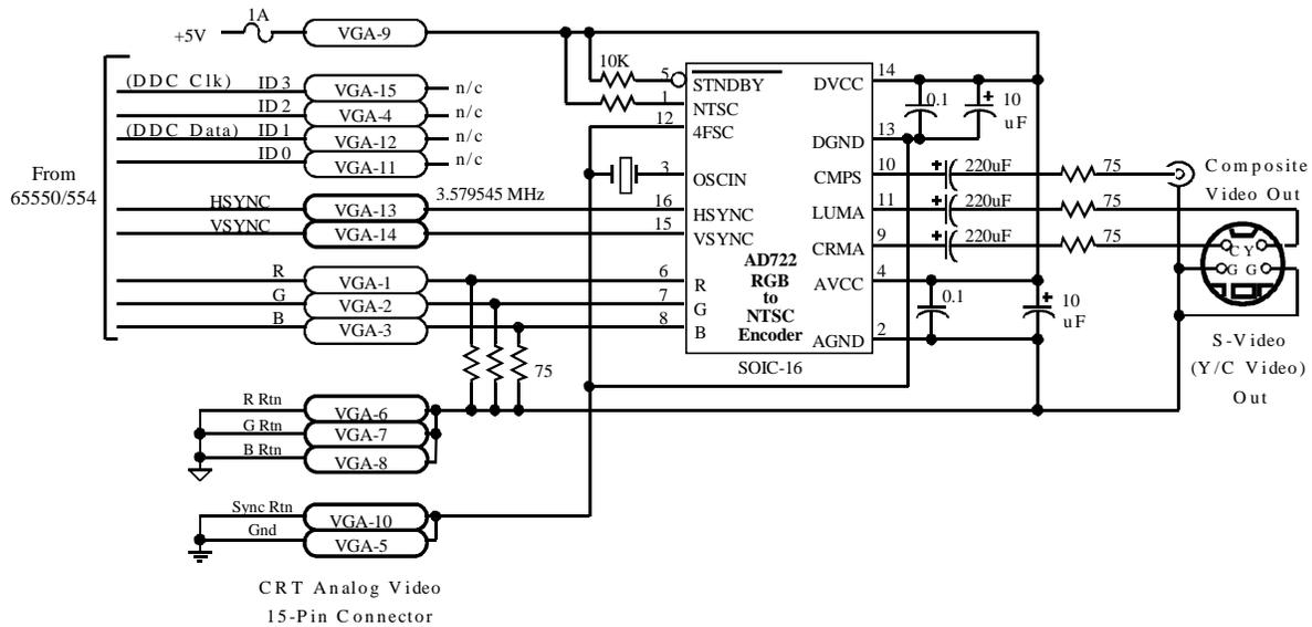
**Figure 16-10: Circuit Example RGB-to-NTSC Encoder**
