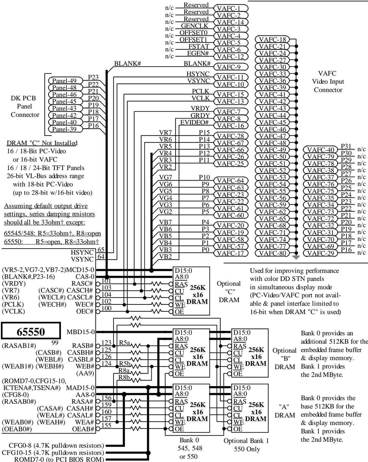
†Typical resistor value. Actual value for a specific PCB layout should be determined by experimentation for optimal signal damping
