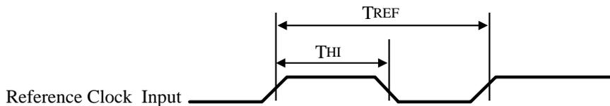
Figure 17-2: Reference Clock Timing
