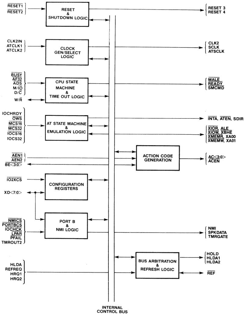
**Figure 1-1. 82C301 Functional Block Diagram**
