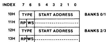
**Figure 2.6. DRAM Configuration/Timing Register Summary**
