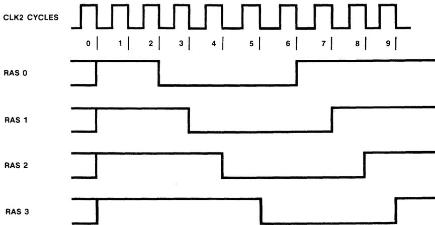
**Figure 2-3. Staggered RAS pulses during refresh**
