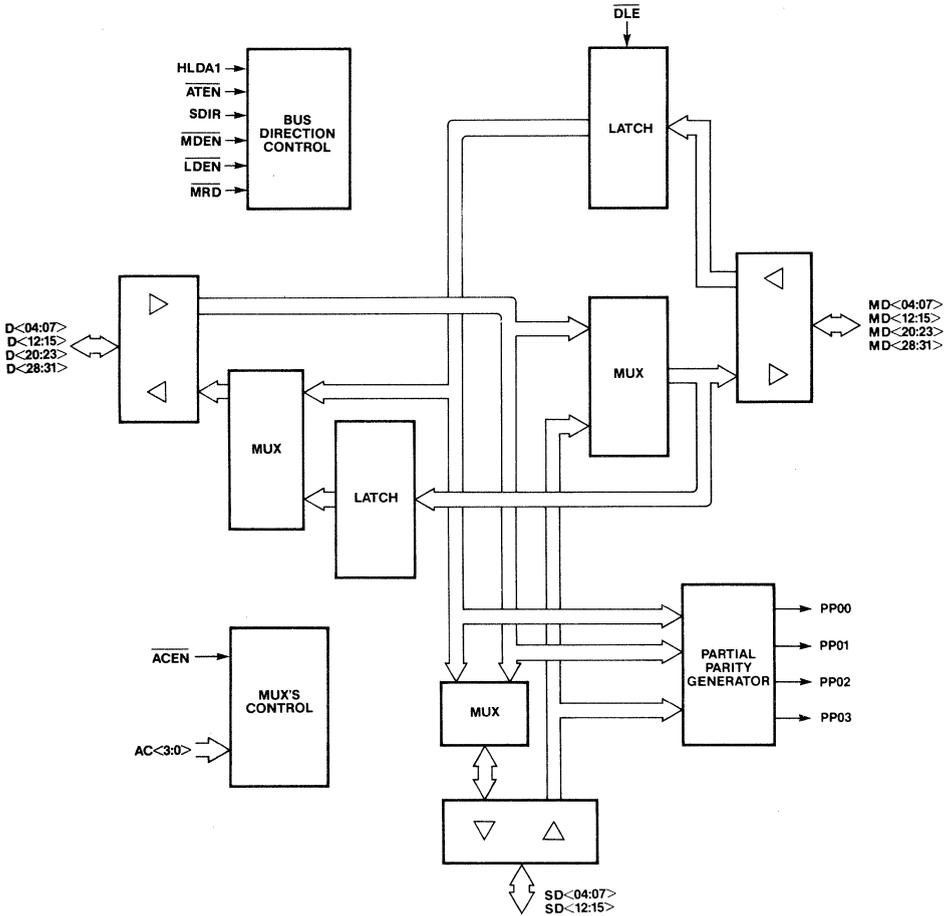
**Figure 5-1. 82A305 Functional Block Diagram**
