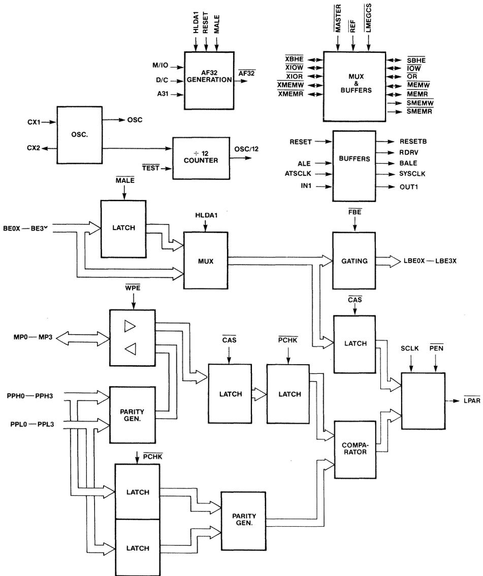
Figure 6-1. 82A306 Functional Block Diagram
