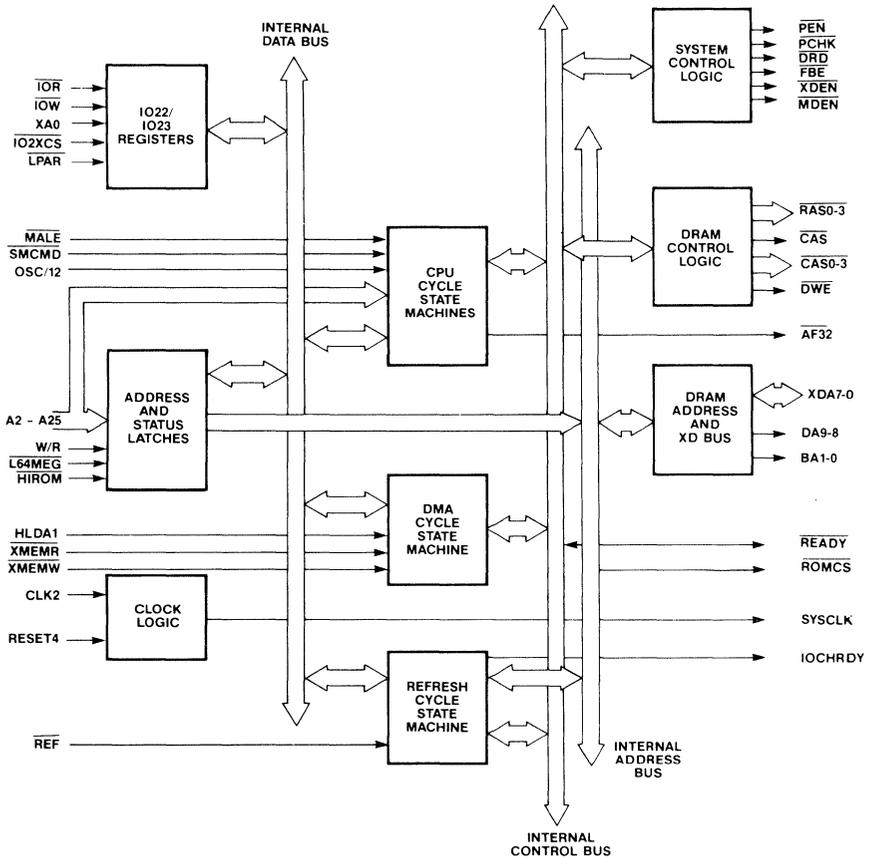
**Figure 2-1. 82C302 Functional Block Diagram**
