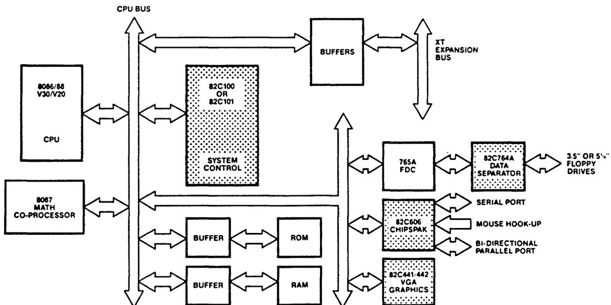
**Figure 1. Super XT Model 30 Compatible System**
