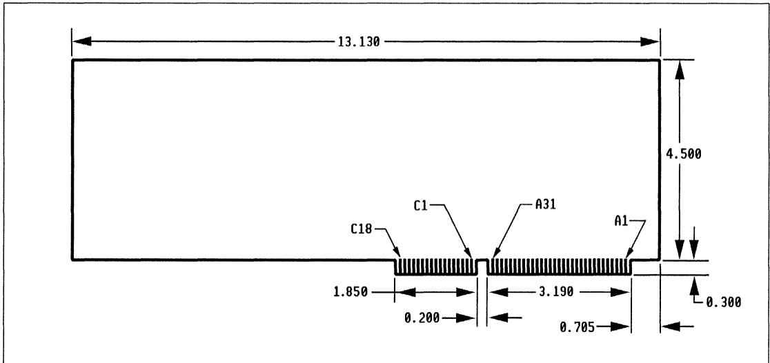
Figure 3-7 shows the maximum length of an AT board in I/O slots 1 and 2.
