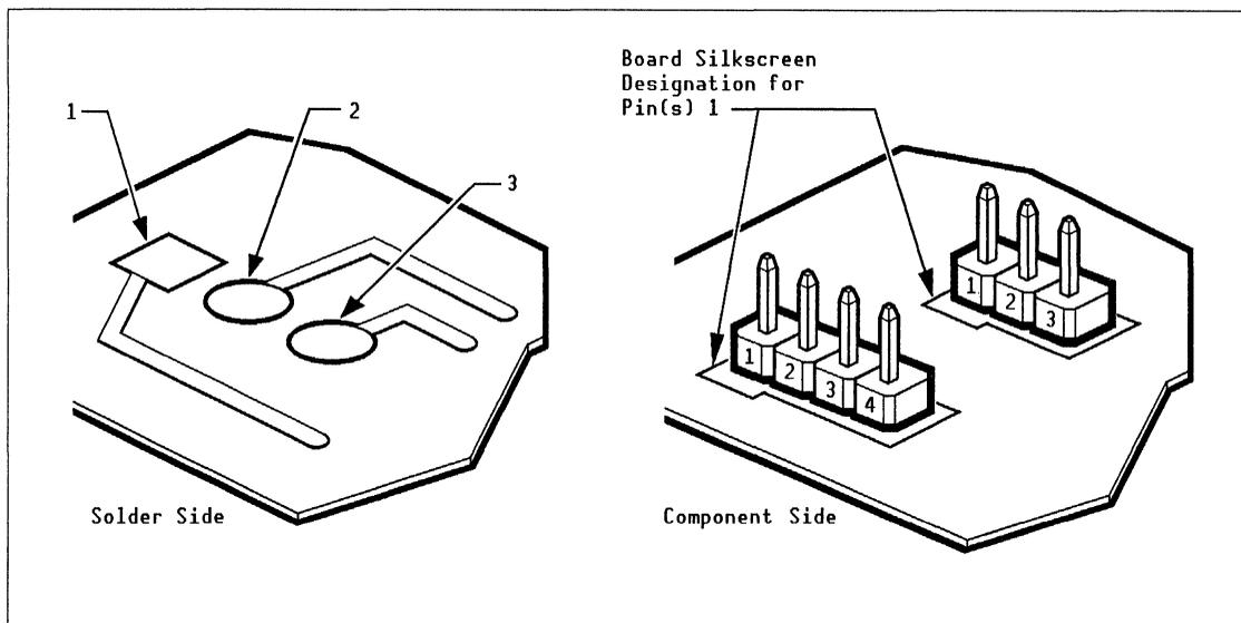
The MK82310-PI-Super system board also contains Berg connectors that are “keyed.” A missing pin is the key or polarity indicator. It is used as a guide to install the system cables correctly. Figure 2-4 shows a 5-pin Berg connector with key.
