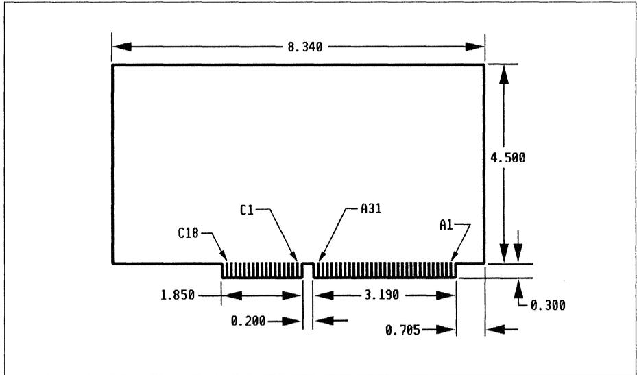
AT slot 5 on the MK82310-PI-Super board accommodates XT adapter boards with PCB depths below the 8-bit I/O connector. XT cards can have depths up to 0.5 inch below the 8-bit I/O connector. Note that AT slot 5 can be optionally populated with an 8-bit or 16-bit I/O connector. The MK82310-PI-Super is shipped with AT slot 5 configured as an 8-bit slot. Figure 3-8 shows the XT deep slot adapter board dimensions.
