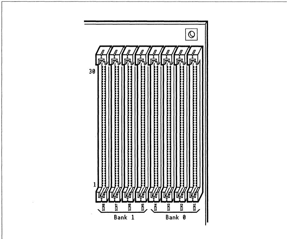
SIMMs 1-4 are configured as bank 0. SIMMs 5-8 are configured as bank 1. The same type of memory must be placed in each bank if interleaving of banks is to be used. When only one bank is populated, bank 0 should be used. The MK82310-PI-Super board can be configured for different amounts of memory. Table 3-10 shows the possible memory configurations.
