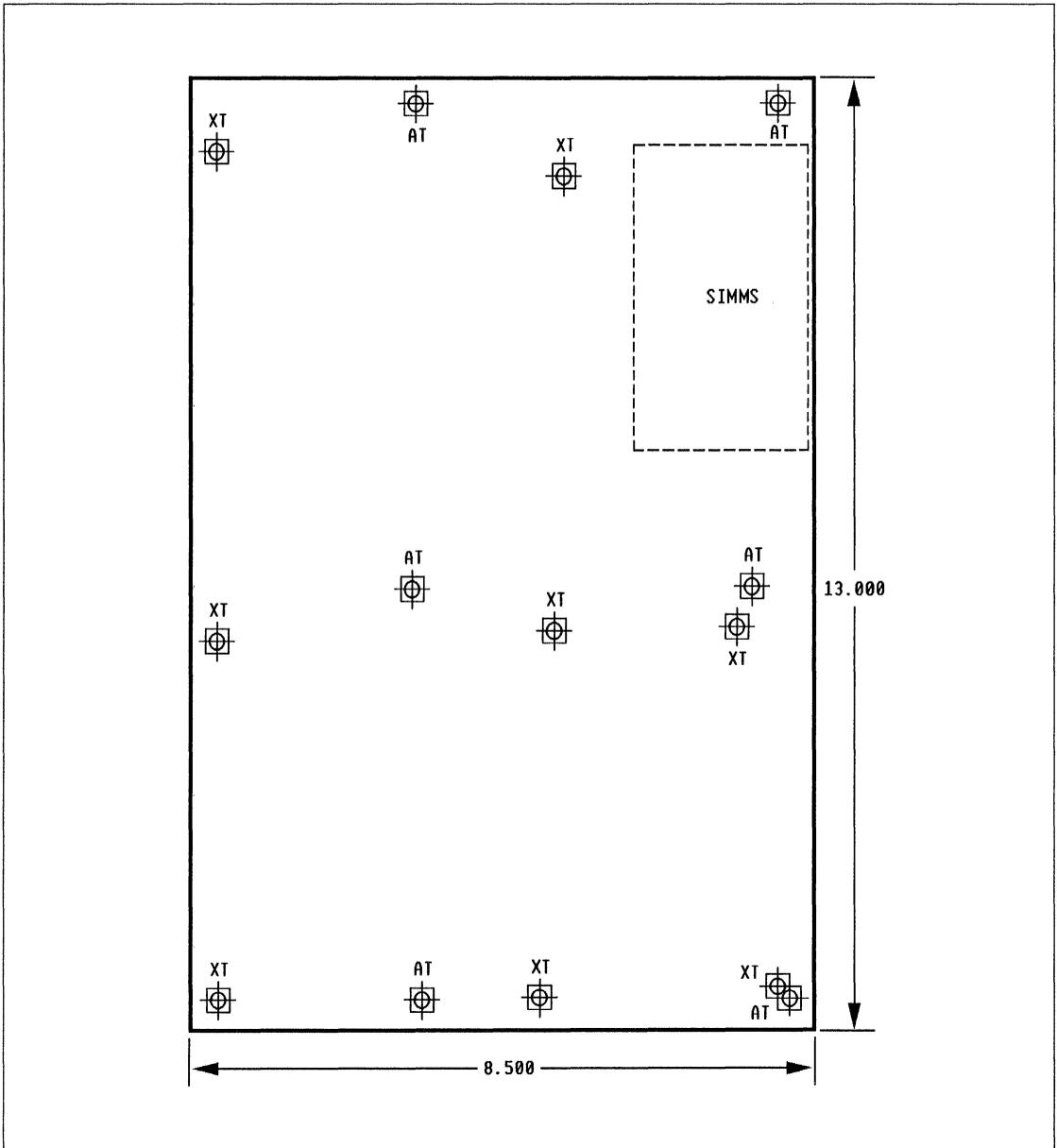
Figure 3-5. Adapter I/O Slot Locations
