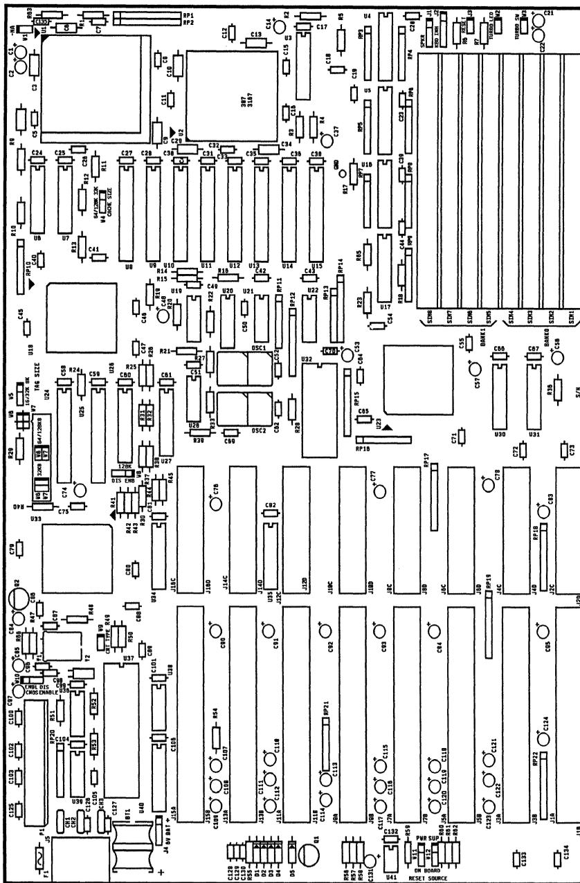
**Figure 2-2.** *Location of MK82310-PI-Super Connectors and Jumpers*
